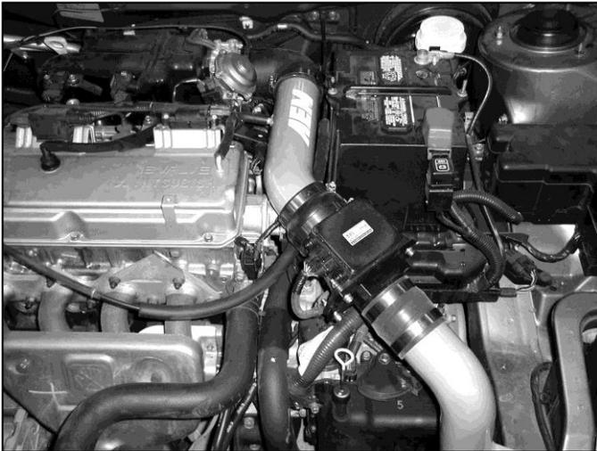
h. Plug the wiring harness into the MAF sensor and attach the lower intake pipe to MAF sensor using the provided silicone hose and two hose clamps.
