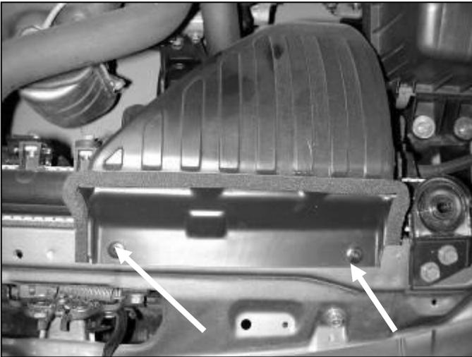
e. Release the air snorkel. Press in the centers of the plastic rivets and remove.
