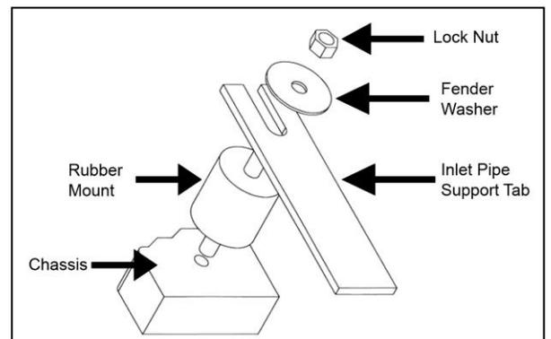
j. Proper installation of the rubber mount.
