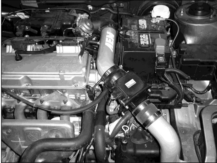
k. Install the AEM<sup>®</sup> air filter onto the lower end of the intake pipe. Check the clearance of the air filter and tighten the hose clamp once proper fitment is achieved.
