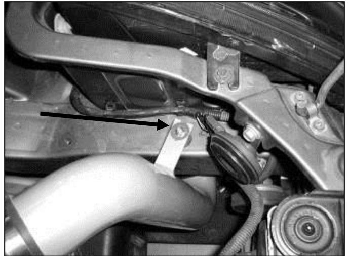
i. Install rubber mount into frame and attach the lower intake pipe's support bracket as shown. Secure with a lock nut and fender washer but do not completely tighten the lock nut. See the diagram below for proper installation of the rubber mount.
