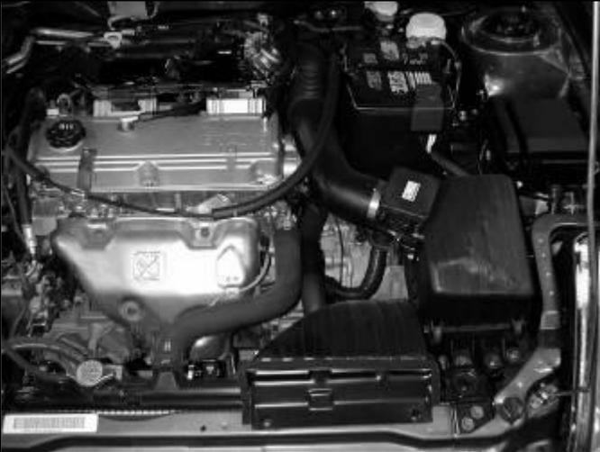
a. Stock air box system installed.
