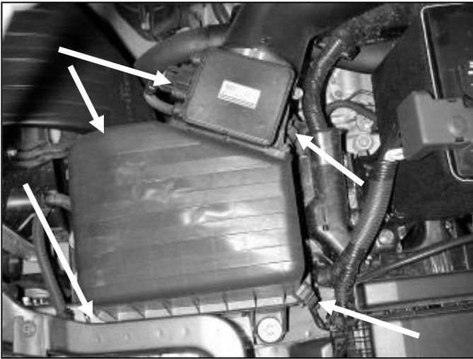
c. Unplug the MAF sensor. Remove the stock inlet pipe. Release four clamps on the air box and remove the upper air box from the vehicle.
