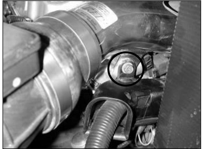
g. Attach the bracket on the upper pipe to the engine using the supplied 6mm bolt and washer. Place the pipe's tab behind the stock plastic tab. Attach the MAF sensor assembly to the intake pipe as shown.
