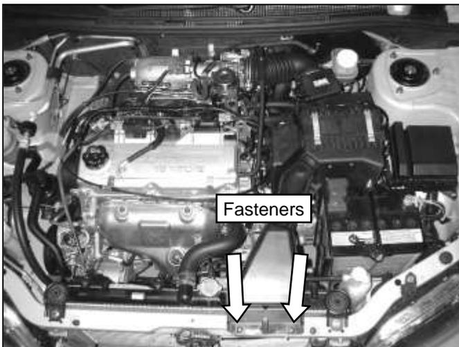
a. Remove the fasteners holding the air duct to the radiator support, and remove it.
