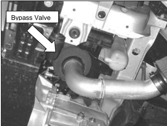
If AEM<sup>®</sup> Bypass Valve (part # 20-402S) is installed, install the bypass valve as shown in the figure above. The intake pipe will require modification so follow the instructions included with the AEM Bypass Valve accordingly.
