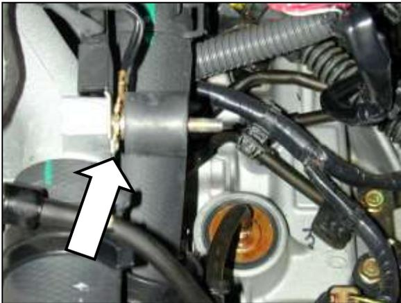
b. Install the supplied rubber mount where the bolt was removed in step 2o using the 1/4" flat washer as shown.
