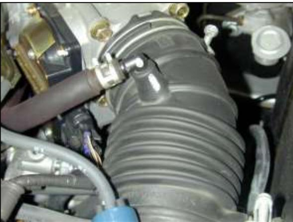
c. Remove the breather hose from inlet air hose by compressing the spring clamp and pulling it off.
