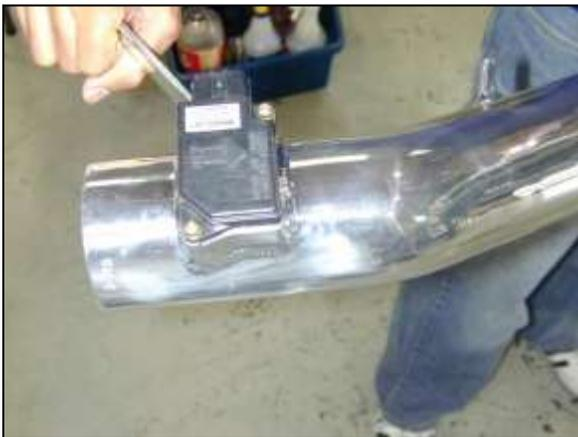
d. Install the previously removed MAF sensor into the upper intake pipe using the two bolts removed in step 2p.
