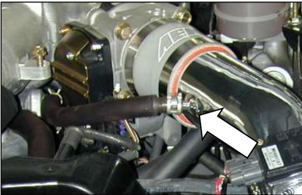
h. Attach the stock breather hose using the original spring clamp.
