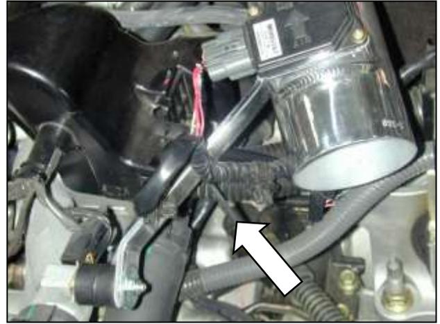
g. Plug in the MAF sensor wiring harness. Secure the plug and extra wire for the bypass solenoid using a 6" zip tie.
