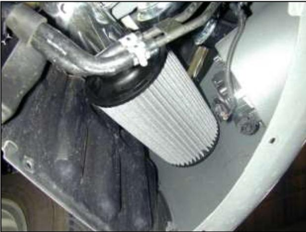
n. Install the AEM® air filter onto the end of the intake pipe. Push the air filter over the intake pipe until the stop in the air filter is reached. Then install one hose clamp to secure the filter onto the intake pipe.
