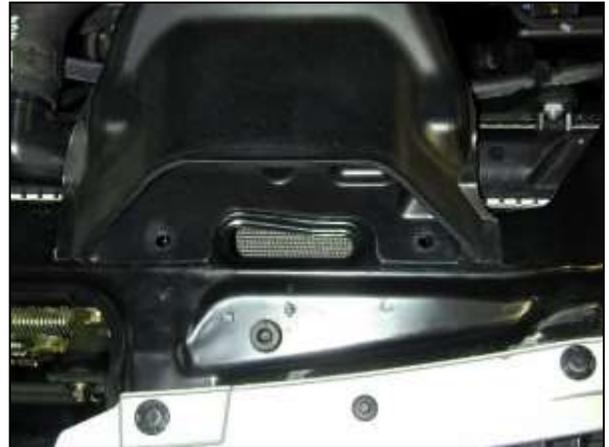
b. Remove the two plastic rivets holding the intake duct to the radiator support.
