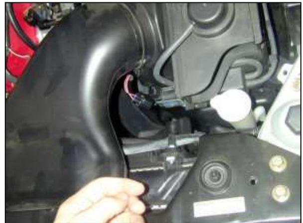
h. Unplug the bypass solenoid harness and vacuum hose. Unclip the harness from the air filter housing. Unplug the vacuum hose from the intake manifold and remove the bolt securing the line.
