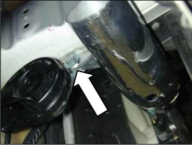
l. Align the fixed lower intake pipe bracket with the hole where the horn was previously removed. Install the supplied M8 bolt, washer, and horn.
