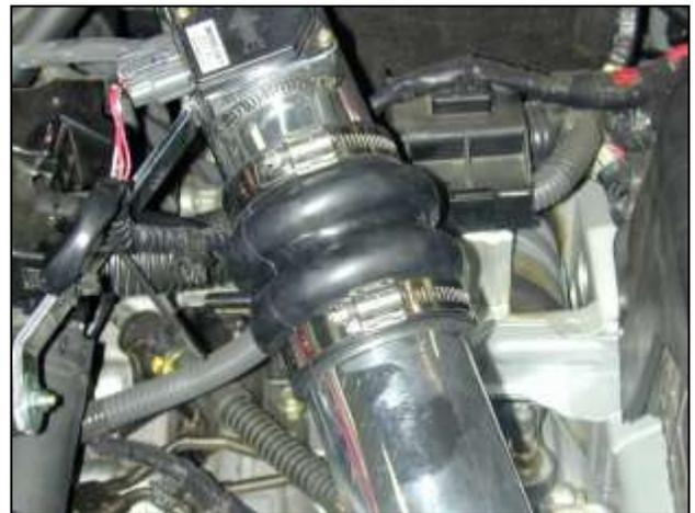
k. Slide the lower intake pipe in from the bottom and align the upper and lower pipes. Slide the hump hose over the end of the upper intake pipe and secure using a #44 hose clamp.
