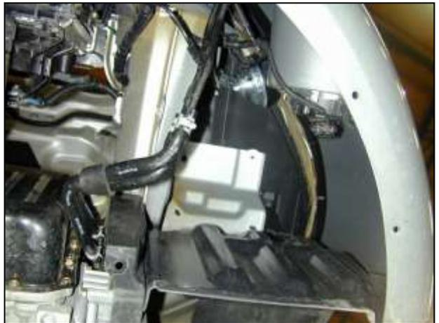
n. Remove the bolt securing the horn to the chassis and remove the horn. Remove the remaining two bolts securing the lower resonator to the chassis and remove the resonator.
