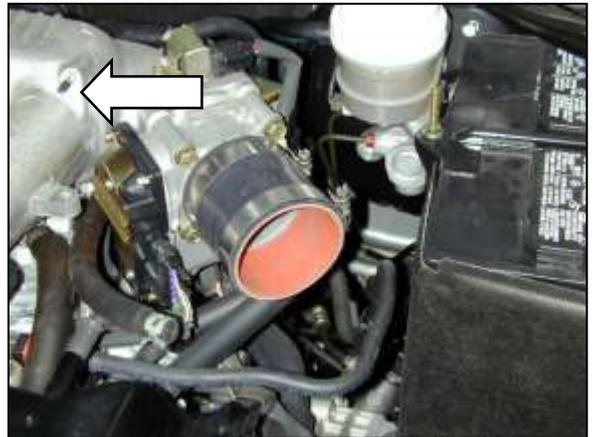
c. Install the 2.75" silicone coupler onto the throttle body and secure using a #44 hose clamp. Also, install the vacuum cap on the intake manifold nipple as indicated above.
