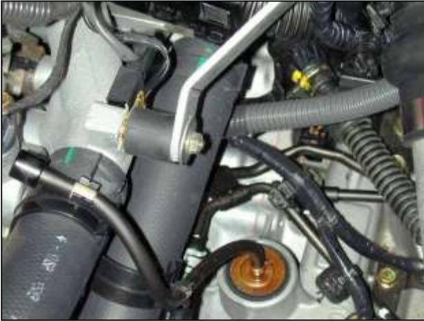
f. Align the intake mounting bracket with the previously installed rubber mount and secure using a 6mm flat washer and serrated nut.
