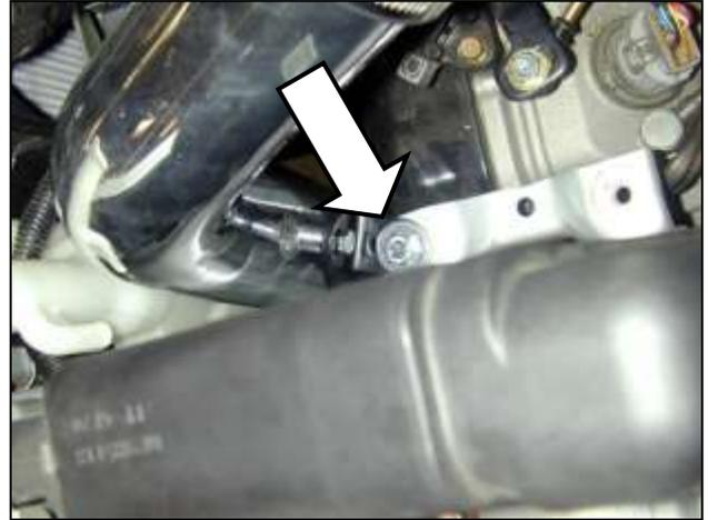
m. Install the M6 bolt into the bracket installed in step 3h. Thread the bolt into the threaded bung on the lower intake pipe. Tighten the bolts loosened in step 2i.
