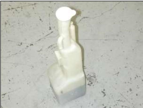
m. Unplug the radiator fan harness. Unhook the radiator overflow hose from the reservoir and remove the reservoir.
