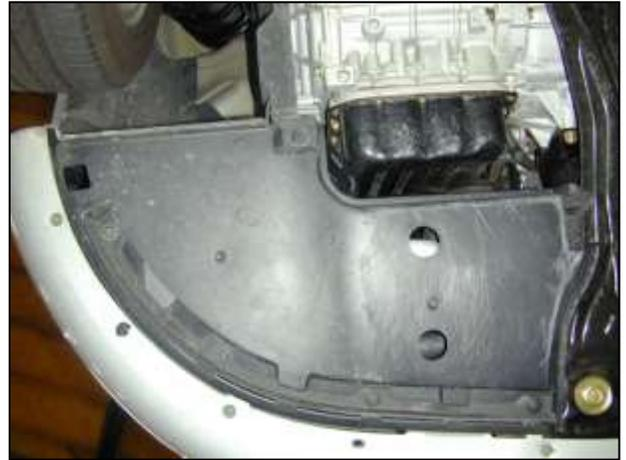
l. Remove the five screws and four plastic connectors securing the driver's side underbody splash shield to the chassis.
