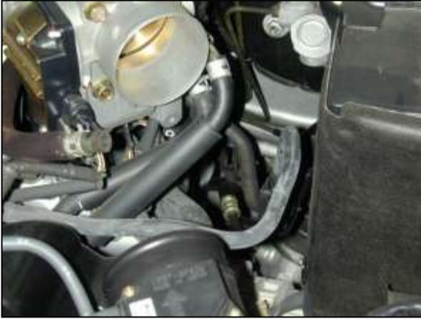
e. Loosen the hose clamp on the air filter housing and remove the air inlet tube and upper resonator.
