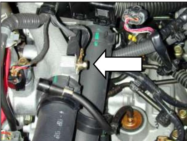
o. Remove the ground bolt on the aluminum coolant line as shown.
