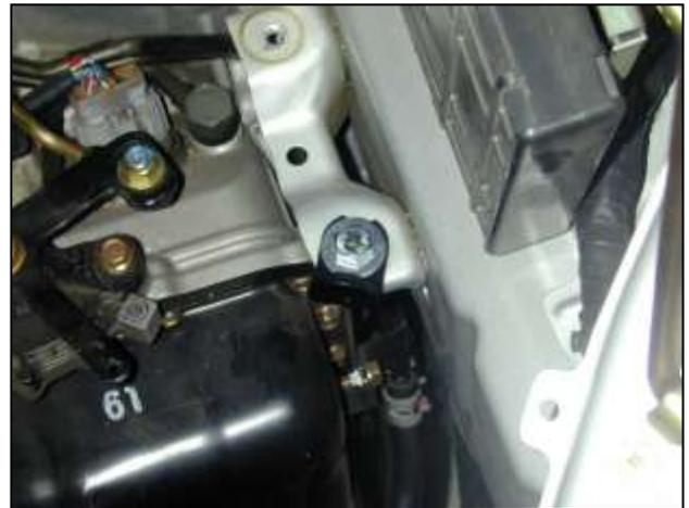
i. Install the lower pipe bolt on mounting bracket using the supplied M8 bolt and washer as shown. Leave this bracket fairly loose.
