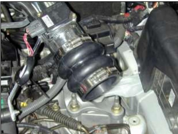
j. Install the supplied hump hose on to the end of the lower intake pipe. Secure using a #44 hose clamp.
