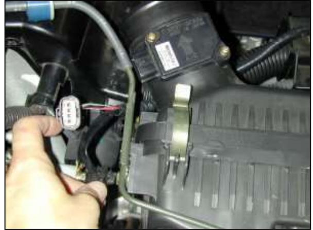
f. Unclip the Mass Air Flow (MAF) sensor wiring harness from the air filter housing. These clips can be removed undamaged from the harness using a small flat head screwdriver. Unplug the MAF sensor from the engine harness.
