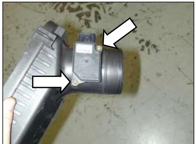
p. Remove the two bolts securing the MAF sensor to the air filter housing and remove the MAF sensor. Be careful not to damage the sensor.
