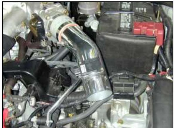
e. Check that the inside of the AEM® intake pipe is free from debris. Install the intake pipe into the previously installed coupler as shown.
