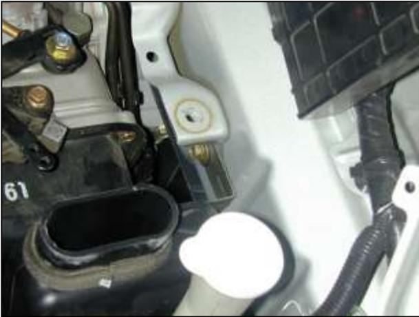
k. Locate the bolt securing the lower resonator in the engine compartment and remove it.
