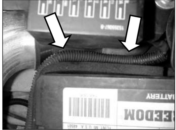
o. Reinstall the battery. Confirm that the positive lead from the fuse box is on top of the intake pipe and is not pinched between the battery and the intake pipe.
