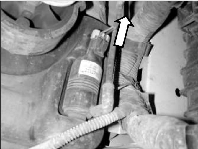
m. Unplug the washer motor. Pull the washer fluid hose off of the motor and drain the fluid into a clean suitable container.
