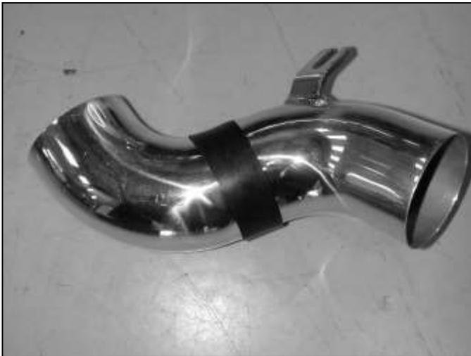
d. Mark the pipe approximately 1/2" above and below the hole in the fender. Remove the pipe and apply the adhesive neoprene material as shown. Reinstall the intake pipe as previously directed.
