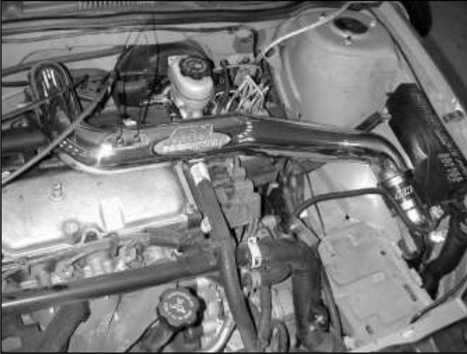
j. Place the upper intake pipe in the engine bay as shown.
