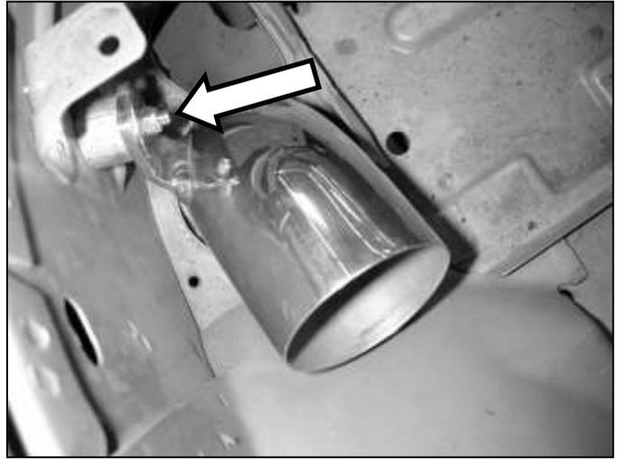
c. Install spacer as shown. Install the lower pipe in the engine bay. Center the pipe in the hole in the fender and tighten the nut on the spacer.
