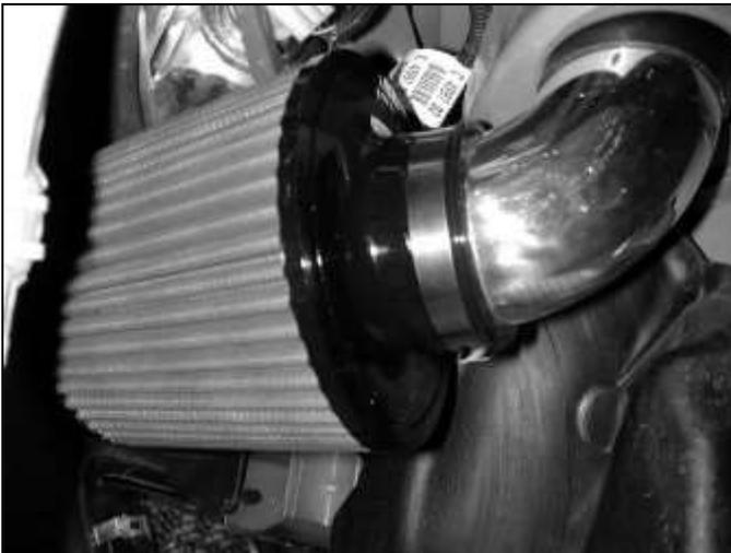
p. Install the air filter onto the end of the intake pipe.
