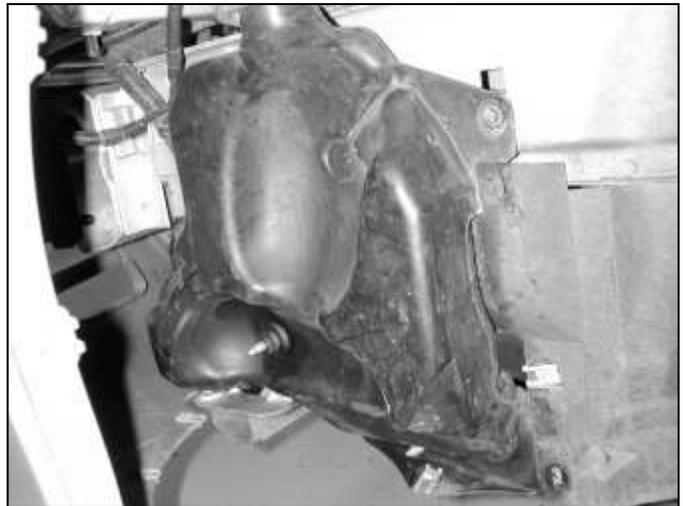
e. Reinstall the washer bottle without the lower air box. Reattach the washer fluid hose and plug in the washer motor.
