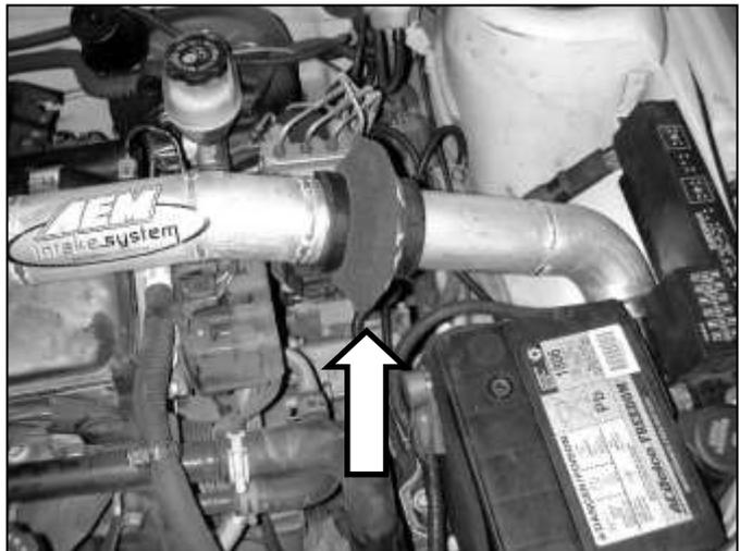
AEM® bypass valve installed.
