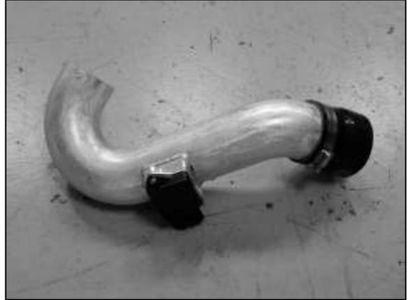
d. Install the 2.75" to 3" connector hose on the end of the upper intake pipe using the supplied hose clamp. Install the MAF sensor onto the intake pipe.
