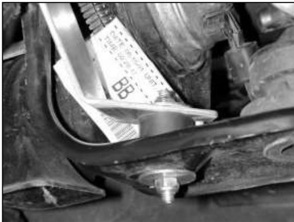
k. Install the lower intake pipe bracket on the rubber mount previously installed in step 3e.
