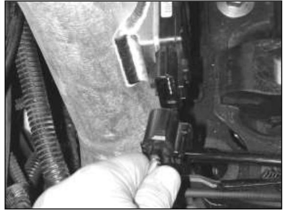
n. Plug in the wiring harness to the MAF sensor.
