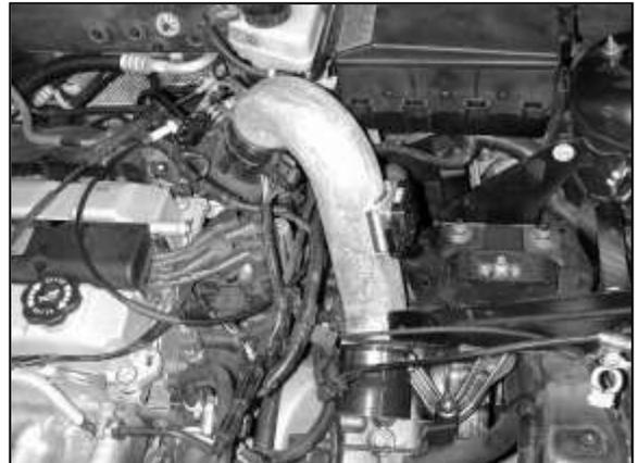
f. Install the upper intake pipe in place as shown.
