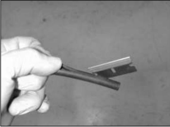
g. Cut the liner hose down the center of one side. Be careful not to cut all the way through the hose.
