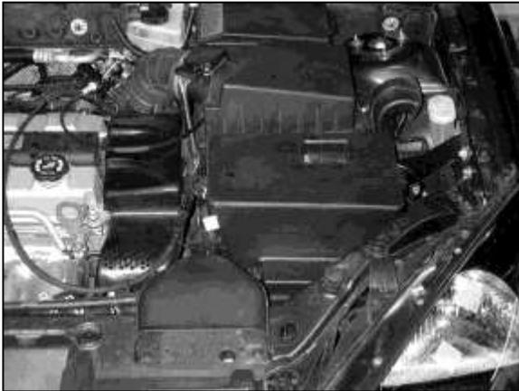
a. Factory air box system installed.
