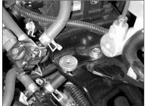
c. Place the supplied VSV bracket spacer in line with the hole exposed in the previous step.
