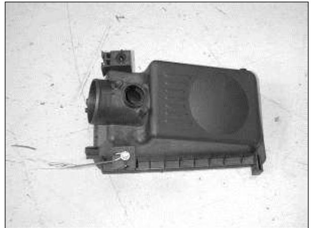
i. Remove the air box cover from the vehicle.
