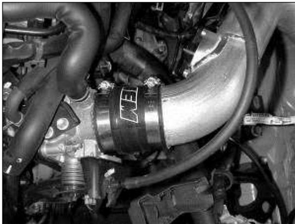
j. Loosely install the 2.75" silicone hose on to the AEM<sup>®</sup> intake pipe with the two #44 hose clamps. Insert the AEM intake pipe into the engine bay, filter end first. The pipe should pass under the bundle of wires going to the fuse box. Loosely secure the silicone hose to the throttle body.
