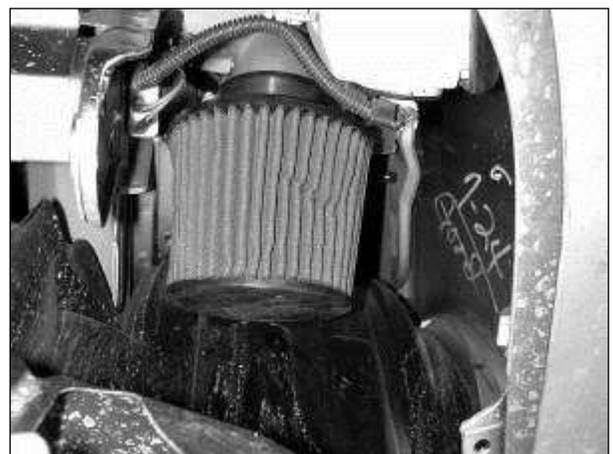
p. Install the AEM® air filter on the end of the AEM® intake pipe. Ensure the air filter does not contact any part of the vehicle and tighten the #48 hose clamp.
