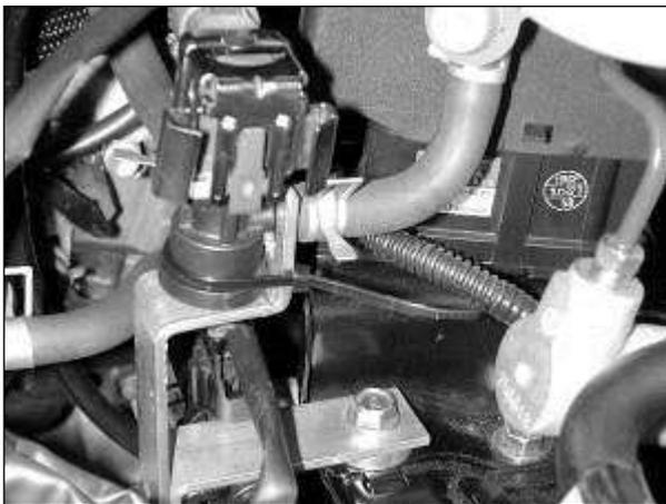
f. Use one of the supplied zip ties to secure the upper VSV to the bracket. Make sure the zip tie rests in the notches in the bracket to ensure that it does not slide off.
