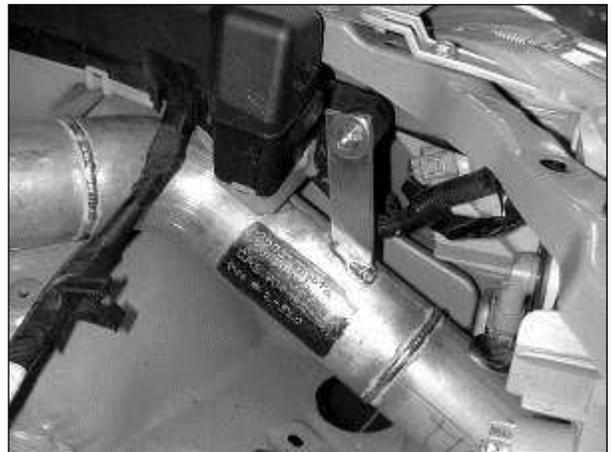
k. Loosely secure the bracket to the rubber mount with the supplied washer and locknut. Plug in the MAF sensor on the back side of the pipe.
