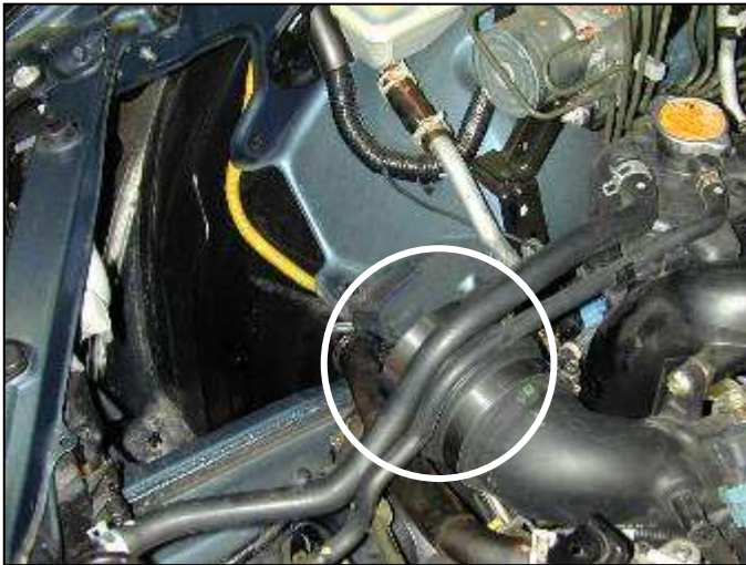
b. Attach 2.75" hump hose to the plastic turbo inlet. Attach hose clamps but do not tighten.
