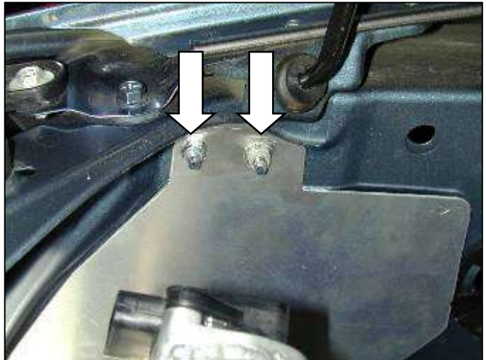
g. Place the heat shield over the intake pipe. Secure the heat shield to the upper two mounting studs left by the air box bracket.
