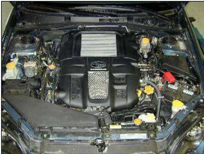
a. Factory air box system installed.
