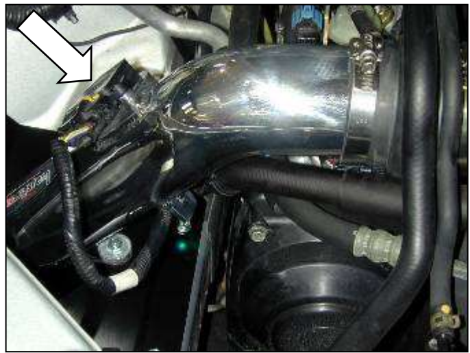
k. Plug in MAF Sensor. Secure MAF sensor with push-in zip tie to the tab on the underside of the intake pipe.
