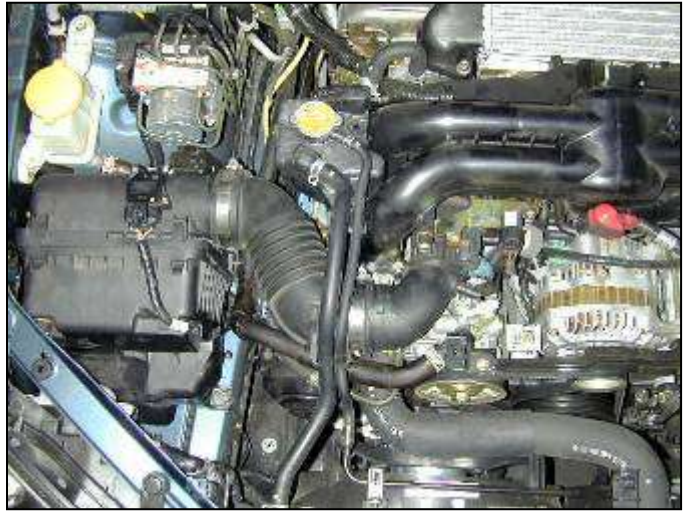
d. Unplug the MAF sensor.
