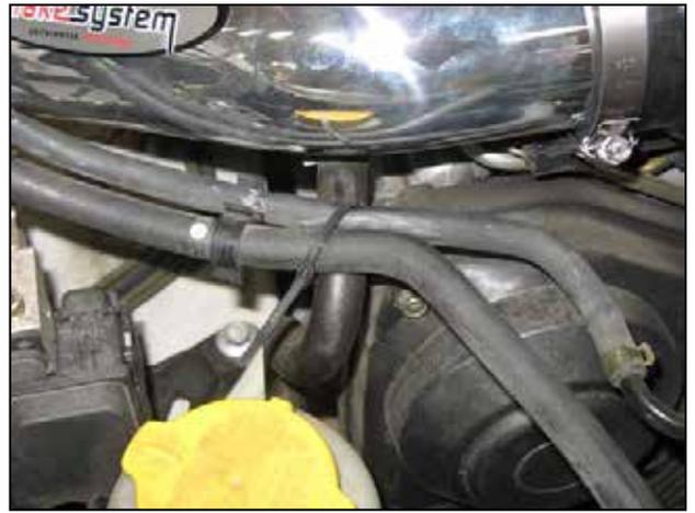
k. Secure the two rubber hoses to the rubber AC hose using the supplied 6" zip-tie. Trim excess plastic.
