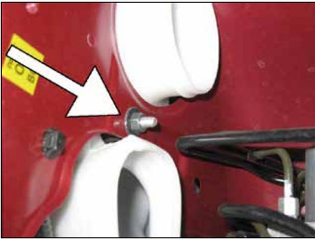
i. From the engine bay, remove the remaining nut securing the lower resonator.
