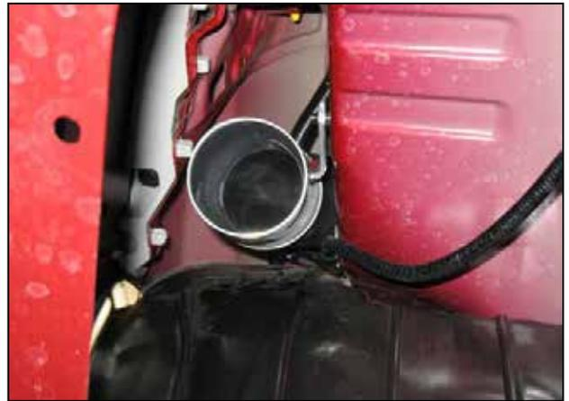
g. Install the lower intake pipe with the shorter side going into the 90° coupler. Rotate the pipe until the mounting bracket is aligned with the stud in the frame rail. Secure the intake pipe using a #48 hose clamp.
