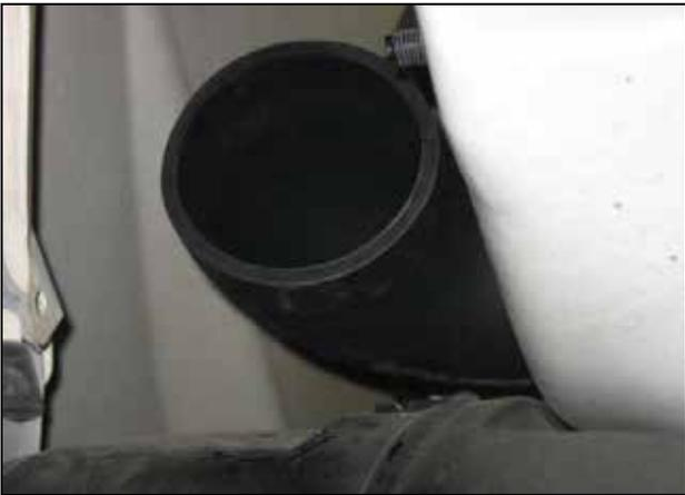
f. Install the 90° coupler by routing it through the inner fender hole and sliding it over the end of the upper intake pipe. Secure the coupler using a #44 hose clamp.
