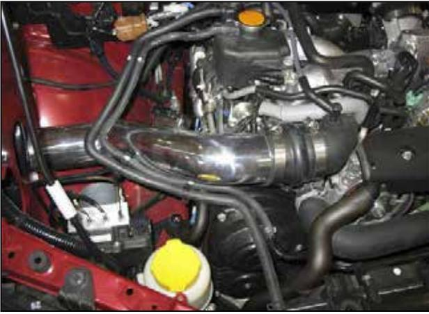
d. Install the upper intake pipe into the coupler on the turbo inlet. Rotate the pipe so that the filter end is centered in the hole in the inner fender. Secure the intake pipe using a #44 hose clamp.
