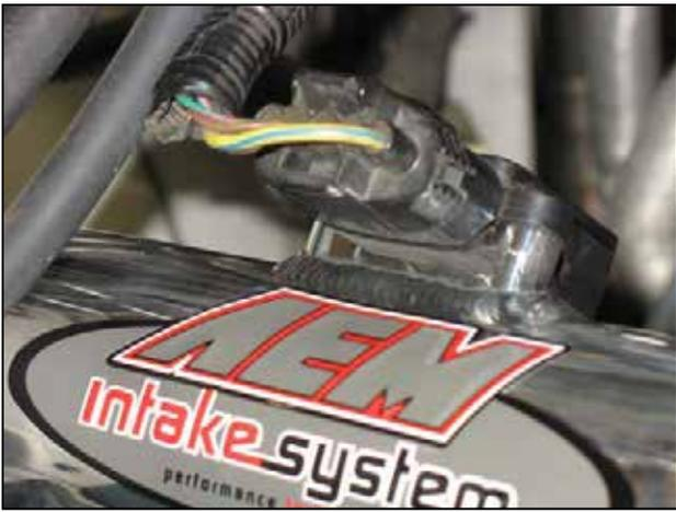
j. Plug the MAF sensor into the wiring harness.
