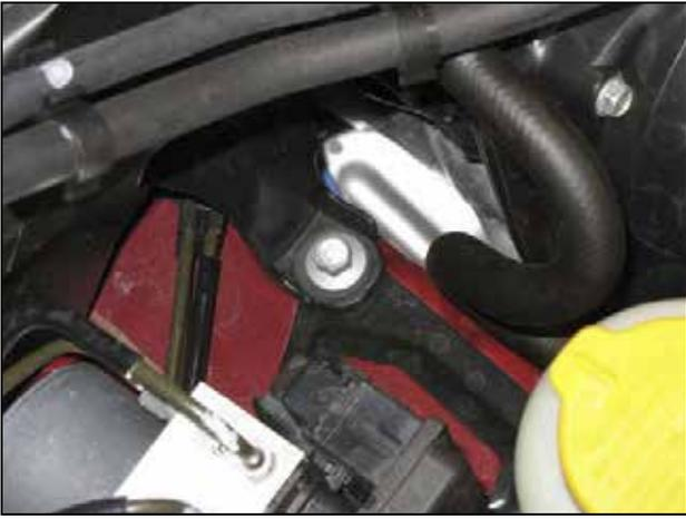
e. Down on the frame rail, on each side of the air box are the bolts that secure the air box in place. Remove the two bolts and gently lift out the air box assembly.
