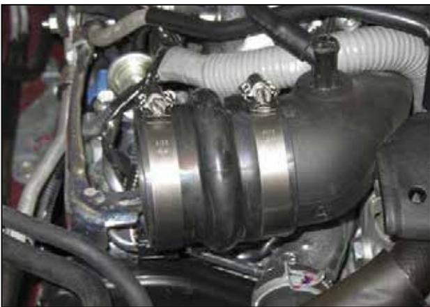
b. Install the hump hose coupler onto the stock turbo inlet tube and secure using a #44 hose clamp.
