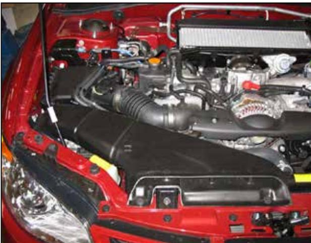
Stock air box system installed
