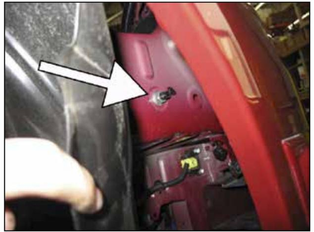
j. Locate the threaded stud behind the area where the lower resonator was mounted. Remove the nut on the stud and set it aside as it will be reinstalled later.
