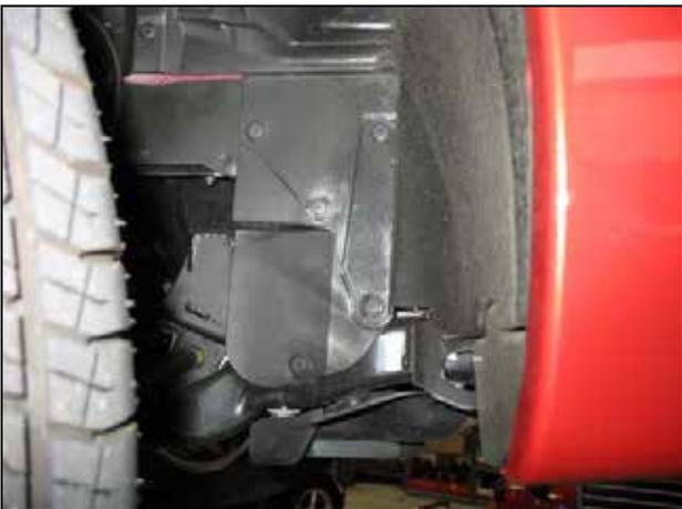
g. With the front wheels turned all the way to the right, locate the plastic clips just forward of the suspension holding the liner to the passenger side wheel well and remove them.
