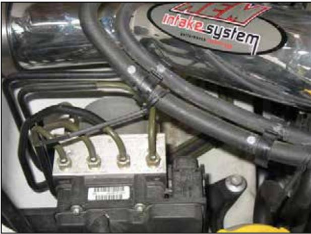
l. Secure the two rubber hoses to the steel brake tube using the supplied 6" zip-tie. Trim excess plastic.
