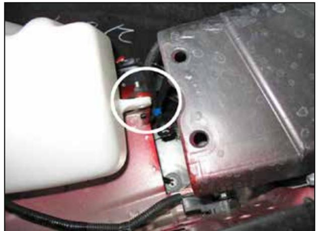
h. Move the wheel well liner to expose the lower resonator. Remove the lower nut securing the resonator to the chassis.
