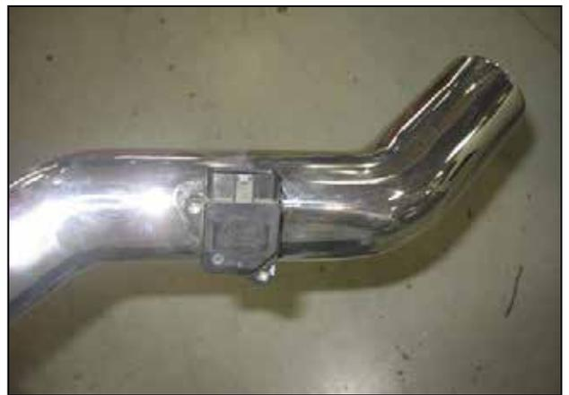
c. Using the two supplied 8-32 bolts, install the MAF sensor into the upper intake pipe.
