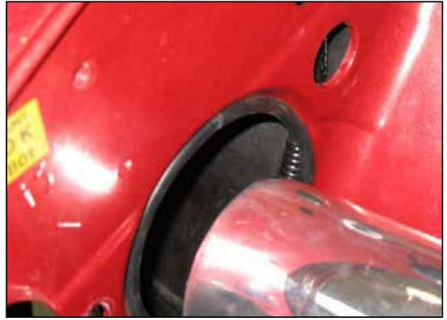
e. Install the rubber edge trim around the hole in the inner fender where the factory intake system was routed.
