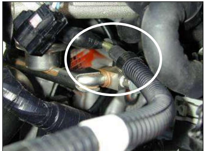
c. Follow the vacuum hose from the air box up to the plastic vacuum fitting under the throttle body. Carefully pull the vacuum hose off of the fitting. Be careful not to break it. Remove hose from vehicle.
