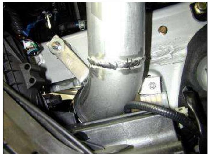
i. Secure the pipe with the supplied washers and lock nuts. Do not completely tighten lock nuts.
