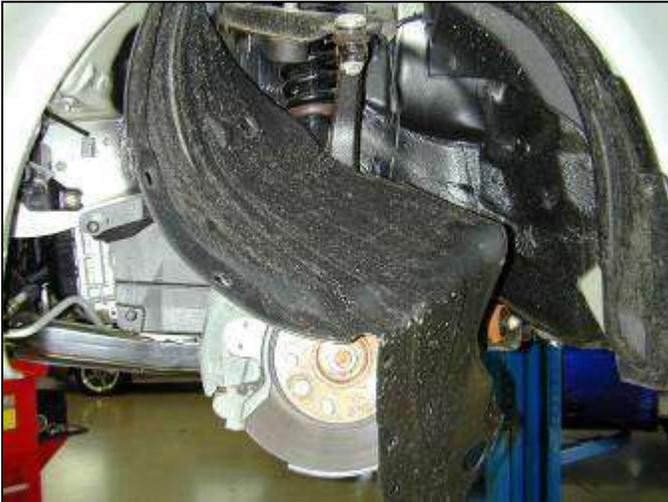
k. Place the partially removed fender liner as shown.
