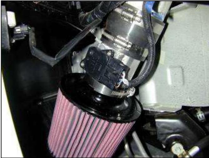
l. Attach the air filter apparatus as shown. Route the stock air flow sensor wiring harness through the hole in the fender and plug it into the sensor as shown. Again check the position of the air flow meter and confirm that is positioned as shown above.
