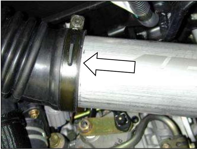
j. Secure the upper end of the pipe utilizing the stock inlet hose and clamp. A small amount of WD-40 on the end of the pipe may ease installation.
