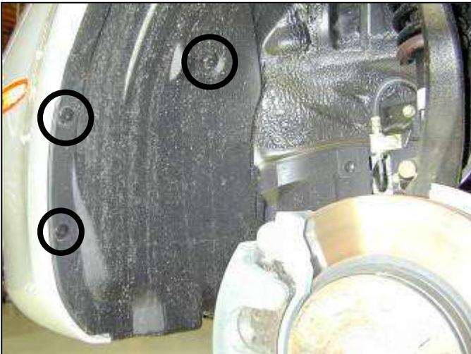
i. Release plastic clips inside the fender.
