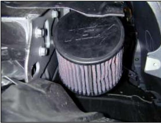
l. Attach the AEM air filter element onto the end of the inlet pipe. Make sure the air filter clears the body and splashguard. Secure the air filter's hose clamp.
