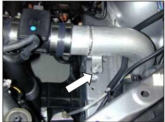
m. Secure inlet pipe at the bracket on the rubber mount.
