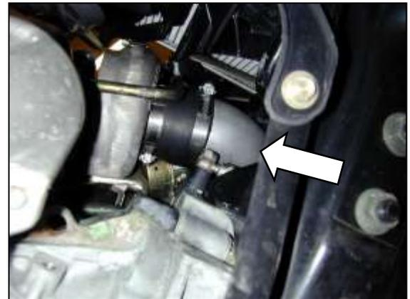
c. Attach the reducer coupler, hose clamps and inlet pipe to the turbo inlet. Make sure to clear the fan shroud. Use the 2.5-2.75" coupler.
