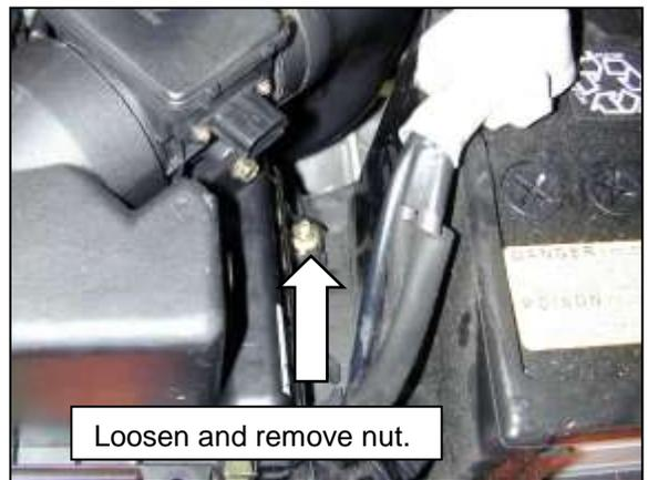
Loosen and remove nut.
