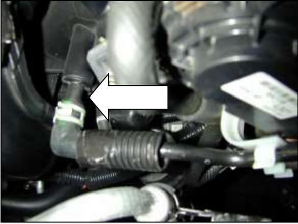
q. **NOTE: 2007-2008 models do not have vacuum solenoid. Proceed to step r.** Pull the vacuum hose off of the nipple on the intake manifold as shown.
