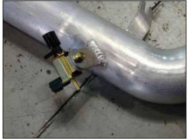
e. **NOTE: 2007-2008 models do not have vacuum solenoid. Proceed to step 3g.** Attach the vacuum solenoid to the intake pipe using the supplied flat washer and the previously removed nut.
