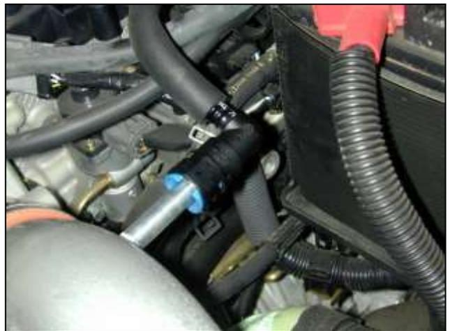
o. Plug the plastic breather hose onto the nipple on the intake pipe.
