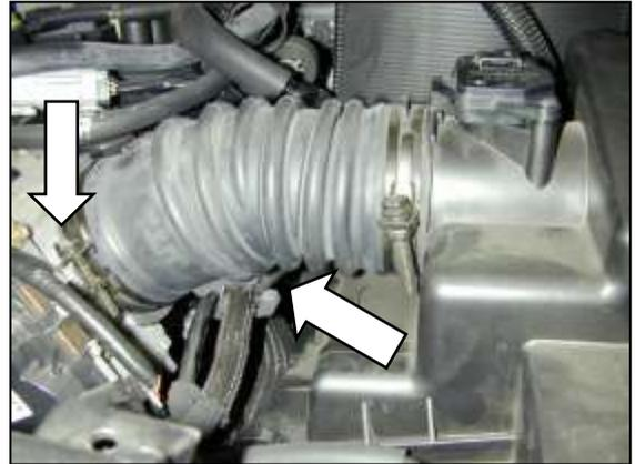
f. Loosen the hose clamp at the throttle body. Unhook the hoses from the bottom of the inlet hose. Pull the inlet hose off of the throttle body.
