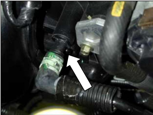
f. Cover the open nipple exposed during step 2q with the supplied vacuum cap.
