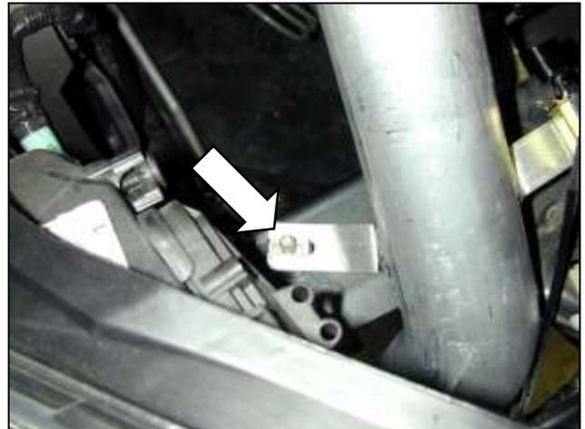
k. Secure the pipe bracket to the rubber mount using a flat washer and 8mm nut.
