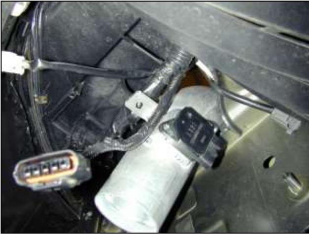
l. Route the MAF sensor harness through the hole where inlet pipe is located. From underneath the vehicle, plug the MAF harness into the MAF sensor mounted on the inlet pipe.
