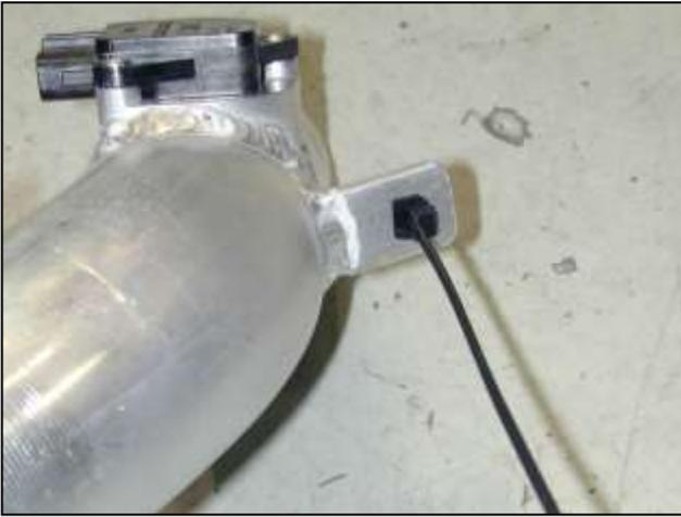
d. Install the supplied tree mount zip-tie into the bracket with the 1/4" hole on the pipe.
