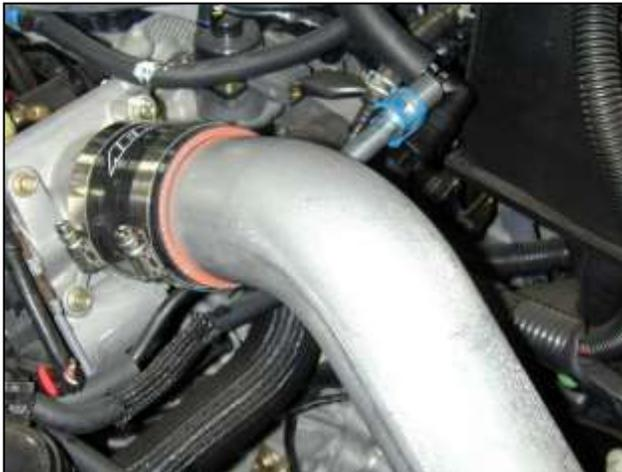
j. Slide the pipe into the silicone coupler on the throttle body and secure using a #44 hose clamp.
