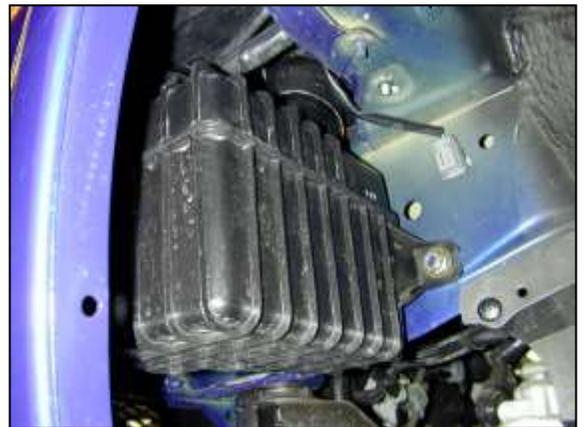
l. Remove the three nuts that secure the lower resonator to the chassis.
