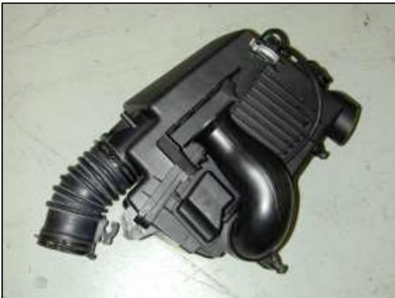
g. Gently pull the air filter housing up and out of the engine bay.
