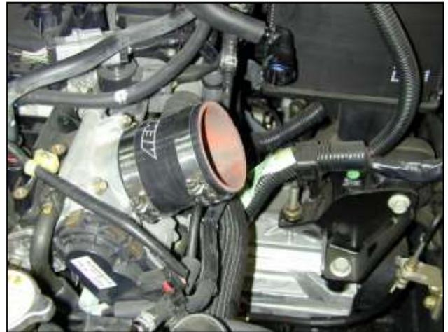
g. Attach the silicone coupler to the throttle body using the supplied #44 hose clamp.
