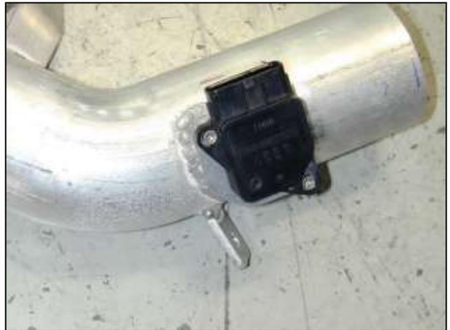
c. Install the previously removed MAF sensor into the inlet pipe using the two supplied bolts.
