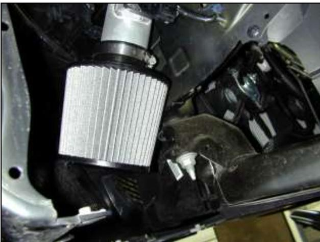
n. Install the AEM<sup>®</sup> air filter on to the end of the inlet tube. Push the air filter over the inlet pipe until the stop in the air filter is reached. Install and fully tighten one #48 hose clamp to secure.
