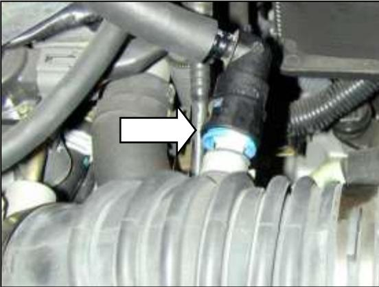
e. Remove the plastic crankcase breather hose by pinching the blue connector and pulling on the hose.
