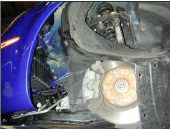
k. Move the fender liner so the lower resonator becomes accessible.
