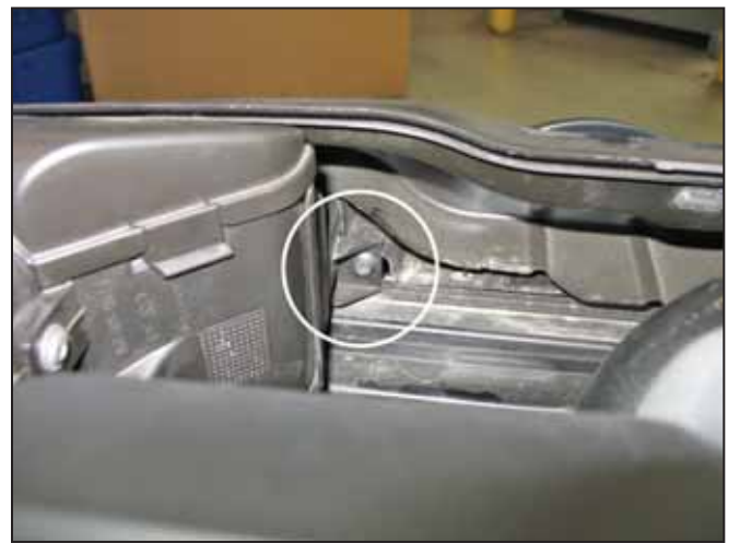
d. Remove the remaining screw securing from the inlet duct as shown.
