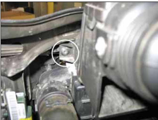
c. Remove the two torx-head screws securing the inlet duct to the radiator support. Remove the first screw shown above.
