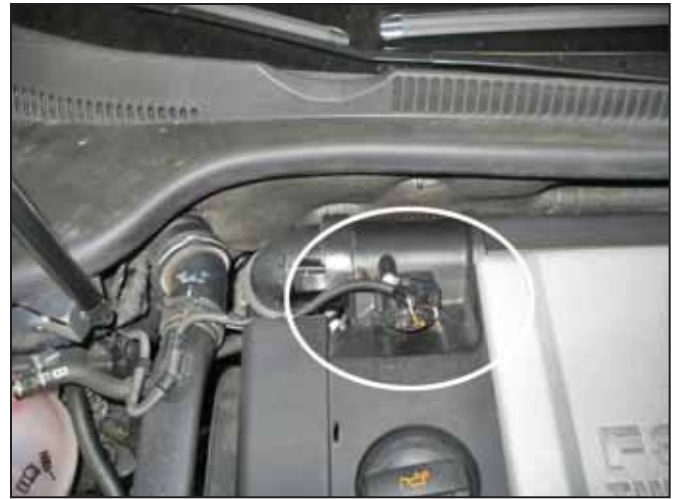
b. Unclip the MAF sensor harness from the engine cover. Unplug the harness from the sensor.
