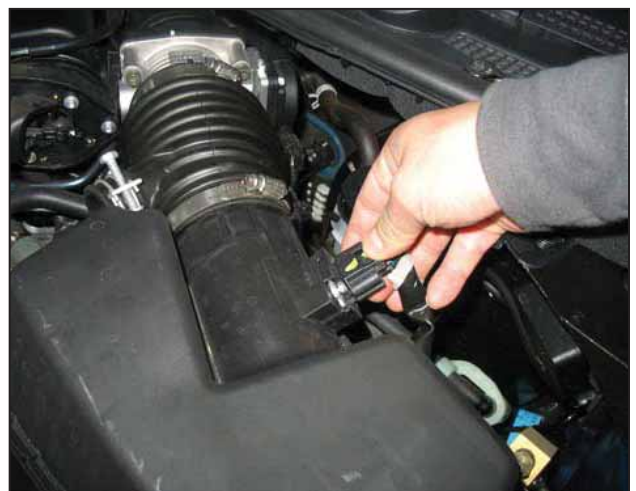
j. Unplug the Mass Air Flow (MAF) sensor harness connector from the sensor.
