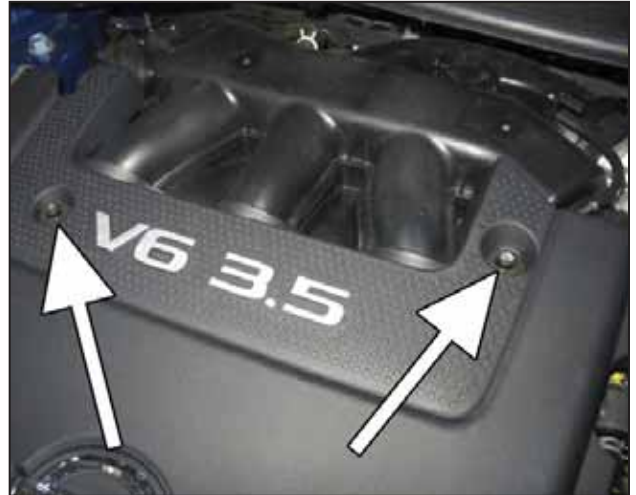
b. Loosen and remove the socket cap head screws on the engine cover.
