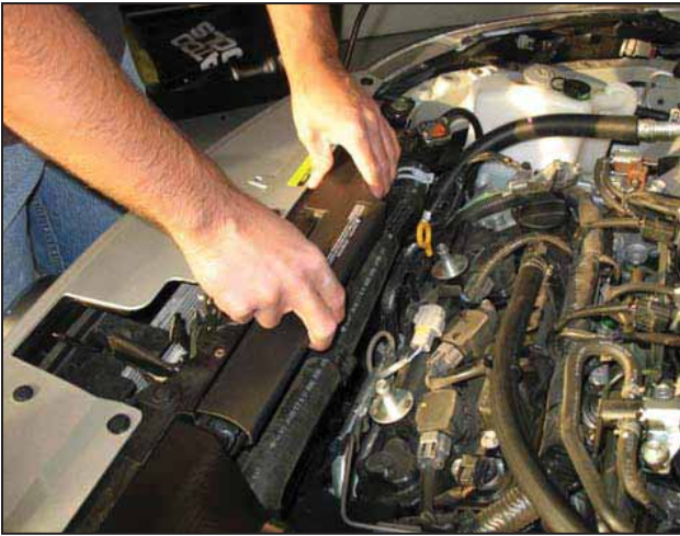
af. Install the factory plastic radiator trim as shown.
