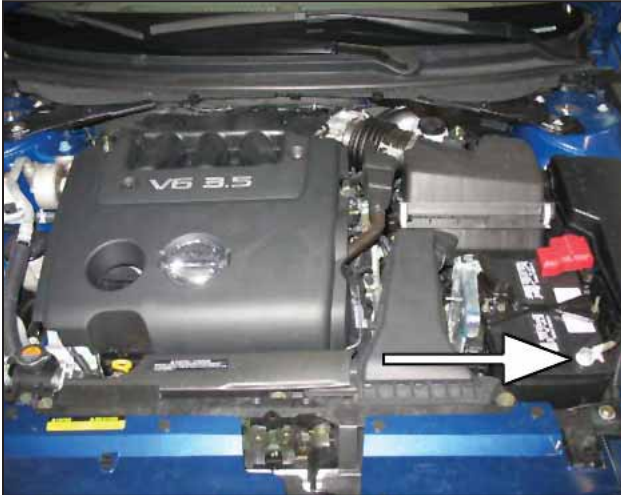
a. Open the hood and disconnect the negative battery cable.
