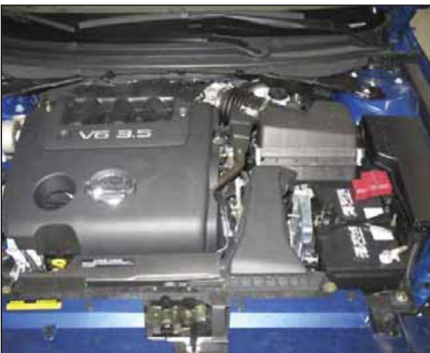
Factory air box system installed
