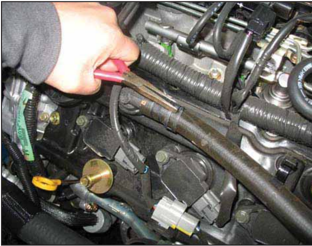
k. Slide the PCV hose clamp off of the engine's PCV port.
