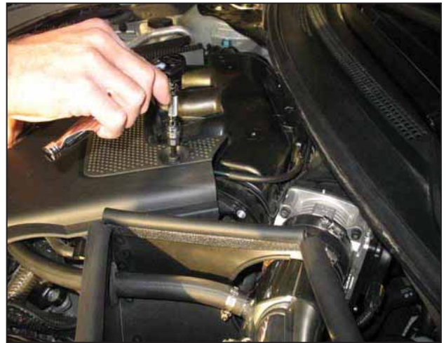
ai. Secure the engine cover with the hardware removed in step 2b.
