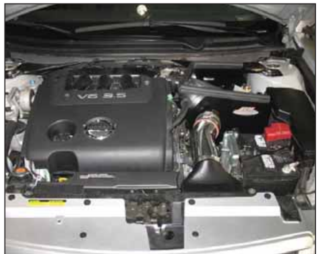
AEM® intake system installed
