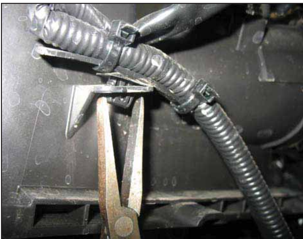
o. Remove the MAF sensor harness clip from the back of the air box lid.
