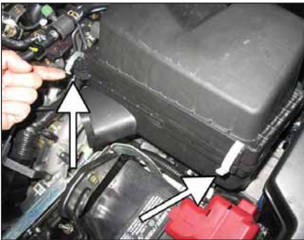
m. Unclip the two metal clips on the air box.
