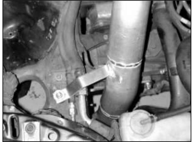
g. Align the aluminum mounting tab with the rubber mount installed earlier in step #4e. Use the supplied nylock nut and washer to secure the bracket in place. Refer to the diagram below on the next page for proper rubber mount installation.
