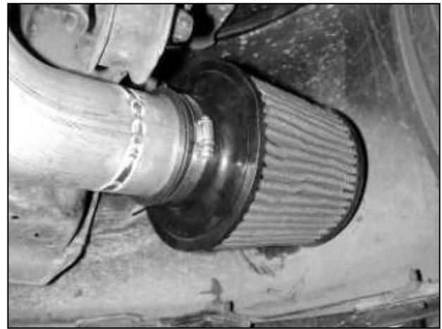
h. Install the AEM® air filter onto the inlet pipe. Once proper fitment is achieved, secure the air filter in place with the supplied hose clamp.
