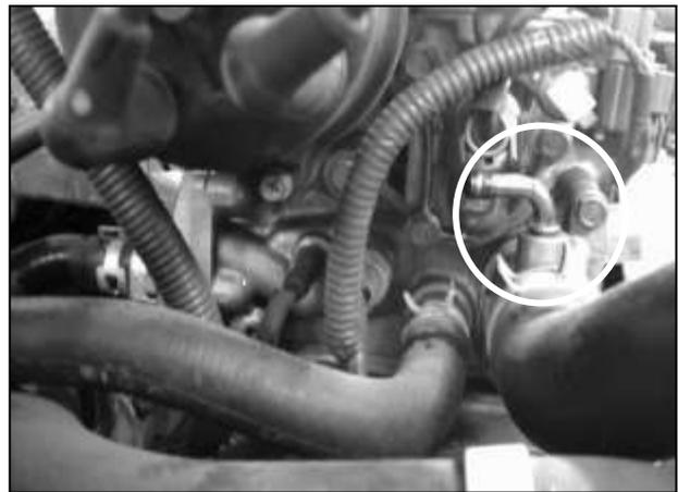
c. Remove the other end of the water bypass hose from the fitting on the engine. Install the opposite end of the 5/16" hose onto this fitting and secure in place with a 3/4" hose clamp. **NOTE:** Replace any coolant recovered during the water bypass hose removal by replenishing the recovery tank.
