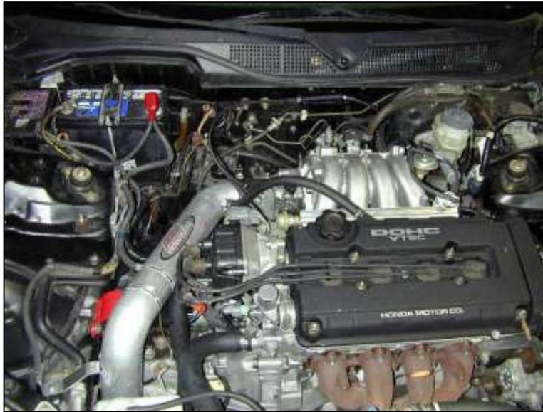
AEM® intake system installed
