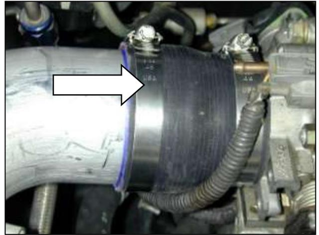
g. Insert the upper end of the pipe into the coupler. Do not tighten the hose clamps.
