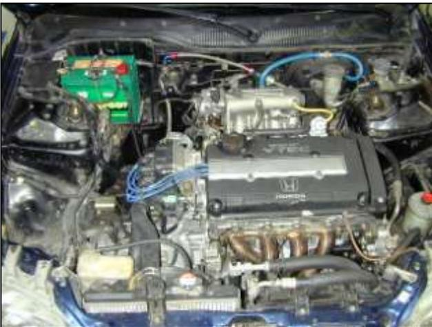
a. Factory air box system removed.
