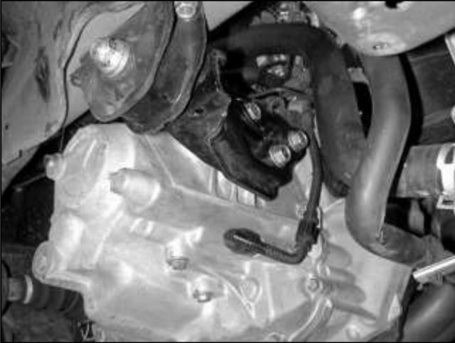
a. Using a 19mm socket, remove the engine mount nut. Also remove the three 17mm bolts and remove the mount.
