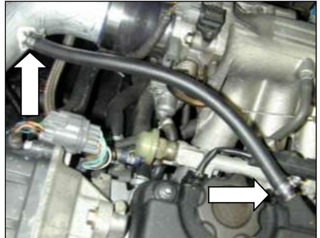
i. Connect the breather nipple on the valve cover to the nipple on the intake pipe as shown. Secure each end with the supplied hose clamps.
