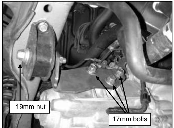
d. Using the supplied bolts, install the AEM<sup>®</sup> engine mount on the transmission; torque the bolts to 61ft-lbs. Also install the factory 19mm nut and washer on the mounting stud.
