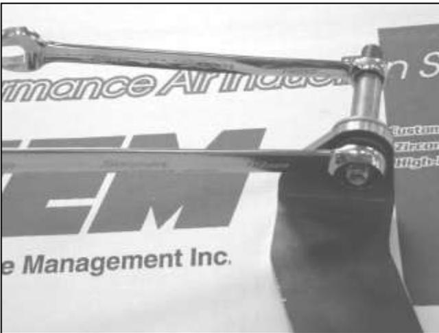
c. Install the factory mounting stud on the supplied engine mount bracket using the supplied nylock nut and washer.
