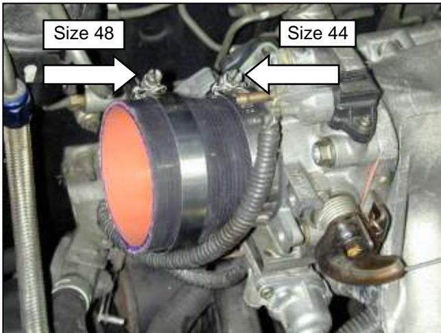
b. Install the coupler on the throttle body as shown. Place the hose clamps over the coupler using the #44 clamp on the throttle body.
