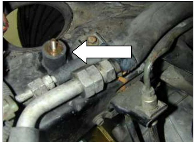
c. Install the rubber mount into the frame rail.
