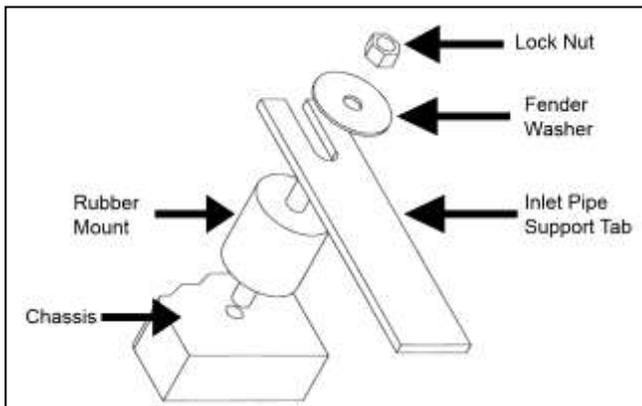
d. Proper installation of the rubber mount assembly.
