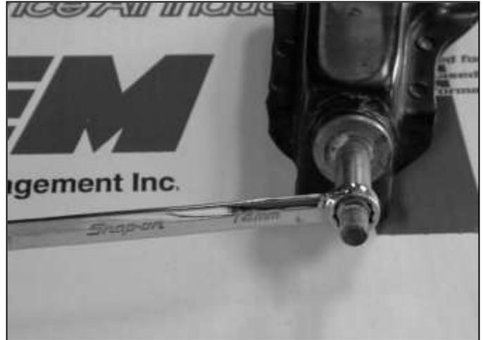
b. Using a 14mm wrench, remove the mounting stud from the factory engine mount assembly.
