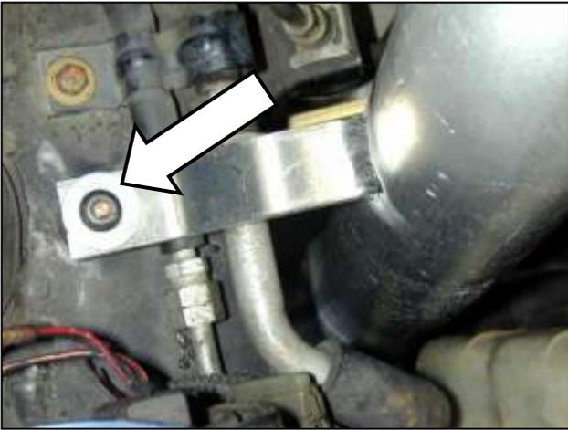
f. Install the washer and the lock nut onto the rubber mount.
