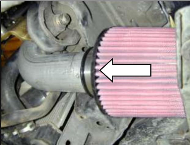
h. Install the air filter onto the lower end of the inlet pipe. Tighten the hose clamp.
