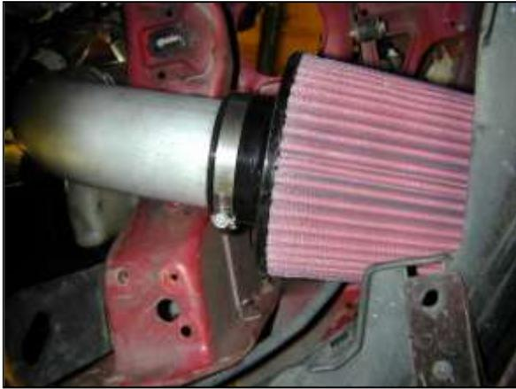
h. Install the AEM<sup>®</sup> air filter on the end of the inlet pipe. Once proper fitment is achieved, secure the air filter in place with the supplied hose clamp.
