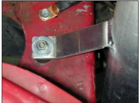
g. Install the lower inlet pipe. The inlet pipe's mounting bracket will line up with the rubber mount installed earlier. Secure in place with the supplied washer and M6 nut.
