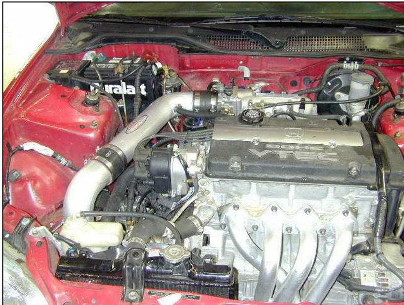
AEM<sup>®</sup> intake system installed
