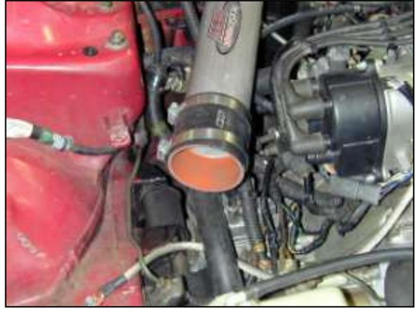
e. Install the supplied 3" coupler onto the upper inlet pipe as shown. Secure the coupler with a #48 hose clamp.
