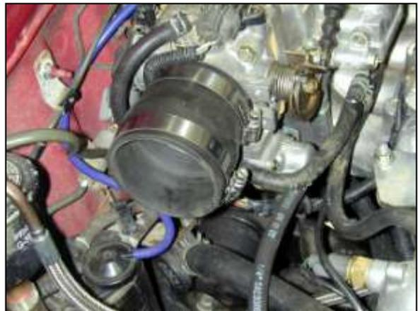
c. Install the supplied hose adapter onto the throttle body using the supplied #44 and #48 hose clamps. Use the #44 hose clamp on the throttle body side.
