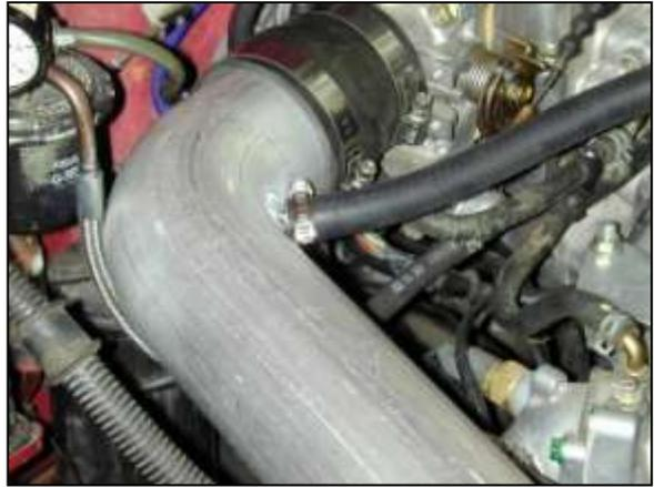
i. Attach the supplied 1/2" breather hose to the upper inlet pipe's nipple and the valve cover nipple. Secure each end of the breather hose with a 3/4" hose clamp.
