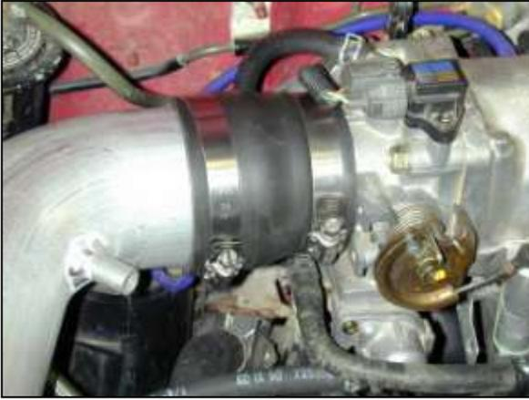
d. Attach the upper inlet pipe onto the hose adapter secured to the throttle body.
