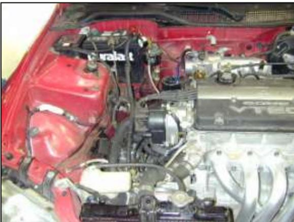
b. Engine bay with factory airbox system removed.
