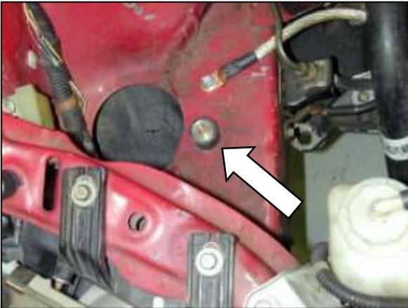
f. Install the supplied rubber mount into the hole in the engine compartment as shown. The hole is located in front of the passenger side shock tower where the stock airbox system was mounted.
