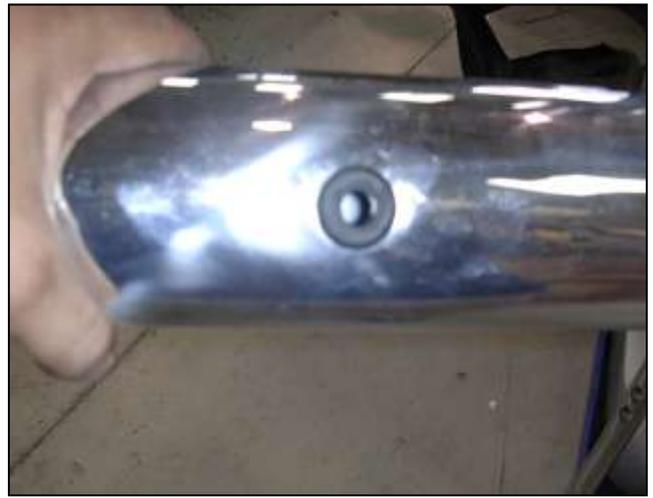
e. Install the supplied grommet into the intake pipe as shown.
