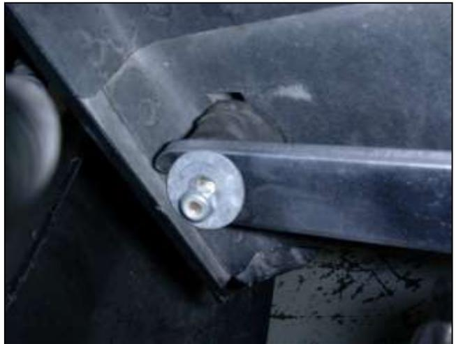
g. Slide the intake pipe's mounting bracket onto the rubber mount, and secure in place with the supplied washer and nut.
