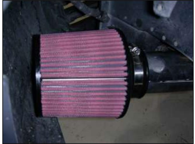
i. Install the AEM® air filter onto the end of the inlet pipe and secure in place with the supplied hose clamp.
