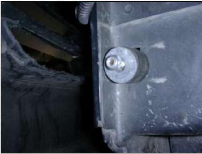
d. Locate the hole on the driver side frame rail in the front area of the vehicle. Install the supplied rubber mount into the hole as shown. Install the supplied washer and nut into the rubber mount.
