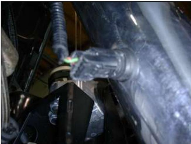
j. Install the inlet air temperature sensor into the grommet installed earlier in step #3e.
