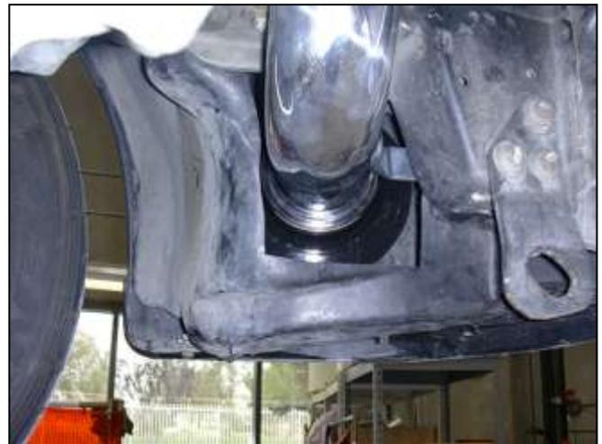
k. The fender liner must be trimmed for the intake system to fit properly.
