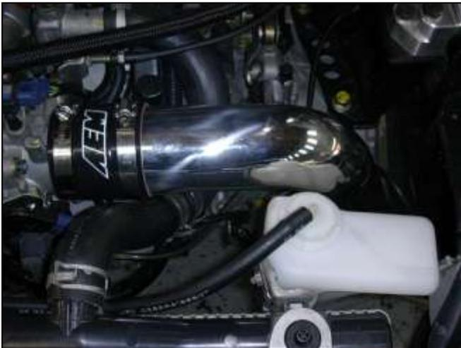
f. Insert the inlet pipe into the hose adapter and align the mounting bracket with the rubber mount installed in step #3d.
