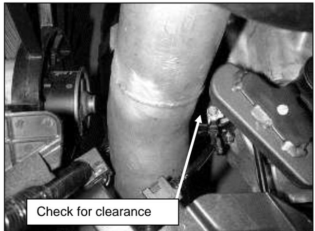
p. Check for clearance between the intake pipe and the shift arm. Watch the arm as it is shifted through its full range of motion and ensure proper clearance.
