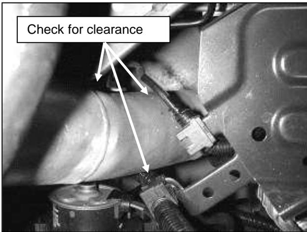
q. Check for clearance between the intake pipe and surrounding objects.
