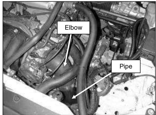
h. Install the intake pipe into the lower end of the connector elbow as shown.
