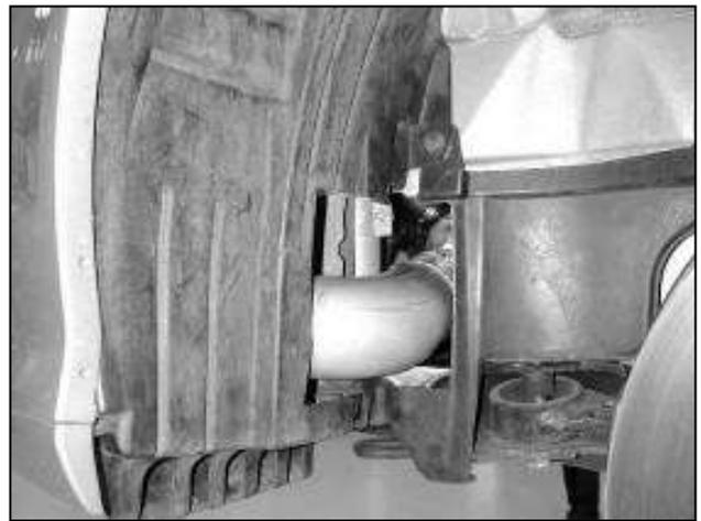
r. Install the left fender well lining and lower splashguard that were removed in step 1eii. The fender liner must be trimmed for the intake system to fit properly. Trim and reinstall the fender liner as shown. Failure to do so will void the warranty.
