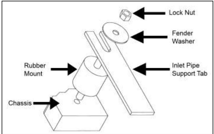
i. Secure the mounting bracket to the rubber mount with the supplied washer and nylok nut.
