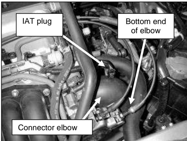
e. Using a supplied hose clamp (9444), install the supplied connector elbow onto the throttle body. Reconnect the IAT sensor. Slide supplied hose clamp (9444) onto the bottom end of elbow in preparation for the intake pipe installation.
