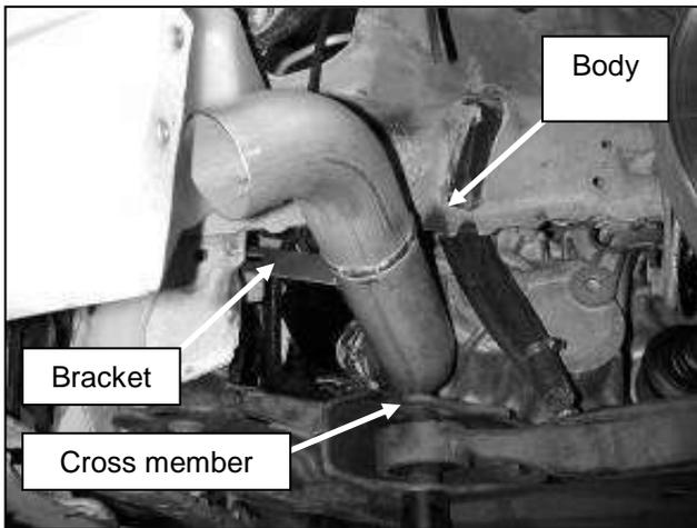
g. For ease of installation, route the intake pipe between cross member and body with bracket oriented to the upper left as shown.
