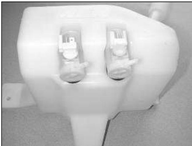
e. Reinstall the two pump grommets and the fill tube grommet on the replacement washer bottle as shown. Wet the grommets with soapy water and insert the two washer pumps and fill tube.
