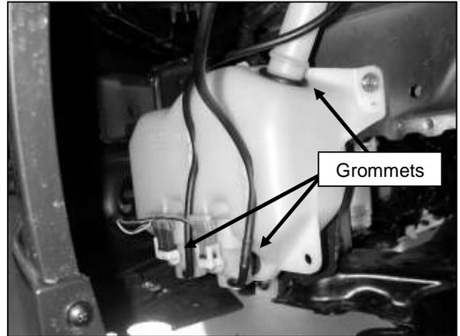
d. Remove the two pumps by pulling them from the rubber grommets. Remove the two grommets from the washer bottle along with the grommet for the filler tube.
