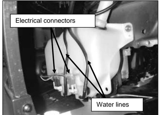
b. Remove the electrical connectors and water lines from the windshield wiper motors. Drain the washer bottle fluid into a clean container.
