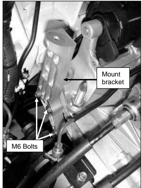
f. Remove the three M6 bolts that secure the air box support bracket and save them for later use. Remove the air filter box mount bracket.
