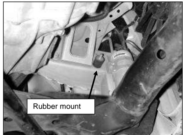
f. Remove the bolt under the battery tray and replace it with the supplied rubber mount as shown.
