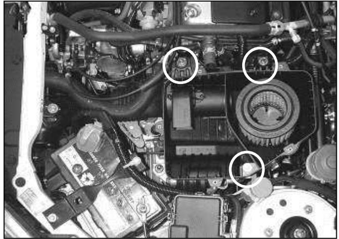
d. Loosen the two M6 bolts and the M6 nut securing the air filter box and remove it.
