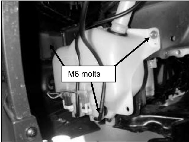
c. Remove the three M6 bolts securing the washer bottle in place. Pull the filler tube out of the bottle.
