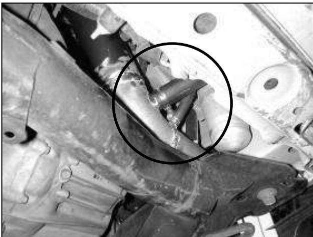
o. Connect the 3/4" and 3/8" hoses to the intake pipe and secure with the supplied clamps as shown.
