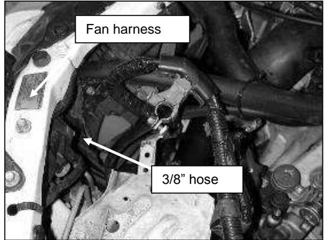
n. Route the 3/4" breather tube behind the fan wiring harness. Route the 3/8" hose between the fan shroud and battery tray as shown.
