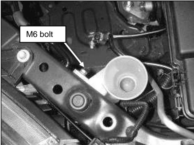
a. Remove the M6 bolt securing the washer bottle filler neck. Remove the washer bottle filler neck by pulling it up.
