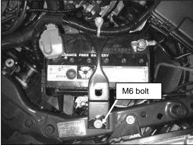
g. Remove the positive cable from the battery. Remove the M6 bolt securing the battery tie down in place. Remove the battery and trays.
