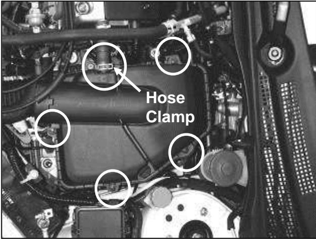
c. Loosen the 5 Phillips head screws and remove the air filter box cover. Also disconnect the breather hose by releasing the hose clamp.
