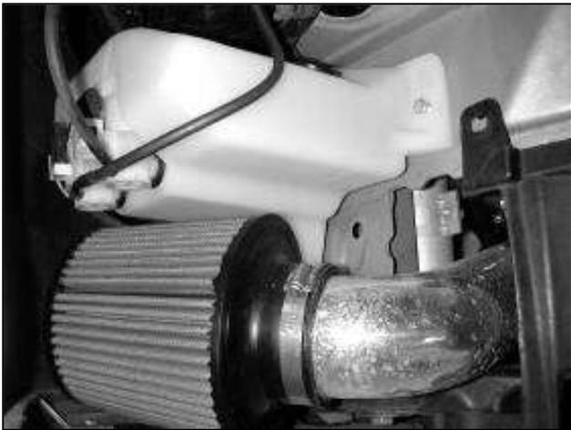
k. Install the AEM<sup>®</sup> air filter onto the lower end of the intake pipe.
