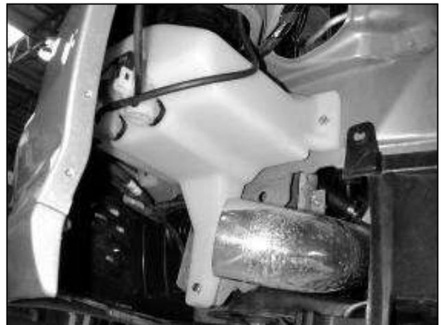
f. Secure the new washer bottle with the three air box bracket bolts removed in step 3c. Reconnect the two feeder lines and the two electrical connectors to the pumps.
