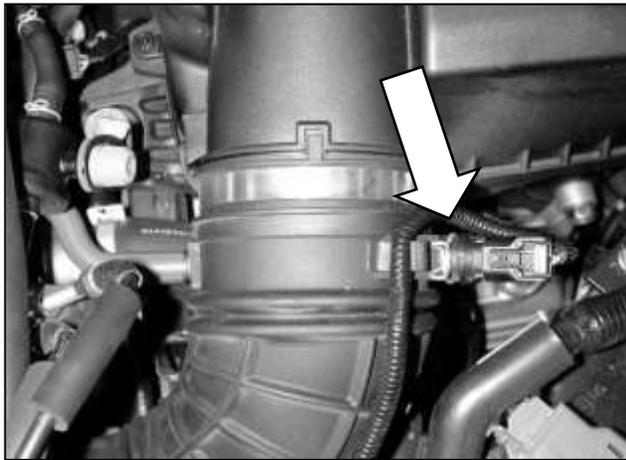
e. Remove the IAT sensor and the thermal valve hose from the inlet tube. Also, disconnect the thermal valve hose from the thermal valve. Finally, remove the inlet tube.
