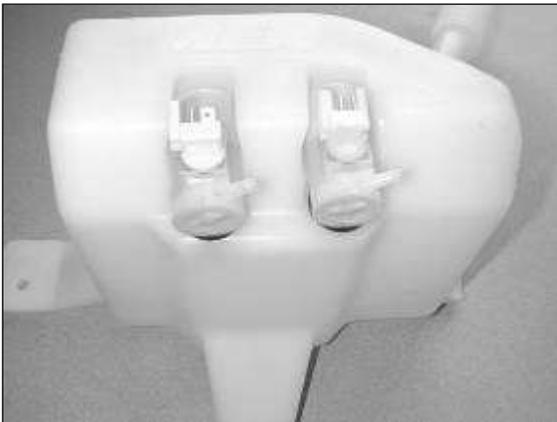
e. Reinstall the two pump grommets and the fill tube grommet on the replacement washer bottle. Wet the grommets with soapy water and insert the two washer pumps and fill tube.
