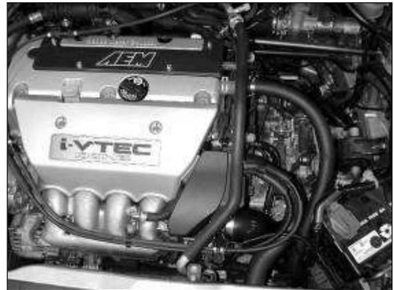
AEM® intake system installed.
