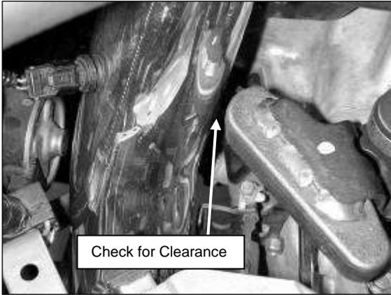
o. Check for clearance between the intake pipe and the shift arm.
