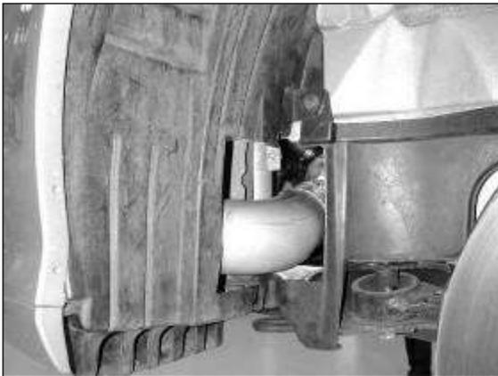
q. The fender liner must be trimmed for the intake system to fit properly.
