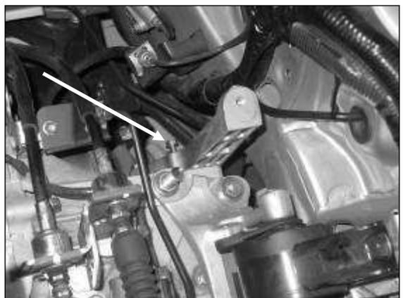
n. Remove the three bolts that secure the air box support bracket and save them for later use.
