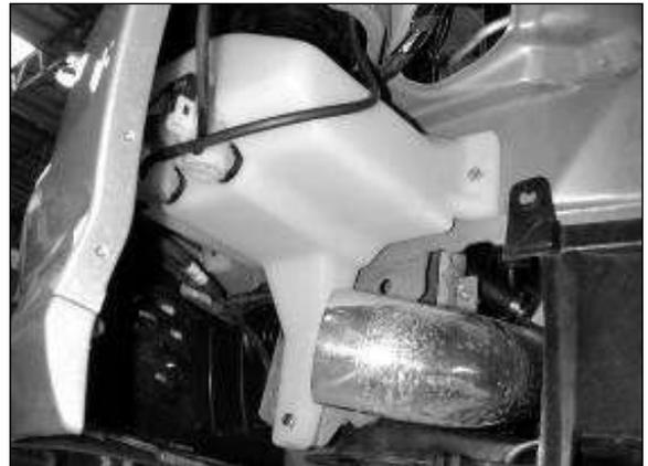
f. Secure the new washer bottle with the three air box bracket bolts removed in step 2n. Reconnect the two feeder lines and the two electrical connectors to the pumps.
