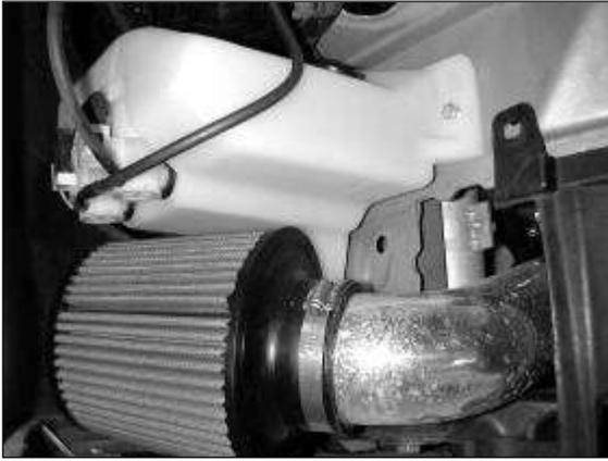
i. Install the AEM<sup>®</sup> air filter onto the lower end of the intake pipe.
