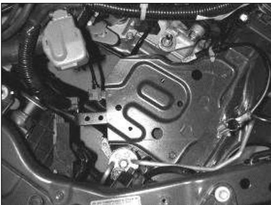
b. With a pair of pliers bend the positive battery cable hold tab 90 degrees.
