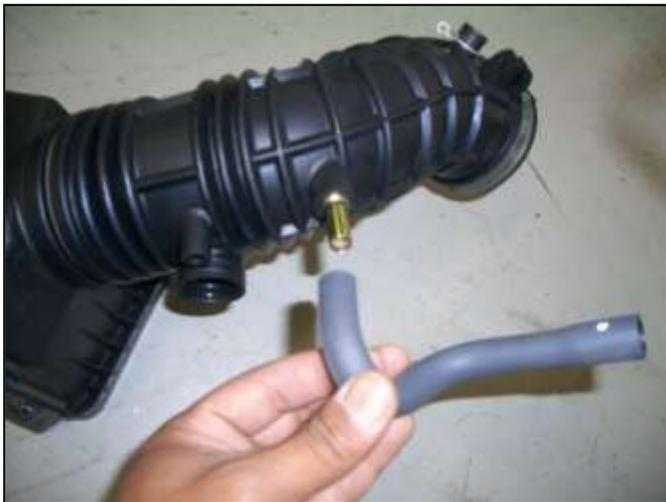
g. Remove the small hose from the factory intake system.
