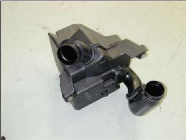
o. Remove the resonator assembly from the vehicle.
