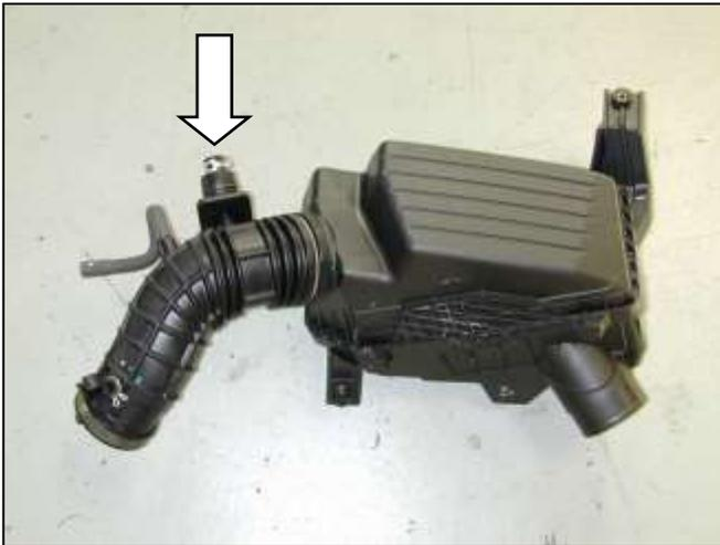
e. Carefully remove the airbox assembly from the engine bay. Remove the oil trap from the inlet duct and retain the clamps for later use.
