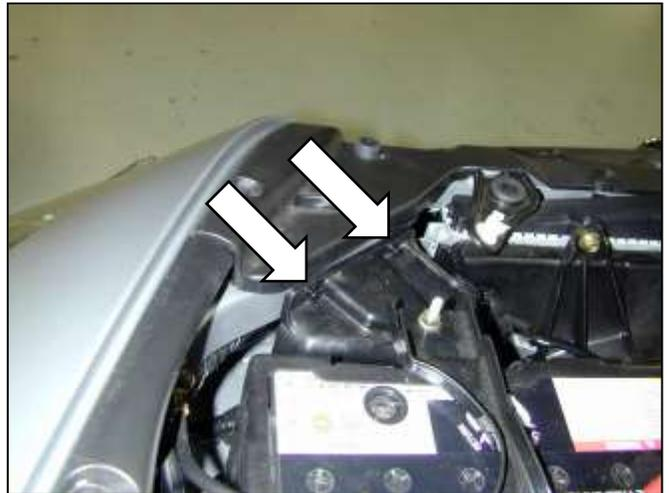
f. Remove the two fasteners securing the plastic cover in front of the battery.
