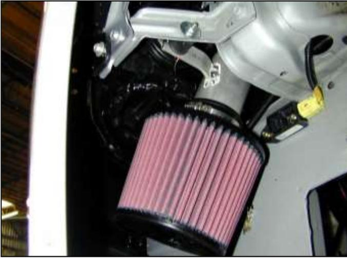
i. Install the air filter on the end of the intake pipe and tighten the hose clamp.
