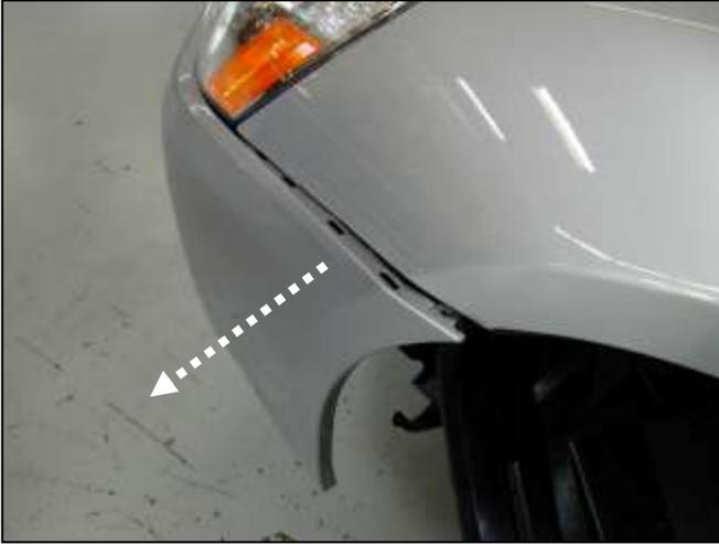
m. Unsnap the corner of the bumper cover as shown in the picture. This will help in the removal of the resonator assembly.
