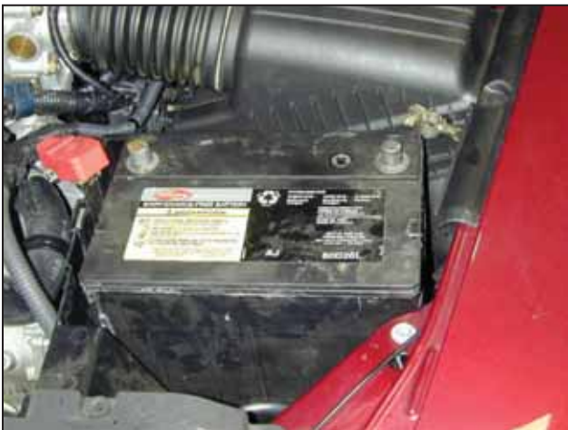
c. Remove the battery tie down and the two J-bolts securing it. Carefully lift the battery out of the engine compartment and set aside in a safe place.
