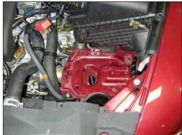
d. Unclip the plastic battery shroud from the positive terminal wire and remove the shroud.
