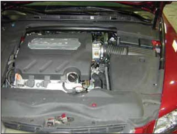
a. Factory air box system installed.
