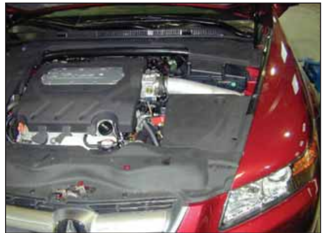
AEM® intake system installed
