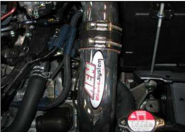
j. From under the vehicle, slide the lower intake pipe up and into the previously installed coupler. Align the bracket with the rubber mount installed in step 3c.
