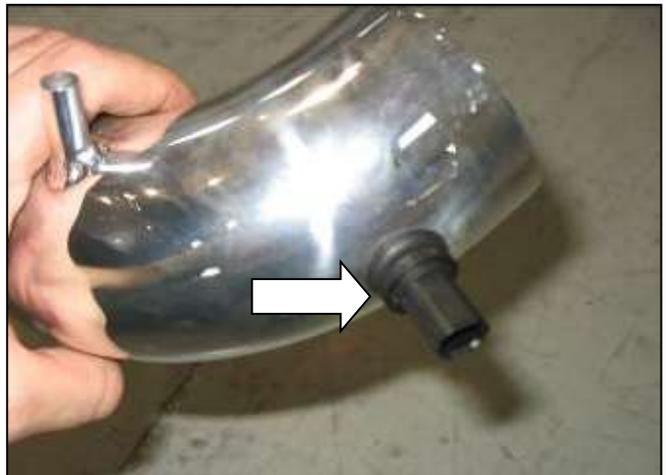
e. Carefully install the IAT sensor into the grommet. Fitment may be tight, if so use soapy water to ease installation.
