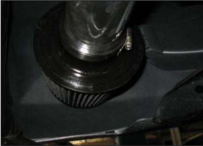
l. From under the vehicle, install the AEM® Dryflow™ air filter onto the end of the lower pipe. Push the air filter onto the intake pipe until the stop inside is reached. Then secure the air filter using a #48 hose clamp.
