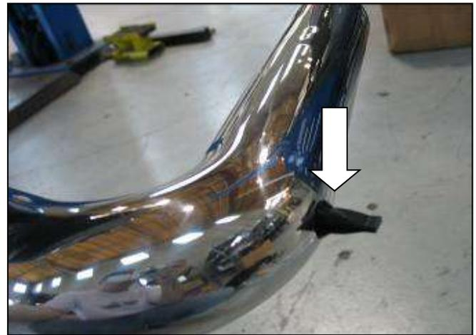
i. Locate the hole on the lower intake pipe and insert the supplied duck bill drain as shown.
