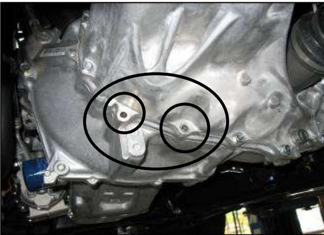
q. Remove the two bolts from the transmission housing shown above. These will be replaced in step 3b.
