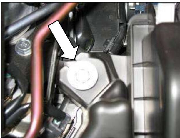
e. Remove the two bolts securing the air filter housing and upper resonator to the vehicle. Start with the bolt closest to the engine.
