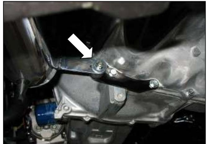
k. With the intake pipe bracket aligned with the rubber mount, install a washer and serrated nut to secure.
