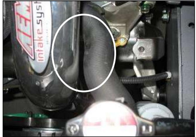
m. Check for clearance around the lower pipe. If the radiator hose is too close or touching, gently bend its support bracket for clearance. Once clearance has been verified, tighten all hose clamps and the nut on the rubber mount.
