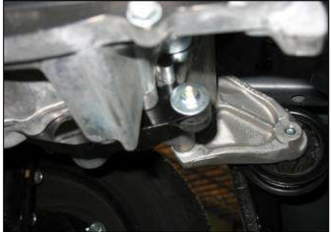
c. Install the supplied rubber mount into the previously installed transmission bracket using a flat washer and serrated nut. The rubber mount should face the driver's side.
