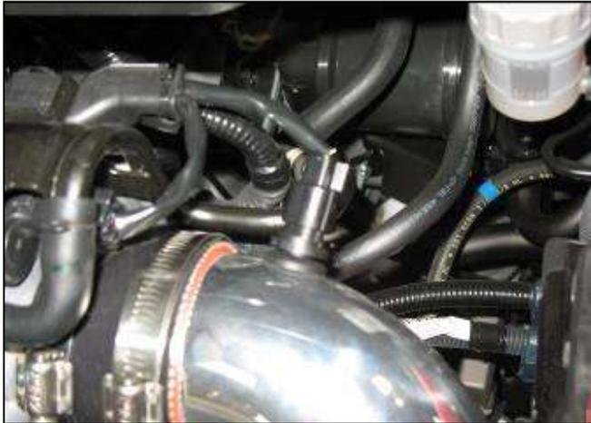
n. Plug the IAT sensor harness that was disconnected in step 2b into the installed sensor on the upper intake pipe.
