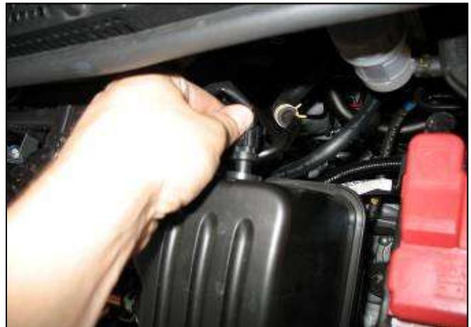
b. Unplug the Inlet Air Temperature (IAT) sensor from the wiring harness on the back side of the resonator as shown.
