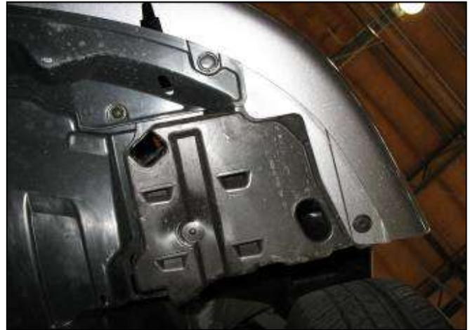
j. Remove the retaining clips and bolts securing the driver side splash shield to the bumper and chassis.
