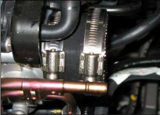
f. Install the supplied reducing coupler onto the throttle body using a #40 and a #44 hose clamp as shown.
