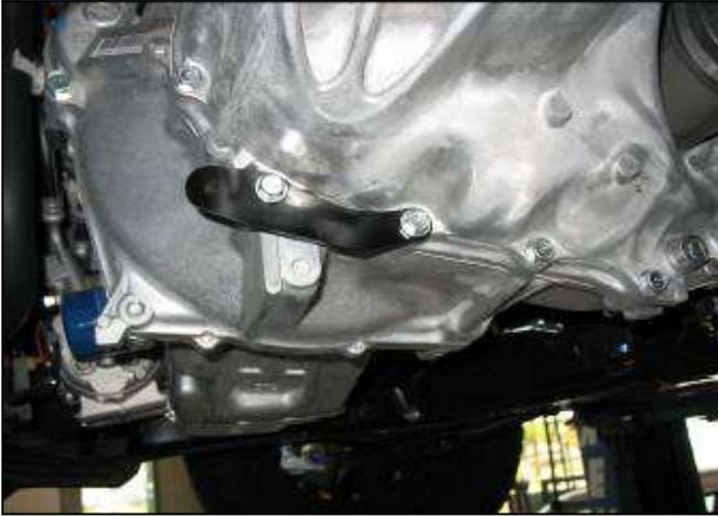
b. Install the transmission bracket using the two bolts removed in step 2q. with the third hole towards the front of the vehicle as shown. Torque bolts to 33 ft-lbs.
