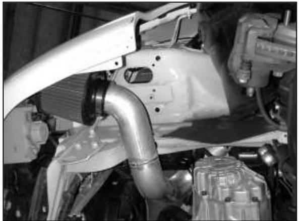
g. Install the air filter onto the intake pipe, and secure it with the supplied clamp.
