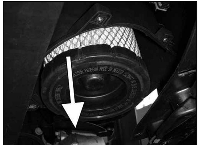
h. Pull the air filter down and out of the air filter box.
