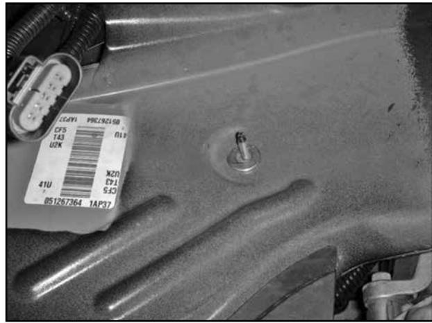
e. Place the fender washer over the rear factory air filter box mount stud.
