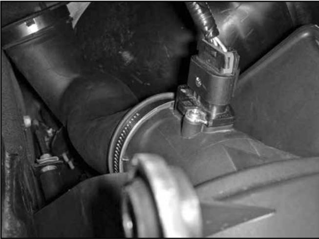
j. Reach to the top side of the air filter box and disconnect the MAF sensor harness.
