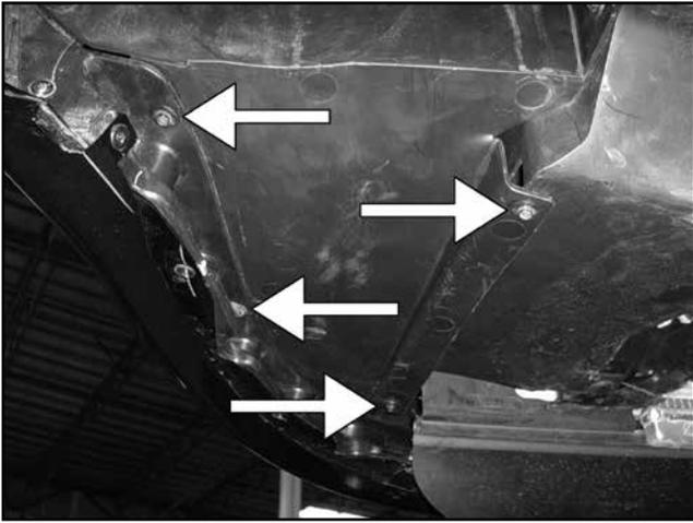
e. Remove four (4) screws holding the lower portion of the splash guard. Pull the splash guard back and out of the way.
