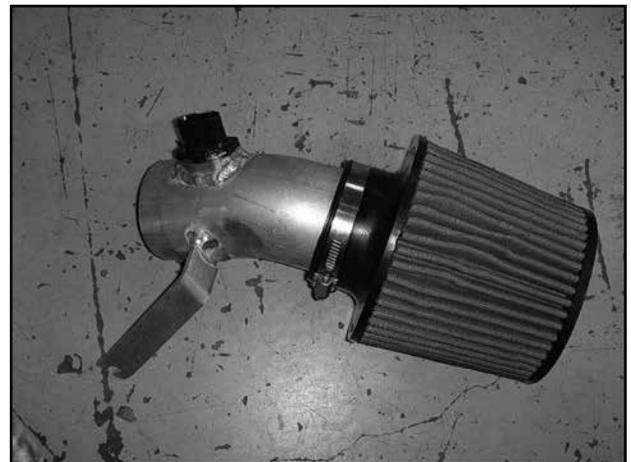
c. Install AEM® air filter onto the intake pipe as shown and secure in place.
