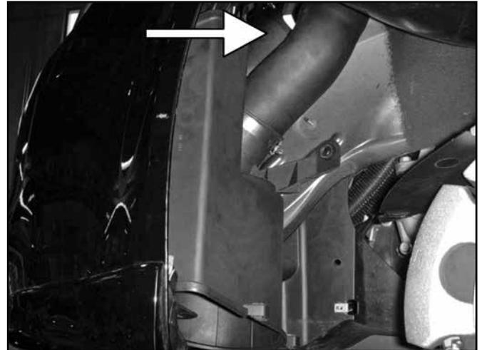
k. Remove the air filter box from the vehicle. It's helpful to guide the top hose out of the fender hole, and to pull the bumper slightly out for more clearance.
