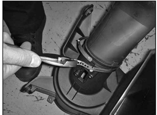
m. Using pliers, remove the stock hose clamp that is crimped onto the stock air filter box.
