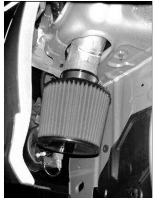
i. Install the air filter onto the end of the lower intake pipe, using the provided clamp.
