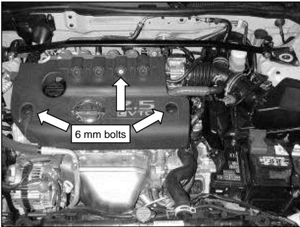
a. Loosen the three 6mm bolts on the engine cover and remove it.
