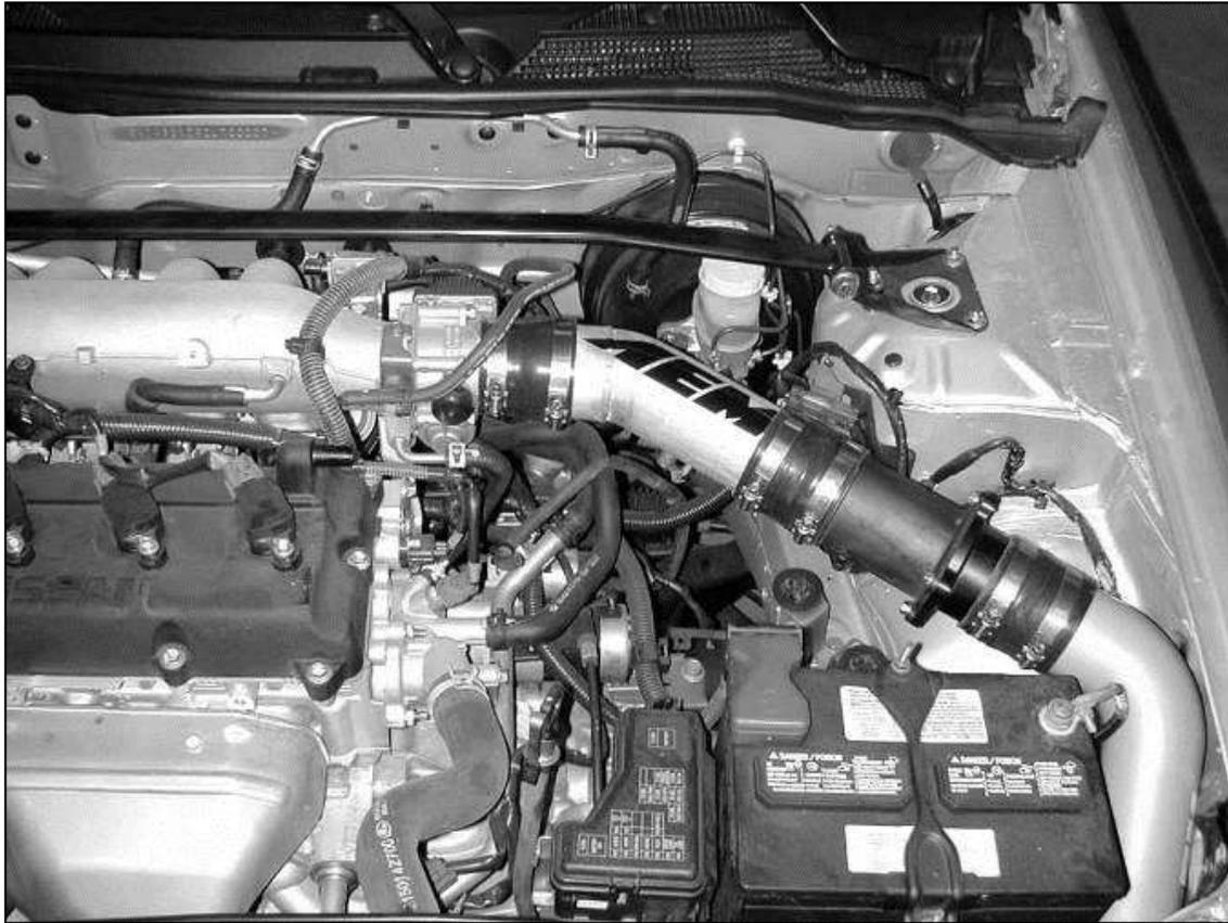
AEM® intake system installed
