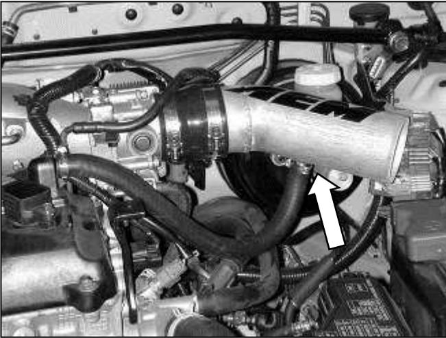
f. Using the supplied reducer coupler, #48 clamp, and a #44 clamp, attach the upper intake pipe to the throttle body as shown. Then attach the 5/8" hose to the cam cover breather and the upper pipe, using the included small clamps, as shown.
