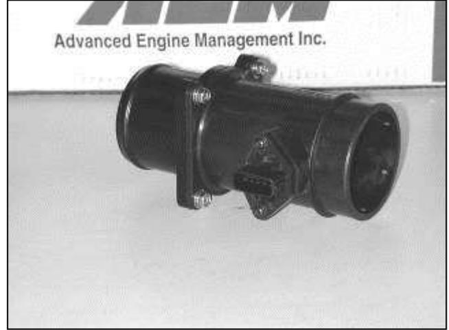
c. Install the included MAF adaptor onto the sensor using the factory bolts as shown.
