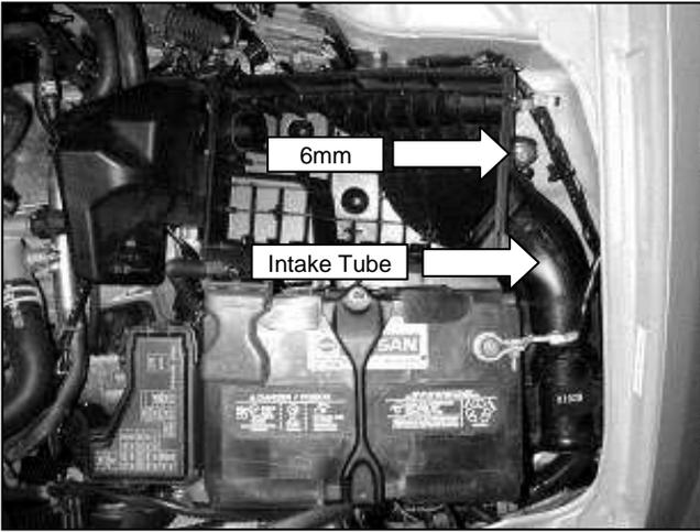
c. Loosen the 6mm air cleaner hold down bolt, remove the air cleaner assembly, and intake tube.
