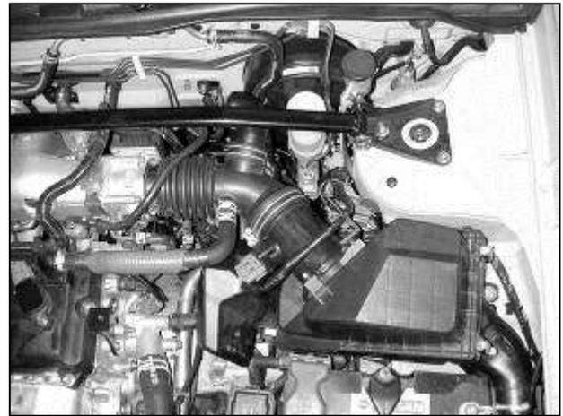
b. Loosen the air filter tube hose clamps, air cleaner lid clips, and remove the air filter lid and intake hose assembly.
