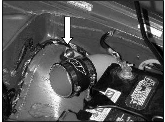
g. Install the lower intake pipe, securing the intake pipe bracket onto the rubber mount on the inner fender. Secure as shown using the included washer and nylock nut.
