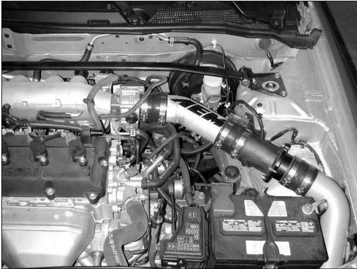
AEM® intake system installed
