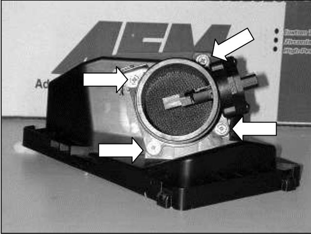
b. Loosen the four 6mm bolts, and remove the MAF Sensor from the air cleaner lid.
