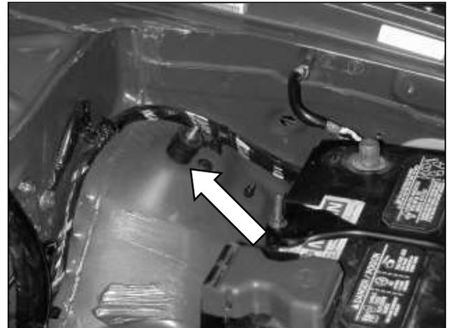
e. Install the supplied rubber mount as shown.
