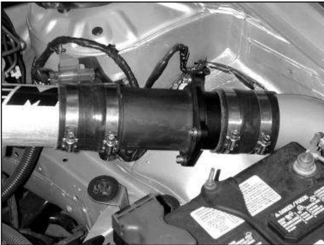
h. Insert the MAF/adaptor assembly into both the upper and lower intake pipes as shown. The adaptor end will connect to the lower intake pipe. Connect the MAF sensor plug, as shown.
