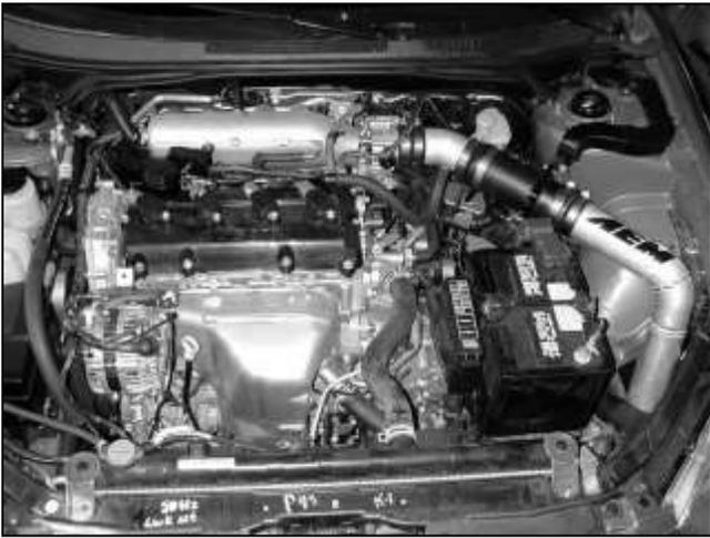
f. Install the middle intake pipe onto the MAF sensor adaptor. Loosely secure using the supplied coupler and hose clamps.
