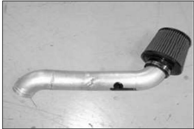
j. Install the air filter onto the end of the lower intake pipe closest to the 7/8" hole. Install the recessed plastic plug in the hole in the intake pipe.
