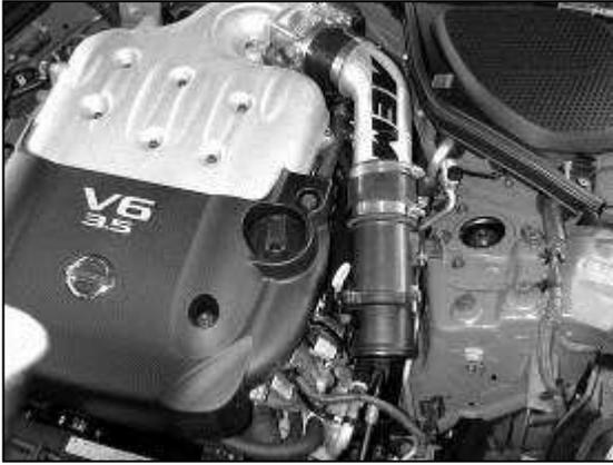
e. Place the 3" silicone coupler around the MAF sensor, not the AEM<sup>®</sup> MAF adaptor. Connect the assembly to the upper intake pipe. Use the #52 hose clamp around the throttle body and the #48 hose clamps for the 3" diameter tubing. Do not tighten the hose clamps.
