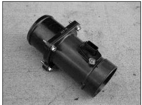
d. Using the four bolts and washers included in the kit, attach the AEM® MAF adaptor to the Nissan MAF sensor.
