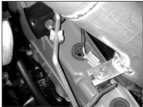
l. Line up the tab on the intake pipe with the rubber mount. Run the wheel speed sensor wire underneath intake pipe support tab. Make sure the plug and wire are not in a place where they will be pinched or damaged. Install the nut and washer according to the diagram below.
