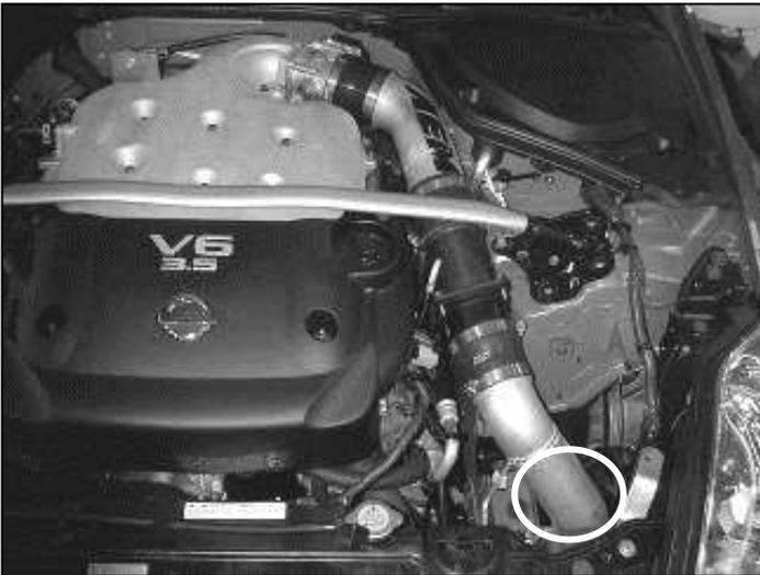
m. Position the intake pipe and air filter for the best fitment. Ensure that the intake system does not contact any part of the vehicle or any other components. **Ensure the intake pipe does not come into contact with any of the adjacent A/C hard-lines. Contact may result in failure of the A/C system and costly repairs.** After the intake system has been positioned correctly, tighten all hose clamps and the mounting tab hardware. Plug in the MAF sensor and re-install the strut-tower bar.
