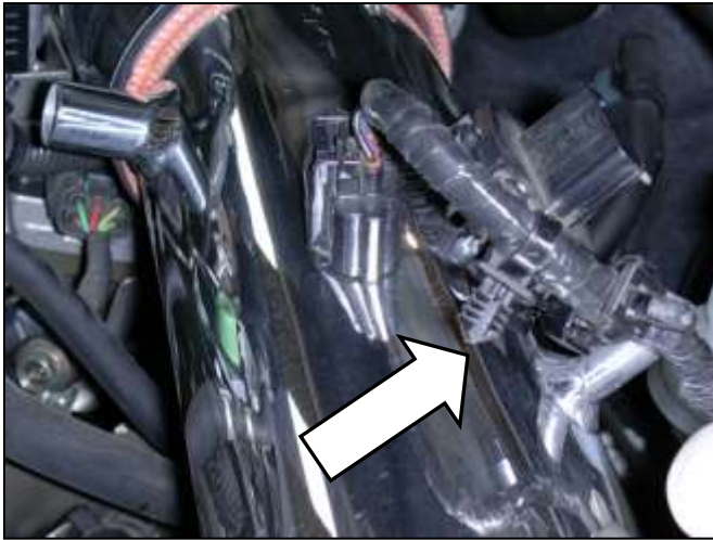
j. Attach the tree mount zip tie to the MAF sensor wiring harness. Trim the excess zip tie band.
