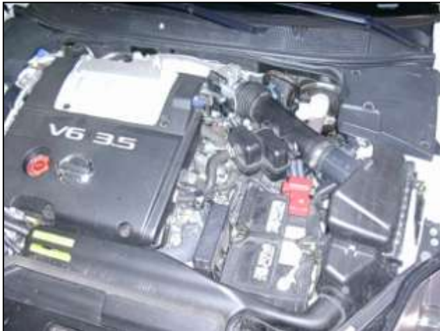
a. Stock air box system installed.
