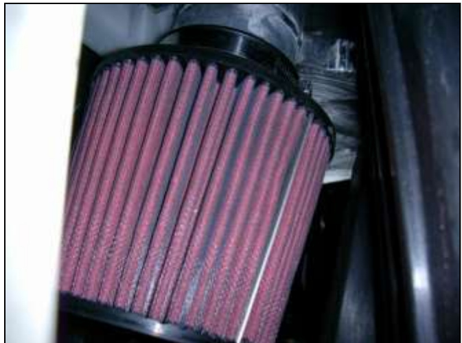
i. Place the air filter over the end of the inlet pipe. Tighten the air filter hose clamp.
