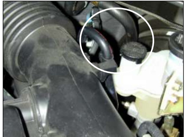
b. Free the differential breather hose from the inlet tube, if equipped. Use a supplied zip tie to secure the hose to the brake booster tube.
