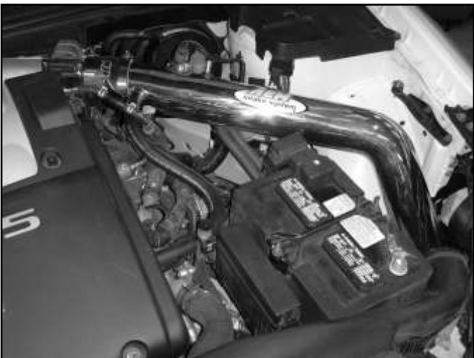
AEM® intake system installed
