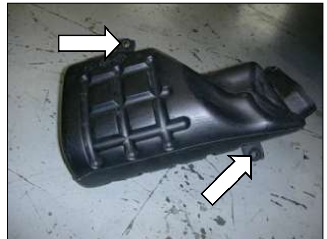
h. From inside the fender well, remove the two bolts that secure the lower air box. Then remove the lower air box from the vehicle.
