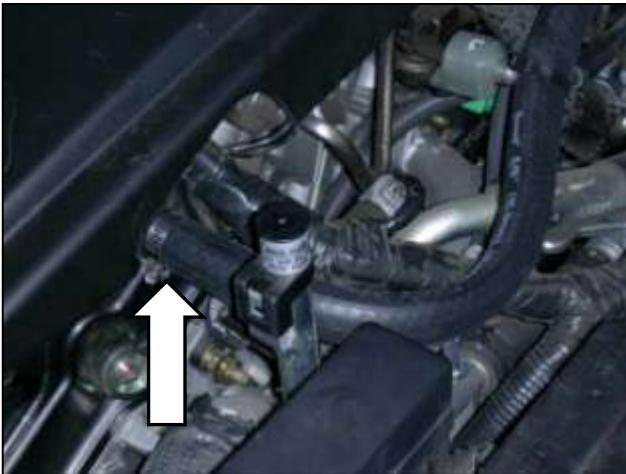
l. Secure one end of the supplied breather hose onto the valve cover with the supplied hose clamp.
