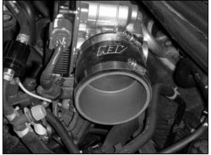
c. Slide the silicone coupler and supplied hose clamps over the throttle body.
