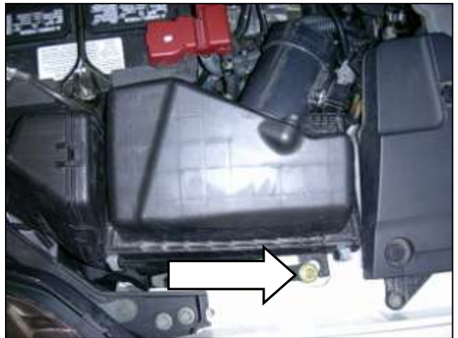
f. Removing the specified bolt and then remove the upper air box.
