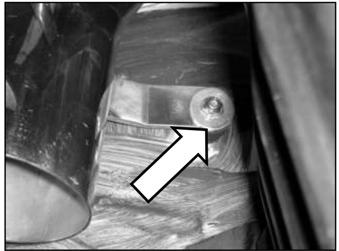
g. Place the large washer over the mounting tab. Lightly thread the lock nut over the washer.
