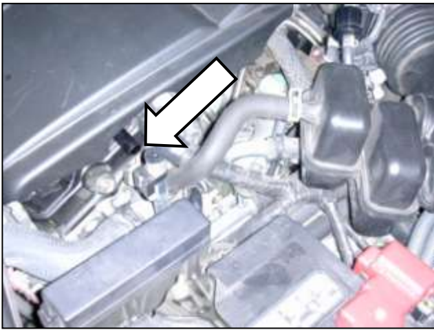
c. Pull the crankcase breather hose from the valve cover.
