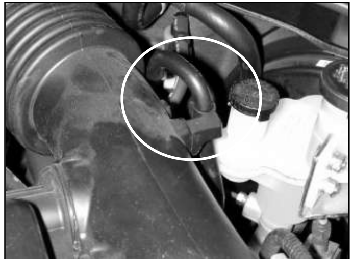
b. Free differential breather hose from inlet tube, if equipped. Use a supplied zip tie to secure the hose to the brake booster tube.
