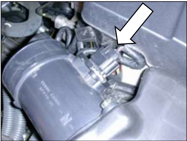
e. Free the clips that secure the mass air flow (MAF) sensor wiring harness. Unplug the MAF sensor.
