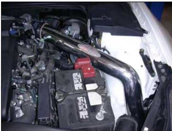
f. Place the inlet pipe in the engine bay.
