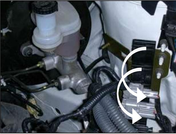
i. Unclip the two wiring harness connectors and move them two places lower.
