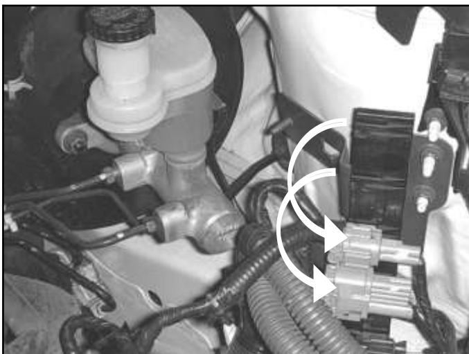
i. Unclip the two wiring harness connectors and move them two places lower.
