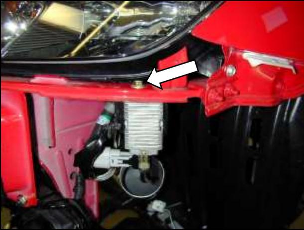
e. Remove the HID ballast bolt under the driver's side headlight.
