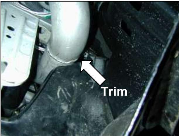
l. Trim the lower splashguard to clear the AEM<sup>®</sup> intake pipe. Hold the splashguard up to the pipe and trim only enough to clear the pipe. Re-secure the lower splashguard using the original hardware.
