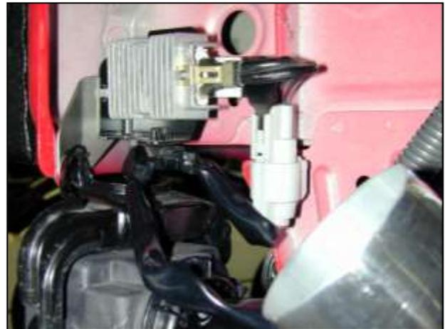
h. Install the HID ballast bracket between the fog light and the radiator support. Tighten the fog light mounting nuts.
