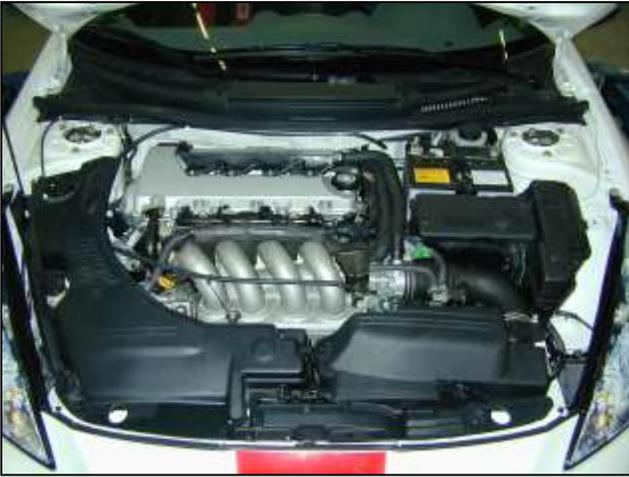
Stock air box system installed
