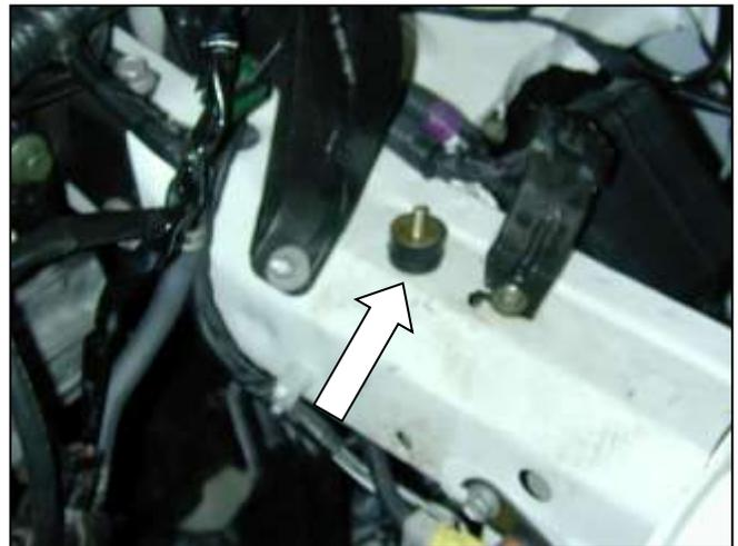
c. Thread the rubber mount into the hole where the bottom of the air cleaner case was located.
