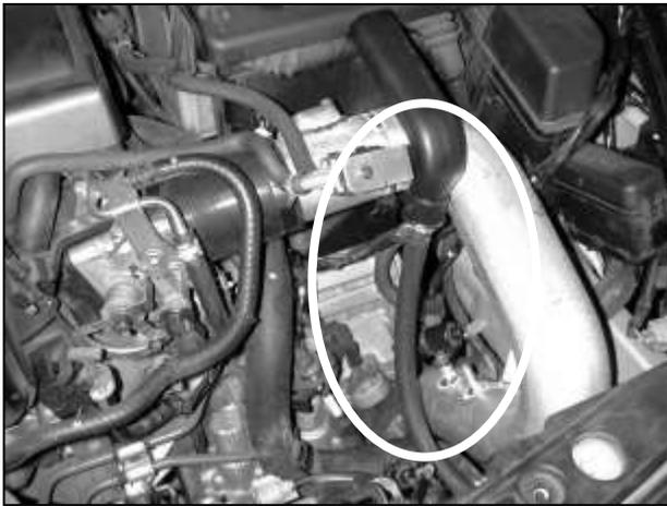
p. Install the upper ECU duct back into the factory location as shown. Attach the supplied section of 1/2" hose with one of the remaining 3/4" hose clamps. Route the hose as shown towards the bottom of the radiator fan shroud.
