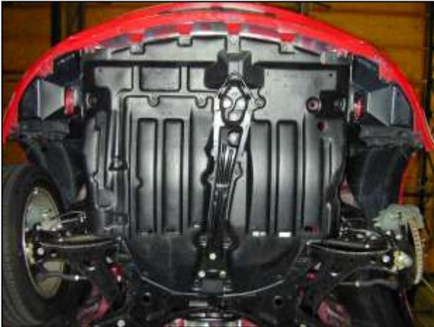
a. Remove the nuts and screws securing the underside of the front bumper.
