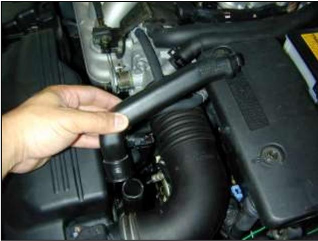
d. Remove the upper section of the ECU cooling duct. The upper piece should pull forward out of the ECU compartment; the other end will pull up off of the lower part of the duct.
