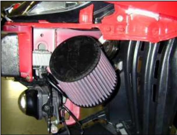
i. Install the AEM<sup>®</sup> air filter on to the end of the inlet pipe. Tighten the hose clamp. Make sure the HID ballast wires are not stretched or rubbing against any part of the car or air filter. Reinstall the front bumper cover in the reverse order of removal. Continue with installation process on step 3l.
