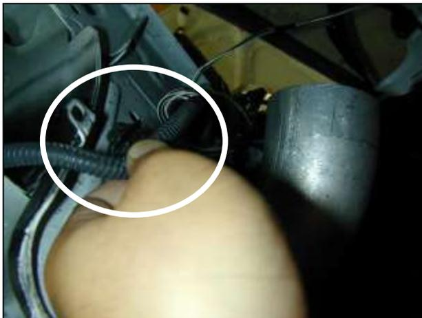
j. On some vehicles, the wire harness connected to the bumper light may interfere with air filter placement. If this occurs, remove the plastic harness clip from the bracket near the tow hook to allow more clearance.
