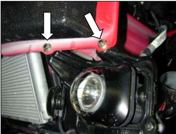
g. Remove the outer fog light nut. Loosen the inner one.
