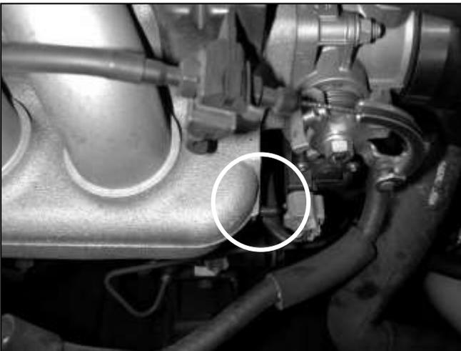
b. Install the 1/8" vacuum cap onto the vacuum port that was left exposed upon the removal of the vacuum line in step 2f.
