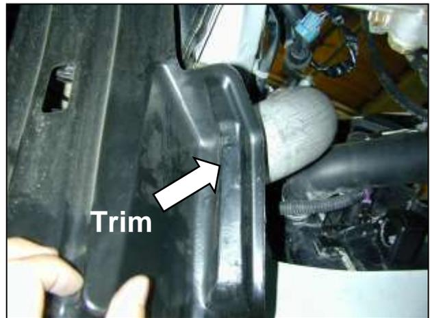
m. Trim the inner fender liner in the same manner. Re-secure the inner fender liner using the original hardware.
