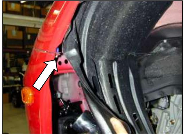
b. Remove the two screws in the upper corners of the front bumper (one on each side).
