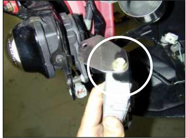
f. Attach the supplied HID ballast bracket as shown using the original bolt. The bend in the bracket should bend towards the HID ballast.
