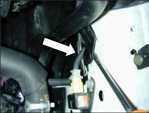
h. Pry the plastic rivet that secures the lower ECU cooling duct away from the engine bay. Pull the lower part of the duct out of the radiator fan shroud. Remove the entire lower ECU cooling duct from the engine bay.
