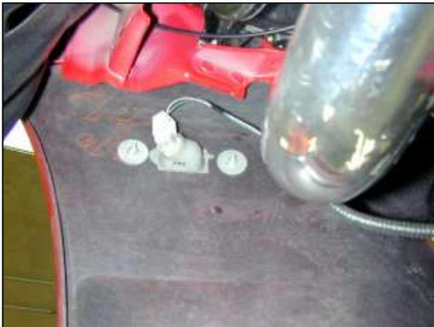
c. Unplug the bumper lights from inside the bumper (one on each side).
