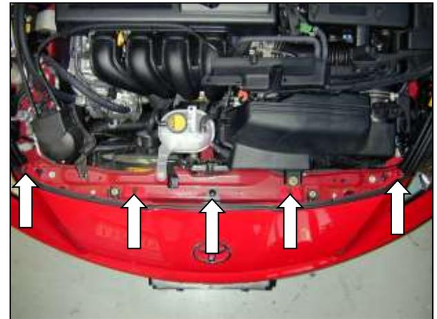
d. Remove the four bolts and one plastic rivet securing the front bumper to the upper radiator support. Remove the front bumper cover carefully, making sure all bolts have been removed and necessary wires unplugged.
