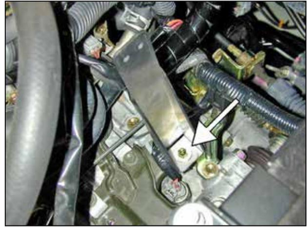
q. Install the VSV mounting bracket using one of the factory air box bolts as shown.
