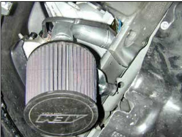
h. Install the AEM® air filter onto the end of the intake pipe.
