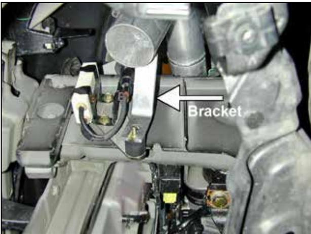
f. Install the AEM® intake pipe from underneath the vehicle. Insert the end near the MAF sensor into the coupler on the throttle body. The mounting bracket on the intake pipe should line up with the rubber mount installed in step 3d.
