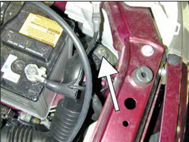
g. Remove the bolt retaining the lower intake air duct. This bolt and duct are located between the radiator support and the battery. Remove the lower air cleaner housing and lower intake air duct from the engine bay.
