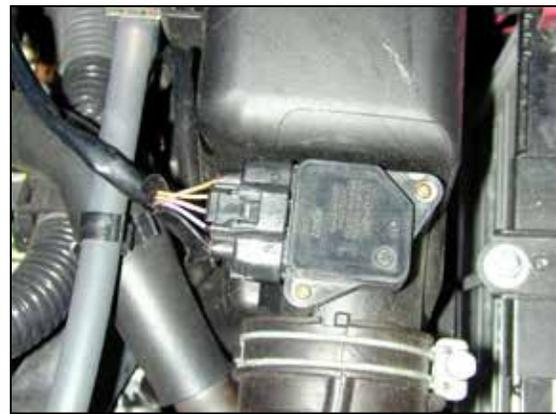
b. Disconnect the wire harness connected to the mass-air flow (MAF) sensor.
