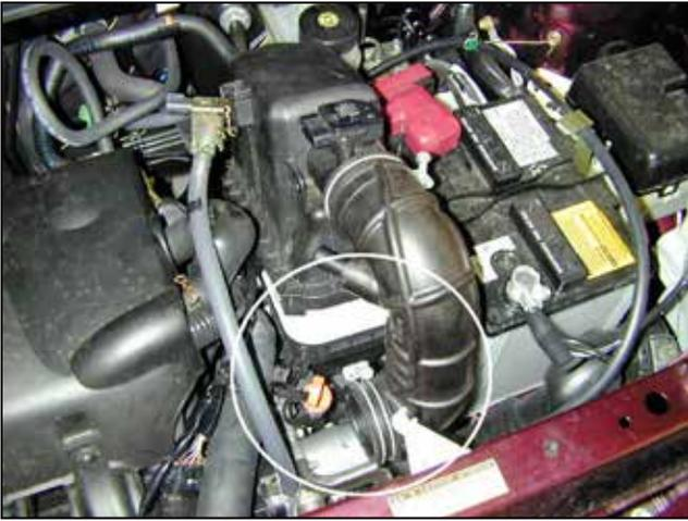
e. Loosen the hose clamp at the throttle body. Release the two spring clips at the front edge of the air cleaner cover. Remove the air cleaner cover, intake tube, and MAF sensor from the engine compartment.
