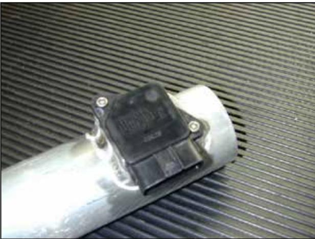
b. Install the MAF sensor into the AEM® intake pipe. Use the supplied 8-32 cap head screws. Use care to avoid damaging the o-ring.
