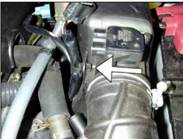
c. Release the wire harness from the air cleaner cover by squeezing the plastic clip from the top and bottom. Carefully remove the plastic clip to allow the MAF and VSV connector harnesses to be routed separately. Remove the breather hose from the vehicle by squeezing the spring clamps on both the intake tube and at the valve cover. Save the spring clamps for use later in the installation.
