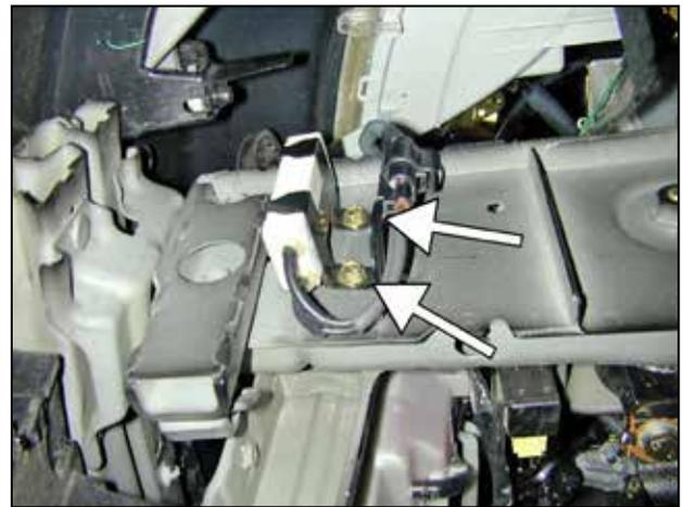
c. Remove the two bolts securing the resistor ballast beneath the driver's side headlight.
