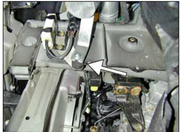
g. Loosely secure the mounting bracket with the remaining fender washer and lock nut. Refer to the diagram below for proper rubber mount installation.
