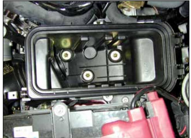
f. Loosen the three bolts that retain the lower air cleaner housing in the engine bay.
