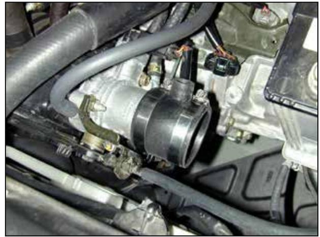
e. Loosely install the coupler onto the throttle body using the two #36 hose clamps. Orient the nipple so that it is pointed approximately 45° back towards the firewall. This will be adjusted later in the installation.
