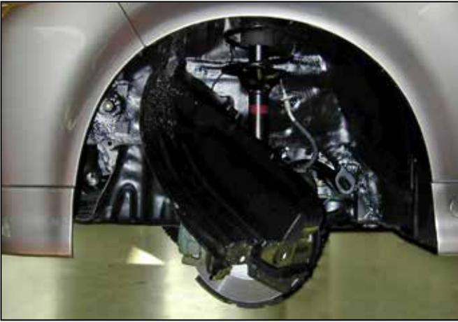
i. Raise the front of the vehicle with a jack. Refer to your owner's manual for proper jack and jack stand placement to properly support vehicle. Support your vehicle using properly rated jack stands before wheel removal or while working under the vehicle. **NEVER WORK UNDER A VEHICLE WITHOUT USING JACK STANDS.** Remove the bolts and plastic rivets that secure the fender liner. Pull the fender liner back to gain access to the area behind the front bumper.
