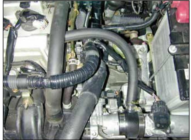
l. Install the supplied vacuum nipple into the throttle body coupler. Secure the nipple with the supplied hose clamp.
