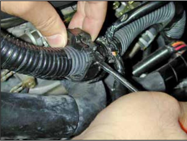
p. Place a small screwdriver in the slot of the clip and gently pry downwards. Split the housing of the clip open. Slide the clip down the wire harness a couple of convolutions to free up more harness towards the MAF sensor. Repeat for the second wire harness clip. Reinstall both clips to the bracket on the engine. Plug in the MAF sensor wire harness and make sure the wires are not stretched.
