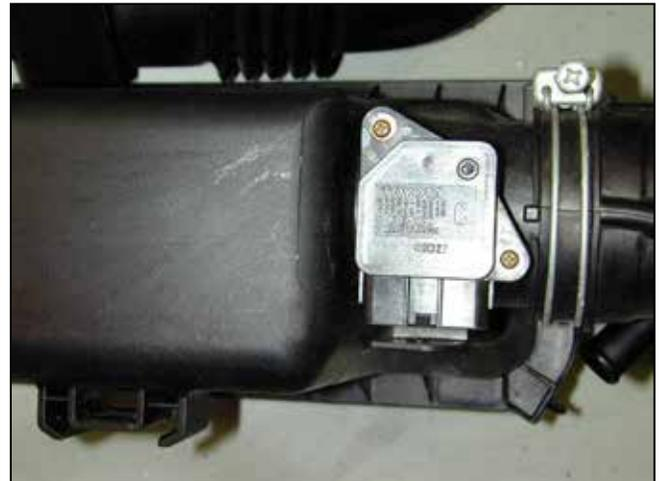
h. Remove the MAF sensor by loosening the two Phillips head screws. Save the screws for use if the vehicle is ever returned to stock condition. Handle the MAF sensor with care to avoid damage.
