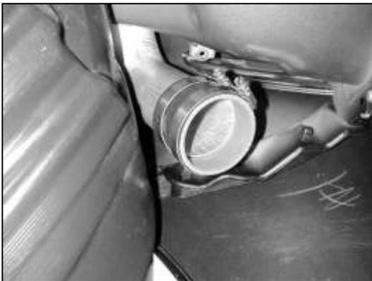
j. Attach the supplied coupler to the lower end of the upper intake pipe (located in the fender well). Loosely secure two of the provided hose clamps onto the coupler.
