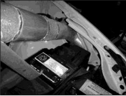
d. Insert the 90 degree bend of the upper intake pipe (the long one) into the fender from the engine bay.
