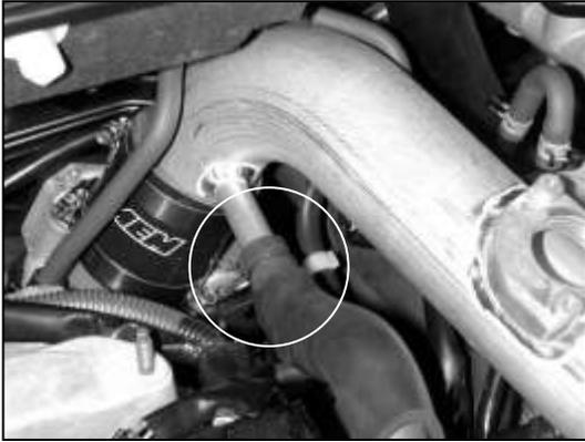
h. Connect the breather hose to the upper intake pipe's nipple.
