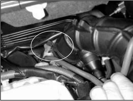
g. Squeeze the spring clamp securing the inlet tube to the throttle body. Remove the inlet tube and upper airbox as one assembly.
