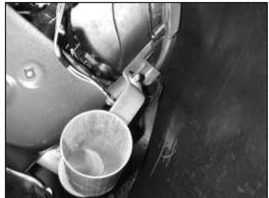
k. Install the lower intake pipe into the coupler. The bracket will line up with the rubber mount installed in step 3i. Loosely secure the bracket to the rubber mount with a washer and locknut.
