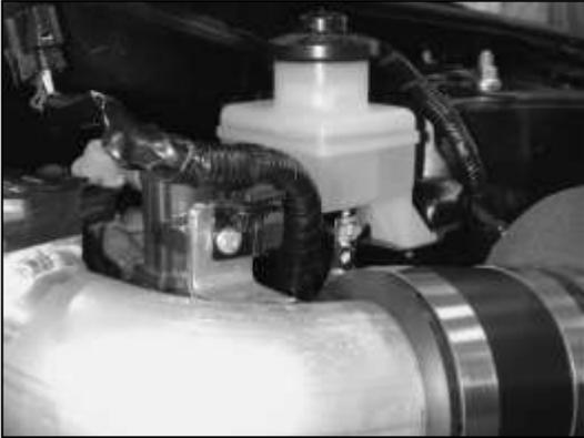
n. Plug in the MAF sensor wire harness connector back into the MAF sensor. Mount the EVAP VSV to the bracket on the upper intake pipe using the supplied M5 screw and washer. Insert the screw through the wire harness clip and through the intake pipe bracket so it threads into the VSV. Adjust the wires so that they are not in tension.
