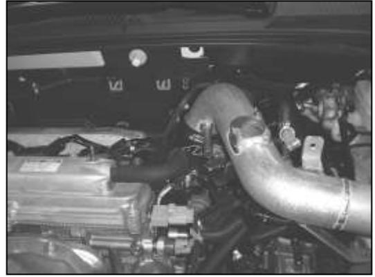
e. Install the upper intake pipe into the coupler on the throttle body. Leave the hose clamps loose for adjustment.
