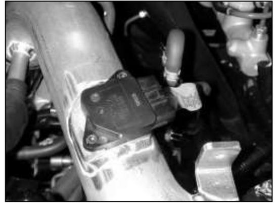
m. Secure the MAF sensor to the AEM® intake pipe with the supplied 8-32 bolts. Use care to avoid damaging the o-ring.
