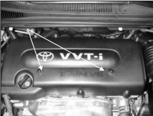
a. Remove the two nuts securing the plastic engine cover to the valve cover. Remove the plastic engine cover from the vehicle.
