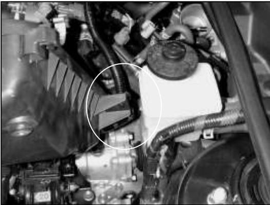
i. Free the wire harness loom clip by gently squeezing the sides in. Remove the lower airbox from the engine bay.
