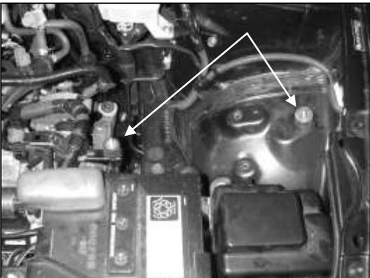
b. Install two of the supplied rubber mounts into the threaded holes as shown in the image.
