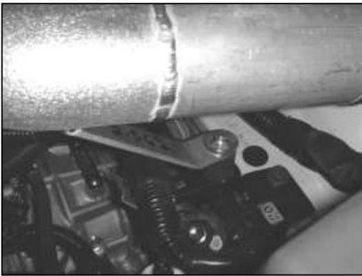
f. The pipe's bracket will line up with one of the rubber mounts installed in step 3b. Loosely secure the bracket to the rubber mount with a washer and nut.
