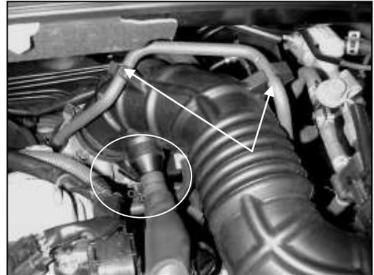
b. Pull the EVAP purge hose free from the two rubber clips on the intake hose. Remove the crankcase breather hose from the intake tube. Save the factory clamp for use later in the installation.
