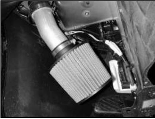
l. Install the AEM® air filter onto the end of the lower intake pipe. Once proper fitment is achieved, secure the air filter to the lower intake pipe with a supplied hose clamp.
