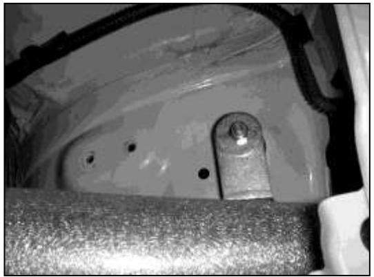
g. Loosely secure the second bracket to the rubber mount with a washer and nut.
