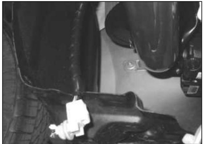
d. Disconnect the side marker lamp. Wrap the wires with the supplied helical wrap, then re-connect the side marker lamp.
