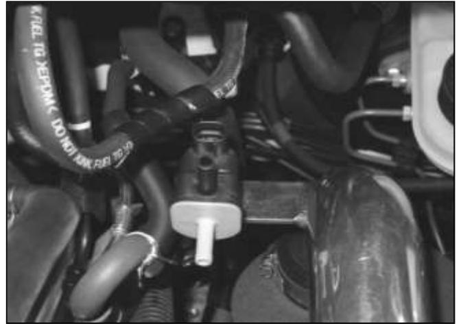
i. Attach the VSV to the bracket on the intake pipe using the supplied bolt and washer. Wrap the fuel line with helical wrap as shown.
