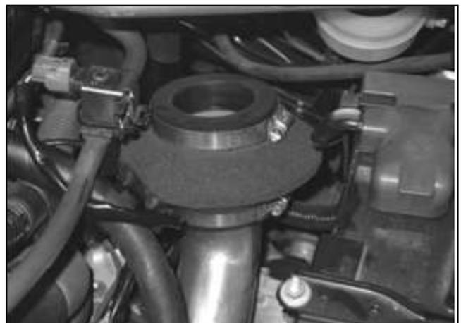
f. Install the air bypass valve on the lower intake pipe.
