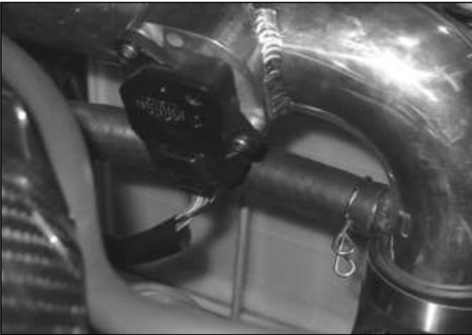
h. Attach the MAF sensor connector to the sensor installed in the intake pipe. Install the supplied hose between the valve cover and the breather nipple on the intake pipe using the factory clamps.
