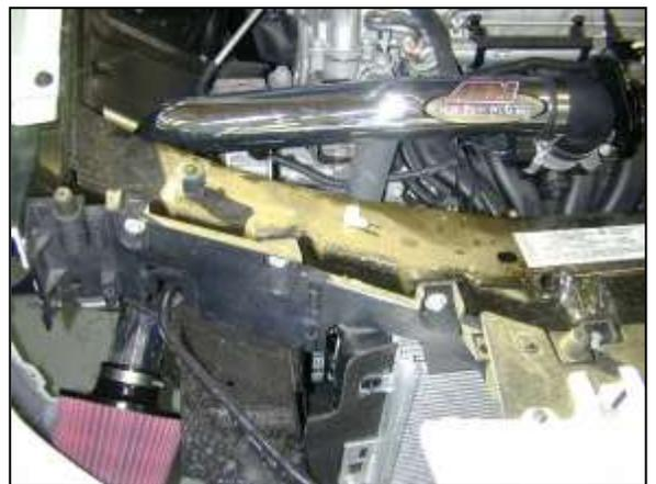
AEM<sup>®</sup> intake system installed
