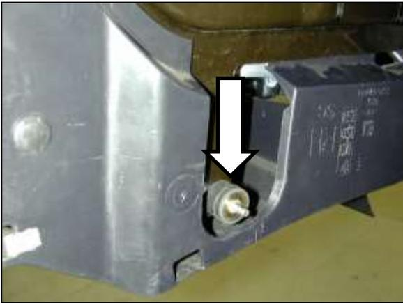
b. Install the 5/8" rubber mount to the lower mounting tab as shown. Secure it with a supplied washer and lock nut.
