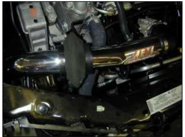
q. If an AEM<sup>®</sup> bypass valve is installed, install the bypass valve as shown. The intake pipe will require some modification to accommodate the AEM bypass valve. Follow the instructions included with the bypass valve for proper installation.
