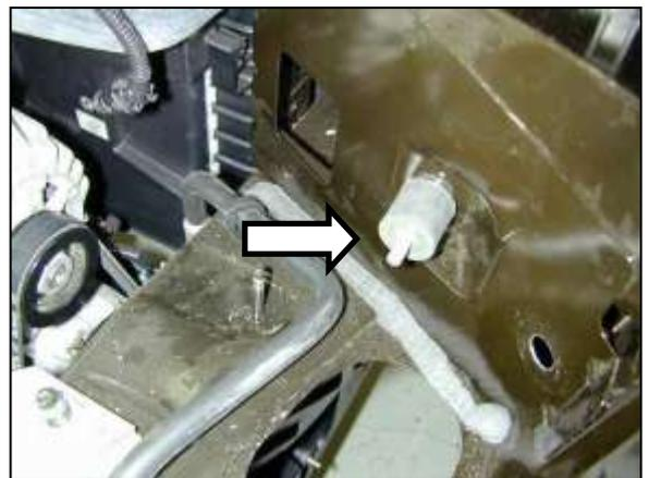
g. Install the 1" rubber mount from inside the engine bay, as shown.
