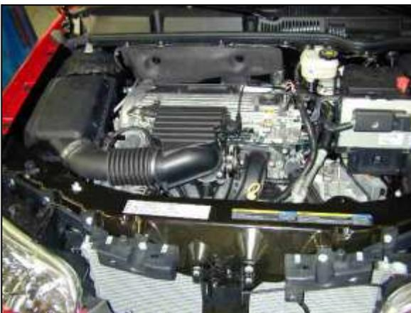
Factory air box system installed.
