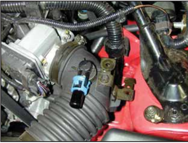
e. Unscrew the Inlet tube from the throttle body and the air filter housing. Remove the inlet tube.
