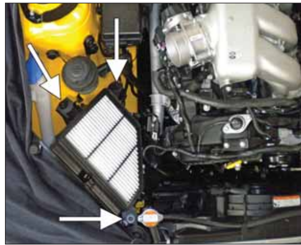
d. Unclip the MAF sensor harness from the lower half of the airbox. Remove the three M6 bolts securing the lower airbox, and remove the lower airbox.
