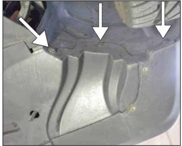
f. Raise the front of the vehicle with a jack. Refer to your owner's manual for proper jack and jack stand placement to properly support vehicle. Support your vehicle using properly rated jack stands before wheel removal or while working under the vehicle. **NEVER WORK UNDER A VEHICLE WITHOUT USING JACK STANDS.** In the wheel well area on each side, remove the 3 clips securing the belly pan.
