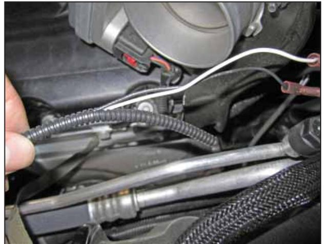
i. Slip the protective convoluted split-loom wire cover over the newly extended IAT wire harness. Trim as needed.
