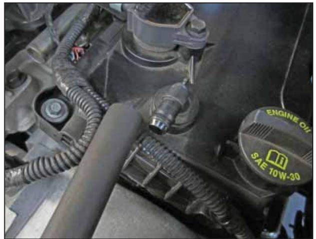
b. Pull to remove the crank case breather hose from the nipple on the head cover.
