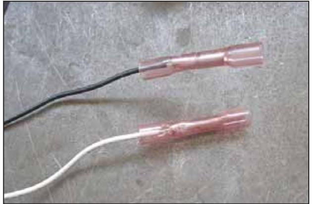
e. Crimp a Perma-Seal connector onto one end of the provided 20ga. black extension wire. Crimp another Perma-Seal connector onto one end of the provided 20ga. white extension wire as shown.
