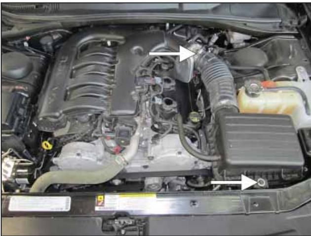
a. Remove the bolt securing the OEM air box and loosen the hose clamp at the throttle body.
