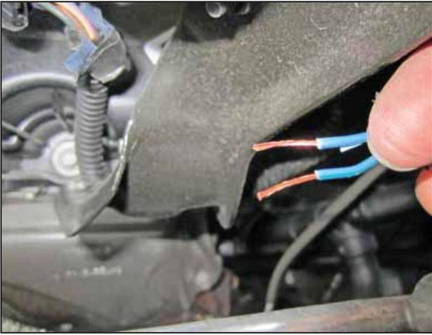
f. Strip the ends of the cut IAT wires near the throttle body.
