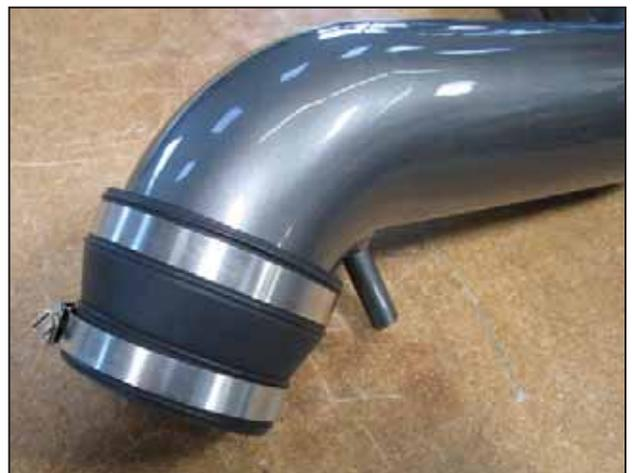
k. At the top end of the upper intake tube, install the reducer coupler, one #56 clamp and one smaller #48 hose clamp. Loosely tighten the hose clamps.
