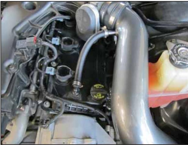
p. Install the supplied 1/2" ID hose between the crank case vent on the head cover and the nipple on the upper intake pipe using the provided small hose clamps. Trim the hose if needed.
