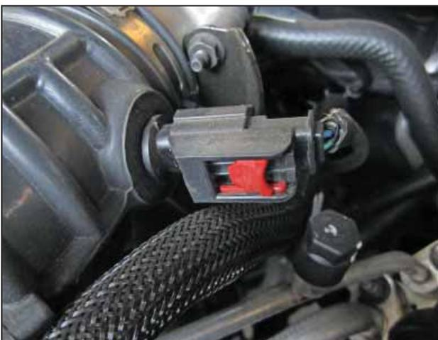
c. Unplug the IAT sensor. To unplug the IAT sensor, slide the red tab back to unlock the latch on the plug, then press in on the latch and pull the plug off of the sensor.
