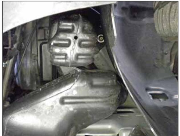
h. Locate and remove the 10mm bolt securing the lower intake resonator to the vehicle. Remove the resonator.
