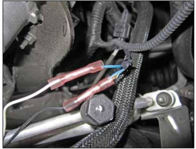
g. Crimp the stripped stock wires into the new Perma-Seal connectors on the black and white wires. Since the color of the stock wires may vary with each vehicle, pay close attention and crimp the other ends of the new black and white wires to the correct color wires on the IAT connector.
