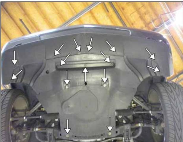
r. Reinstall the belly pan and hardware (3 clips, 7 screws, and 2 bolts) that were removed in step 2g. Also install the 3 clips for each wheel well area that were removed in step 2f.
