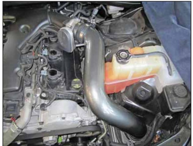
o. The lower end of the upper intake pipe should be inserted into the lower rubber coupler to a depth of about  $\frac{3}{4}$ " to 1". Use glass cleaner as a lubricant if needed. To allow fitment of the reducer coupler over the throttle body, slide the lower end further into the elbow coupler, then adjust the top end of the intake tube to fit over the throttle body. When a proper fit is achieved, pull up on the lower end of the tube to adjust the fit, and then tighten the 3 hose clamps.
