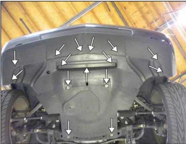
g. From underneath the vehicle, remove the following: 3 clips, 7 screws, and 2 bolts from the front belly pan. Remove the front belly pan.
