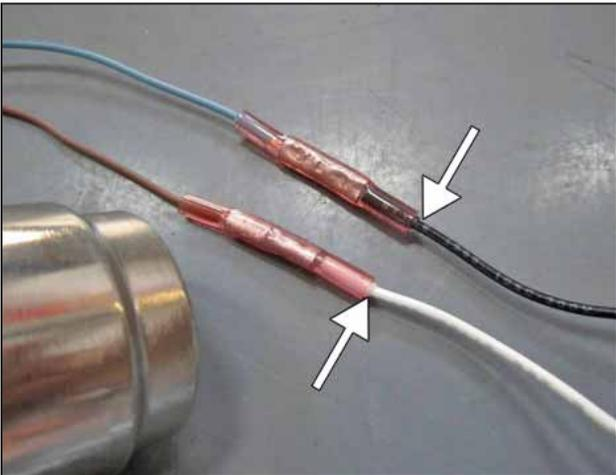
h. Using a heat gun or other safe heat source, heat shrink each of the Perma-Seal connectors until clear sealant comes out of both ends of the connector.
