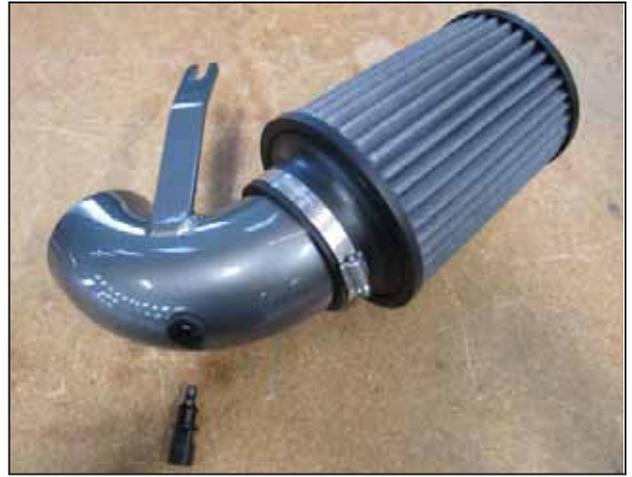
g. Install the grommet into the lower pipe. Attach the air filter with one #56 clamp as shown.
