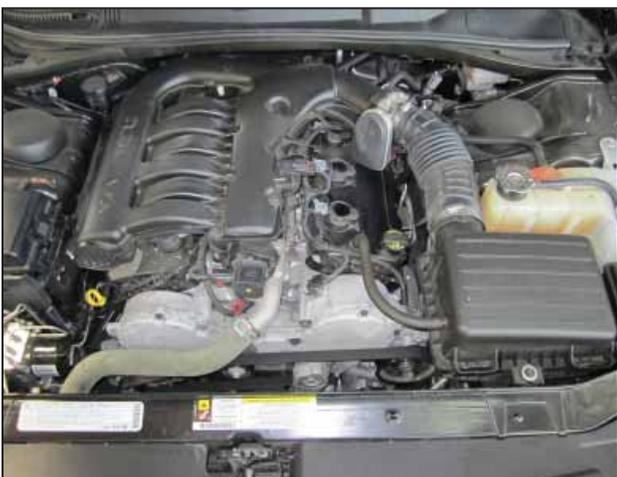
Stock air box system installed
