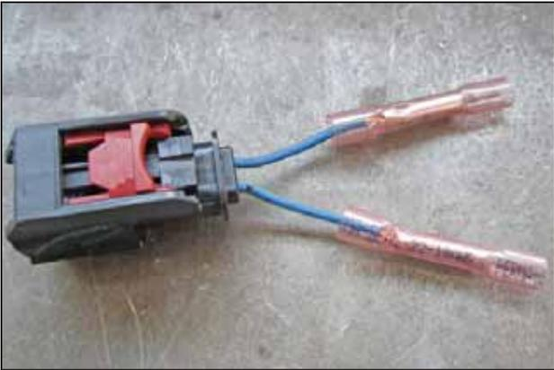
d. Crimp on two Perma-Seal connectors as shown.
