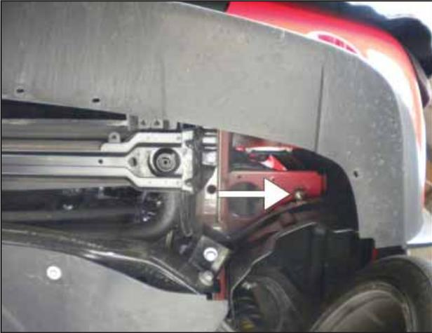
b. From underneath the vehicle, install the M8 rubber mount through the slotted hole in the sheet metal using one M8 washer and M8 nut. In order to leave some room for adjustment, do not fully tighten the M8 rubber mount.
