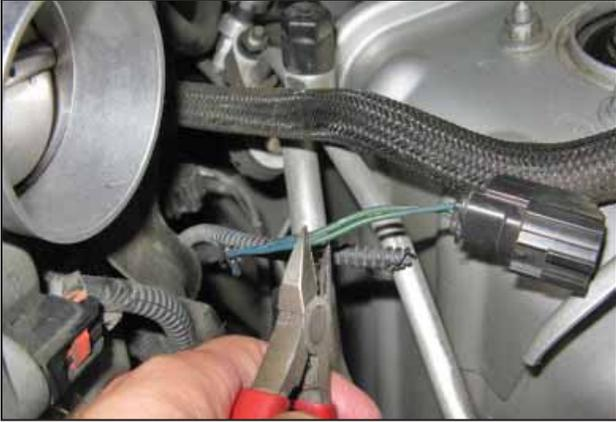
b. Slit open the insulation cover at the end of the IAT connector cable to expose the 2 wires. Cut the wires 1-2 inches [5 cm] below the connector.
