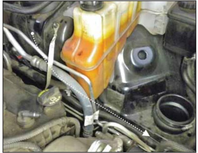
m. Route the new IAT extension harness underneath the existing OEM factory harness as shown. Use the 2 supplied zip ties to secure the extension harness and route the female connector down below to the lower intake tube.
