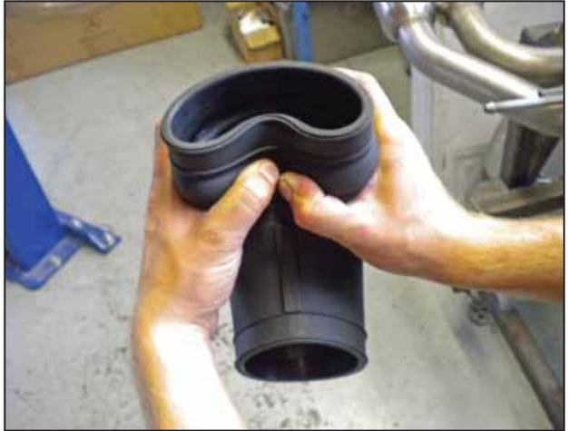
c. Hold the rubber coupler as shown, and squeeze the hump end of the coupler to collapse it into itself.
