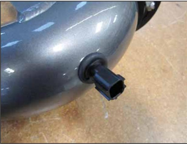
h. Carefully install the IAT sensor into the grommet.
