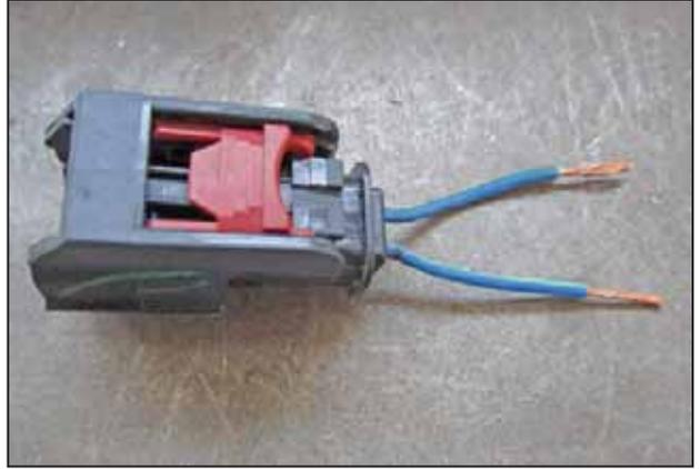
c. Strip the ends of the wires at the connector.
