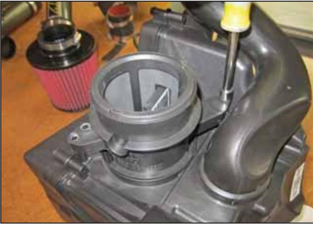
k. Remove the two 8mm bolts that secure the MAF sensor to the air box.
