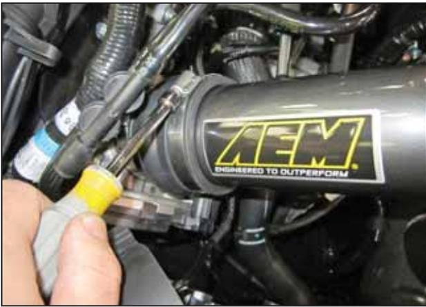
f. Tighten the #44 hose clamp (9444) on the hump hose on the intake pipe side.
