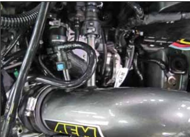
d. Align the intake pipe and connect the both PCV hoses as shown.
