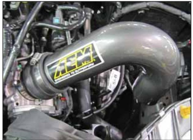
c. Install the upper intake tube (2-1478) as shown.
