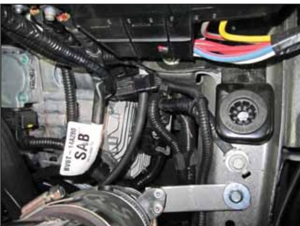
v. Secure the MAF sensor extension harness with the two provided zip ties (1-113) to prevent the wiring harness from moving around.
