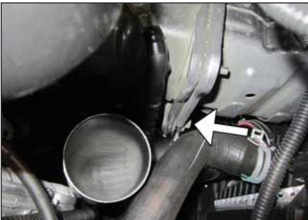
j. Mount the intake bracket onto the stud where the 13mm nut was loosened in step 3g. Hand tighten the 13mm nut to sandwich the intake tube's bracket between the chassis the 13mm nut.
