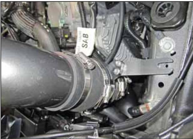
n. Orient the MAF sensor assembly as shown and attach to the upper and middle intake tubes.
