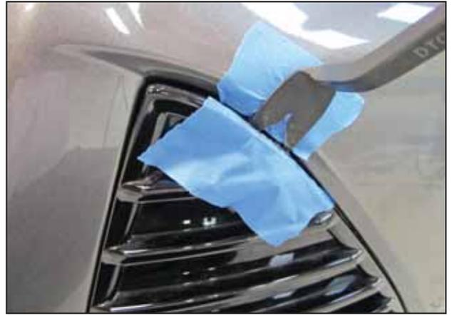
l. Use a panel popper or flat screw driver to remove the front cover on the bumper. Place the tool in between the bumper and cover. Use a towel or some masking tape on the bumper and cover to prevent scratches.
