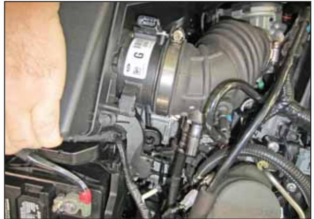
h. The air box is mounted to 3 rubber grommets, pull the air box up and out to dislodge the air box from the grommets.
