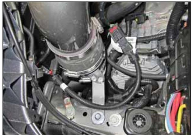
u. Connect the MAF sensor extension harness (21780) to the MAF sensor and engine wiring harness as shown.
