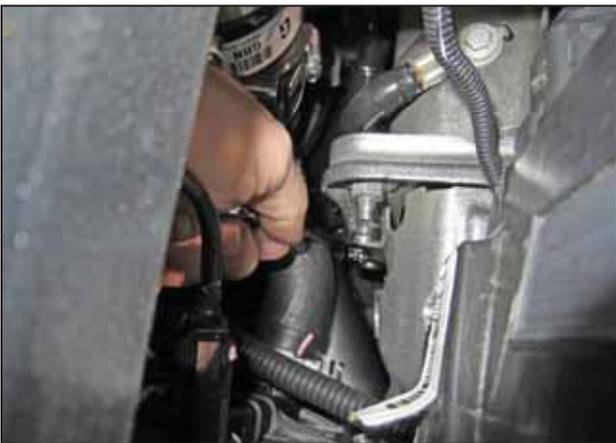
t. Reach down into the engine bay and use a box wrench to tighten the 13mm chassis nut to secure the middle intake tube.
