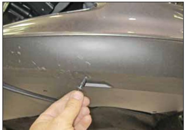
p. Remove the plastic clip securing the fender liner to the lower front side of the bumper.
