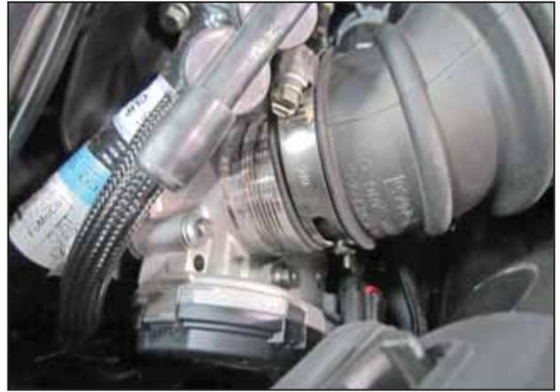
f. Pull the intake tube off of the throttle body.
