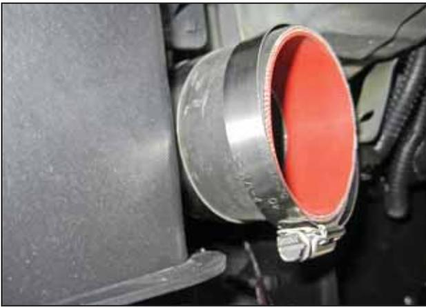
p. Slide a #40 hose clamp (9440) onto the middle intake tube's lower coupler.
