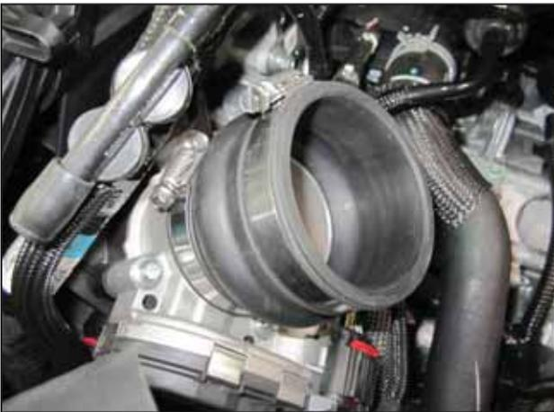
b. Install the hump hose with a #40 hose clamp (9440) on the throttle body side and a #44 hose clamp (9444) on the intake tube side.
