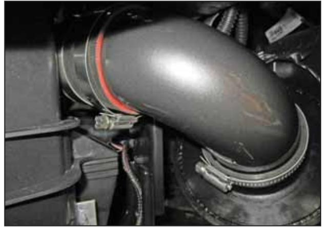
s. Attach the lower intake tube to the middle intake tube coupler. Orient the intake tubes and air filter and ensure the entire assembly has adequate clearance.
