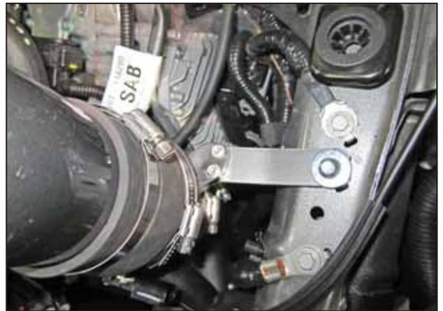
o. Secure the bracket attached to the MAF sensor housing to the vehicle's frame using the provided 10mm bolt (1-2038) and washer (08160).
