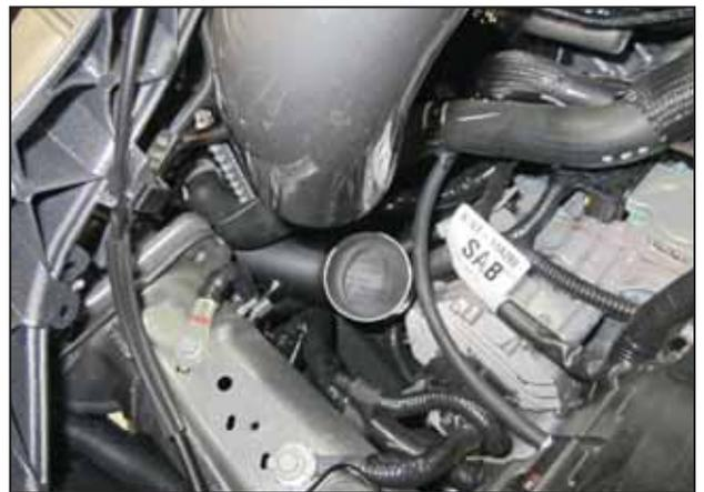
i. Guide the middle intake tube down into the engine bay so the end with the coupler is positioned on the lower end.
