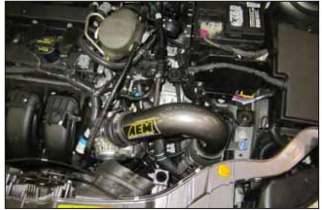
AEM® intake system installed
