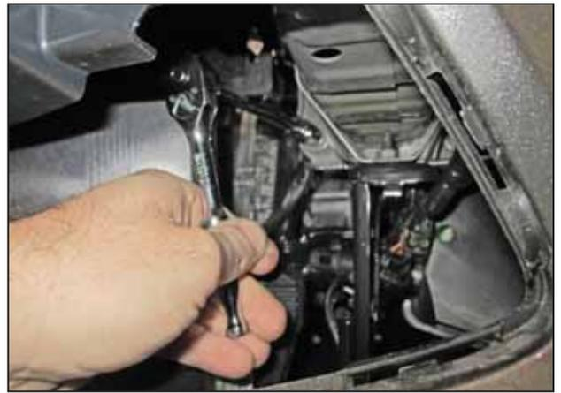
g. Through the opening exposed from the bumper cover removed in step 2m, loosen the 13mm nut on the chassis.
