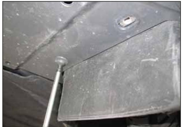
n. From under the car remove the 2 T25 Torx screws.
