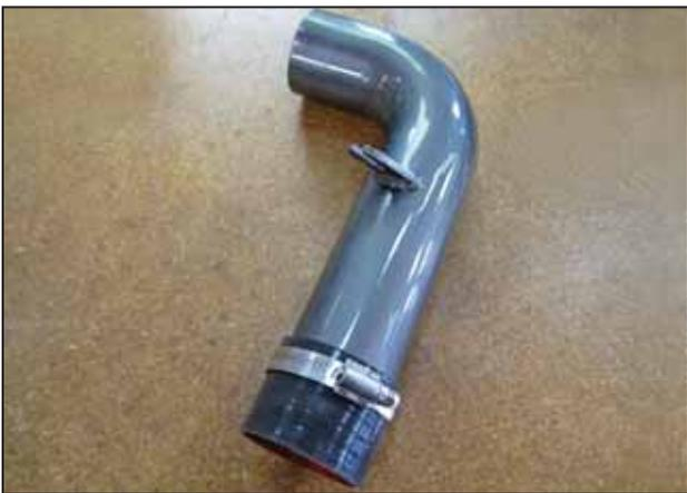
h. Install the coupler (5-250) onto the middle intake tube (2-1479) and secure with a #40 hose clamp (9440).
