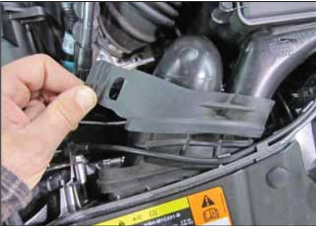
g. Unfasten the rubber air inlet strap securing the air box to the front of the vehicle.
