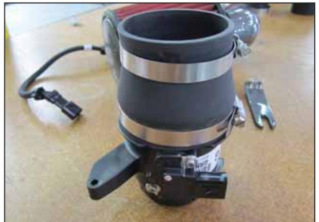
k. Install the 2.75" to 3.25" coupler (5-328) onto the MAF sensor. Slide a #44 hose clamp (9444) and a #52 hose clamp (9452) onto the coupler as shown.
