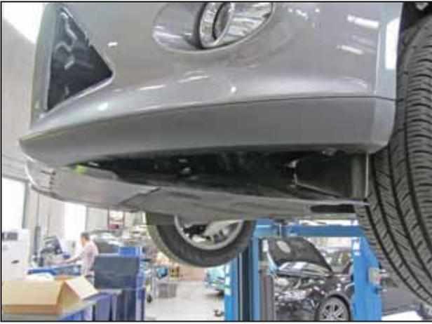
q. Pull down the corner of the belly pan to gain access to the inner bumper cavity.
