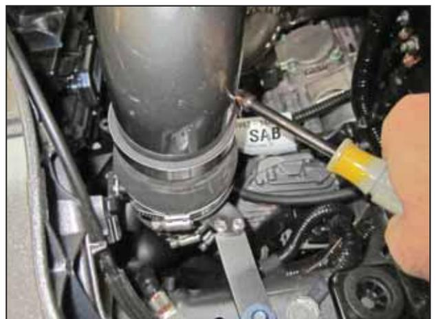
w. Ensure all hose clamps are tightened and secure.
