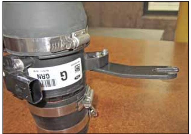
m. Mount and secure the bracket (32-3084) to the MAF sensor housing using the provided socket head bolts (1-2103) and 4mm washers (08278). Tighten the socket head bolts using a 2.5MM allen wrench.
