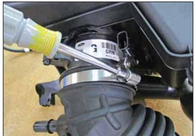
j. Loosen the hose clamp securing the intake tube to the MAF sensor. Remove the intake tube from the airbox assembly.
