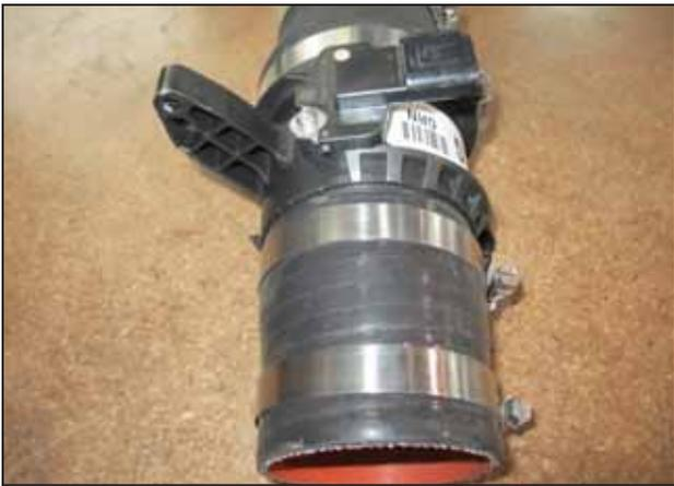
l. Install the 2.75" to 2.5" coupler (5-257) onto the bottom side of the MAF sensor. Slide a #44 hose clamp (9444) and a #40 hose clamp (9440) onto the coupler as shown.
