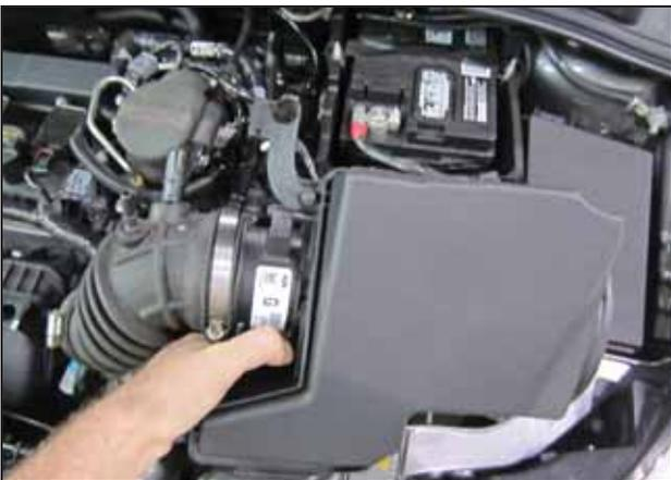
i. Remove the air box assembly from the vehicle.
