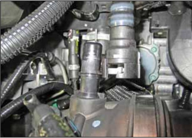
e. Locate PCV hose #2 (Grey Locking Mechanism) and disconnect from the intake tube.
