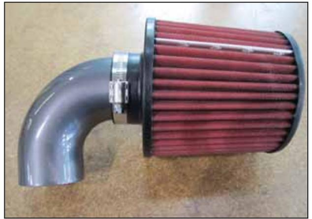
q. Attach the AEM® air filter (21-2011DK) onto the lower intake tube (2-1480) using a #44 hose clamp (9444).
