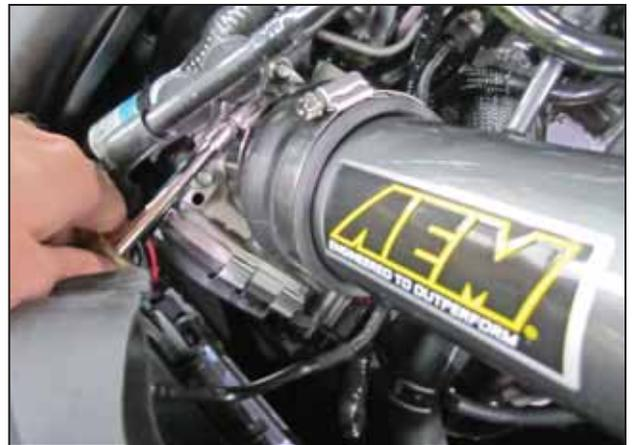
e. Tighten the #40 hose clamp (9440) on the throttle body side of the hump hose.
