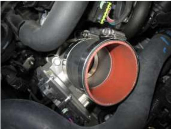
A. Install two #48 hose clamps (F) onto the silicone hose (E), then install the hose over the throttle body flange. Tighten the hose clamp over the throttle body flange and leave the other clamp loose.
