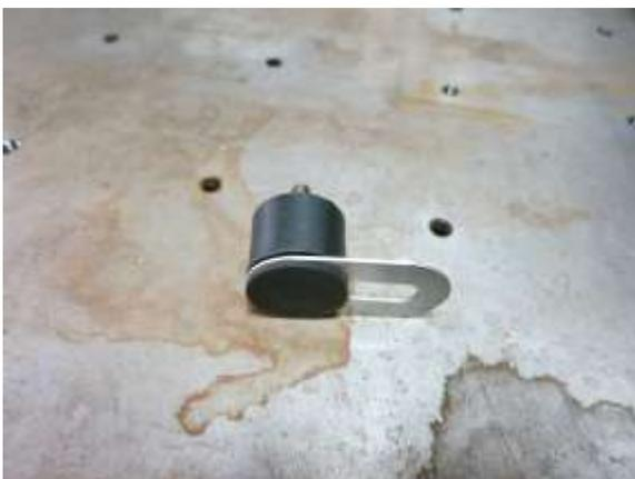
C. On 2014 up models assemble the supplied adapter bracket, rubber mount and rubber insulator pad as shown. **2014 up models require the use of this adapter due to location change of the threaded hole.**
