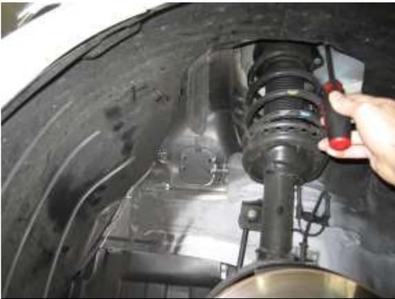
I. Reposition the plastic fender liner and brush guard under the bumper, and then re-install the 5 plastic clips you removed earlier. You can simply push them into each hole to lock in place.
