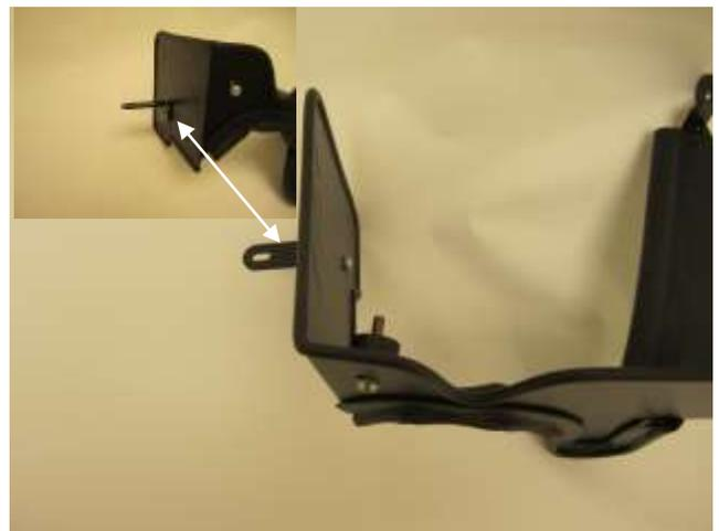
b) Install the bracket (32-3094) onto the backside of the heat shield and secure with provided hardware (1-112 & 1-3018 & 444.460.04). Then install the mount onto the side of the heat shield using (1-112 & 1-3018 & 1228596).
