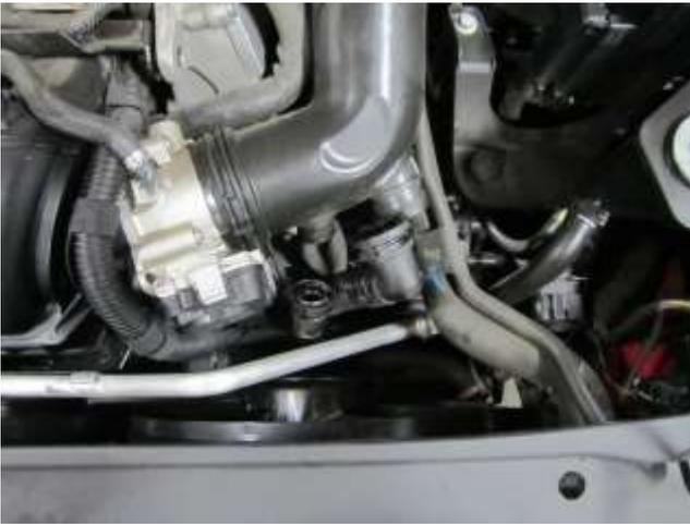
e) Release the pressure on the clamp at the throttle body and remove the stock intake tube. **Note: Do not discard any of your stock intake.**
