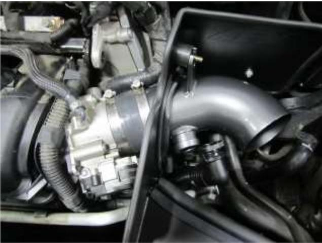
g) Once the lower air injection connectors is properly attached slide the AEM tube into the hose at the throttle body and align the bracket with the mount on the heat shield.
