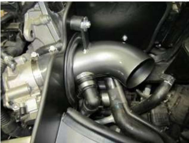
i) Connect the upper (larger) air injection connector onto the AEM tube. **Note: Using warm soap and water on the O-ring (located in the connector) will help ease the connector onto the tube fit-**
