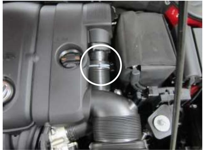
b) Release the pressure clamp at the engine cover outlet as shown and disconnect the stock intake hose from the engine cover.
