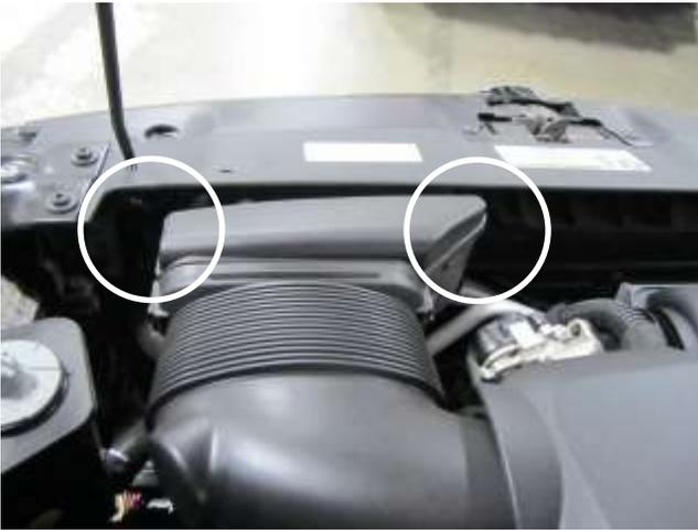
a) With a T-20 Torx, remove the two bolts securing the stock air scoop to the front support. These bolts will be reused.
