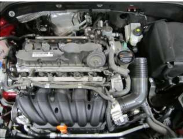
c) Remove the engine cover from the vehicle.
