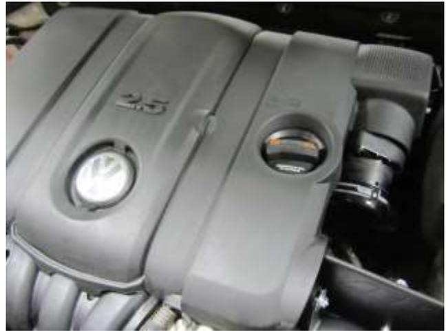
l) Re-install the engine cover onto the engine and push down to secure it.
