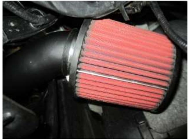
j. Slide the AEM filter onto the tube and tighten the hose clamp (9452). **Note:** Rotate the offset-base filter as necessary to gain best clearance.
