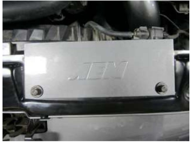
l. Install the heat shield onto the front radiator support using the provided bolts (1-2038)
