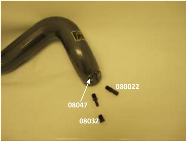
c. Install the correct fitting based on your vehicle vent line configuration. On vehicles equipped with an EVAP vent line use the fitting (08047). On vehicles not equipped, use the plug (08032).
