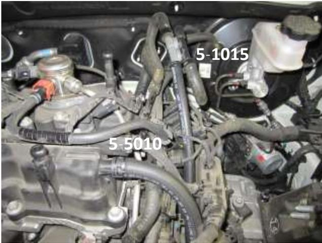
g. Install the other end of hose (5-5010) onto the valve cover port. Install (5-1015) onto the EVAP vent line. Secure with the pressure clamps removed in step 2d.
