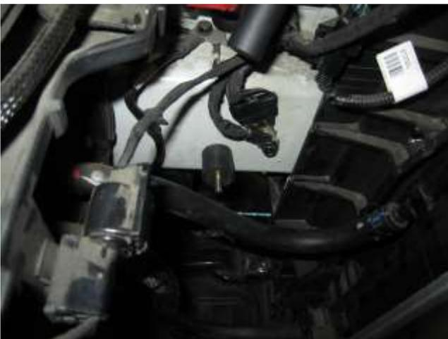
a. Install the rubber mounted stud into the bolt hole that was removed in step 2f. Combine both ground cables together and tighten the bolt back up.
