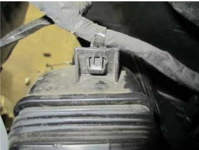
i. Squeeze the clips together while pulling away from the clip retainer. Remove the resonator from the vehicle.
