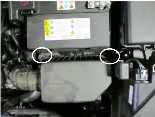
c. Remove the two bolts that secure the stock air box to the vehicle.
