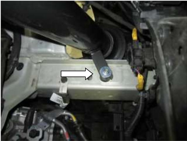
f. After the filter is installed, make sure tube alignment and filter clearance are good before tighten the two hose clamps at the throttle body. Then, tighten the nut securing the bracket to the rubber mount.
