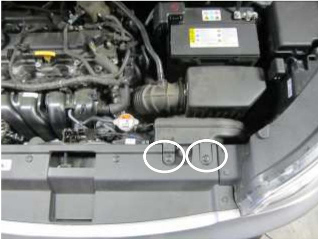
a. Remove the engine cover by pulling it up and out of the vehicle. Remove the two plastic clips (circled) and remove the stock scoop.
