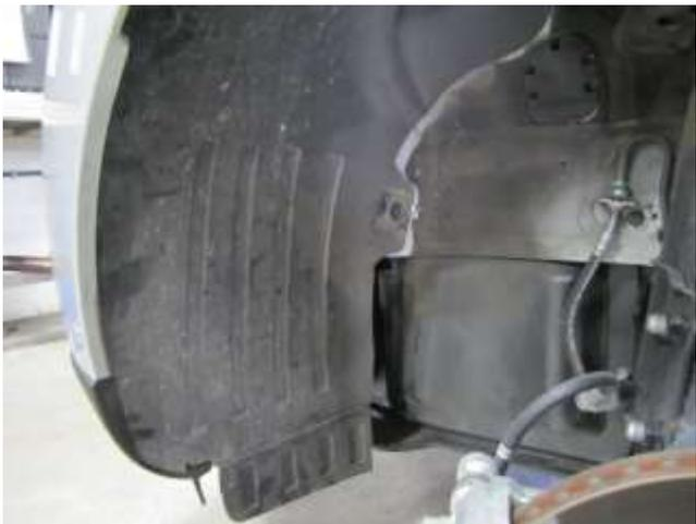
h. Re-install the four plastic clips securing the inner wheel well liner that were remove in step 2f.
