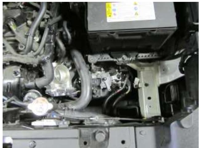
d. Remove the stock air intake system from the vehicle. **Note:** Do not discard any of your stock intake components.
