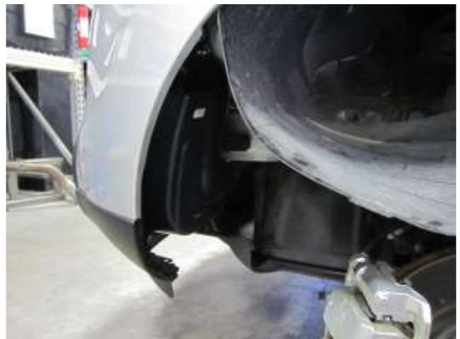
h. Remove the three bolts that secure the resonator to the vehicle. \*See step g for location of the bolts.
