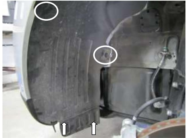
f. Remove the four plastic clips securing the inner wheel well liner. Two of the plastic clips are on the bottom of the liner.
