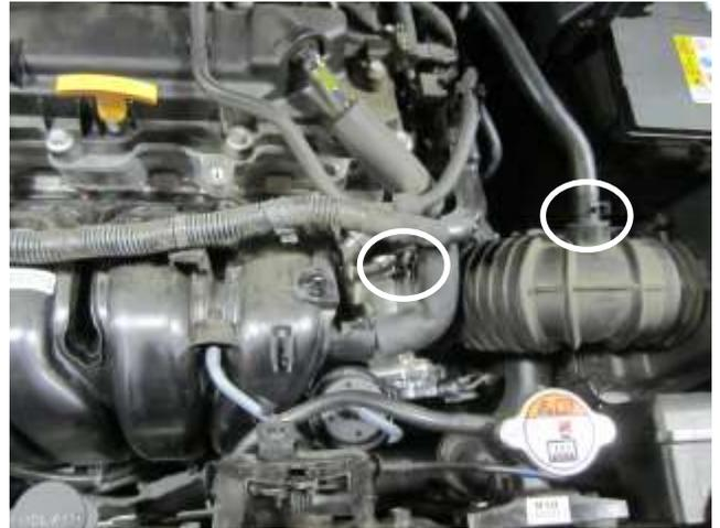
b. Loosen the hose clamp at the throttle body, then release the pressure on the spring clamp and disconnect the valve cover breather hose from the stock intake tube.
