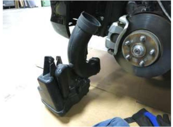
sion, remove the bolt on the right. The resonator can then be pulled out as shown above.
