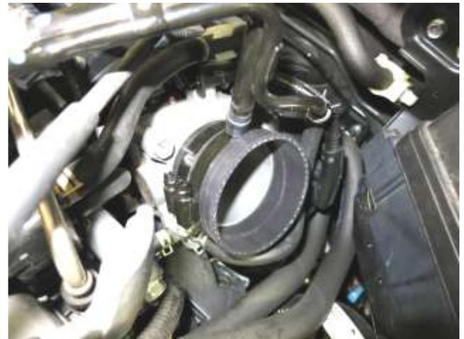
b. Install the included coupler and black hose clamps as shown on the throttle body.
