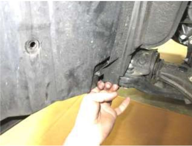
g. Separate the undercarriage panel from the fender liner by rotating them away from each other.
