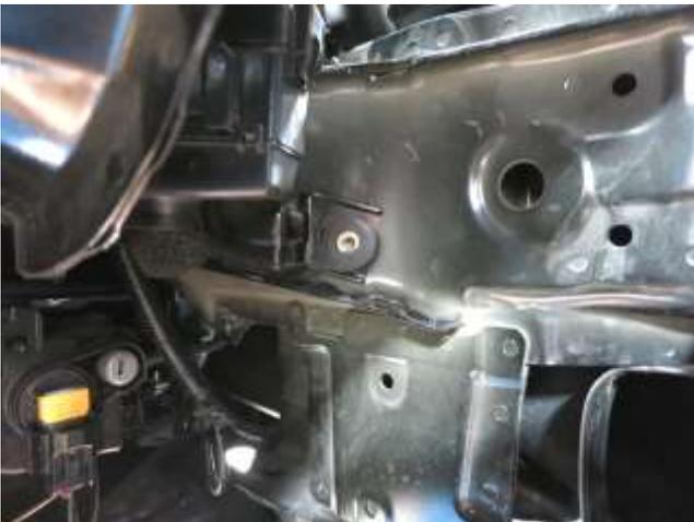
a. Remove the bolt securing the above bracket and replace it with the included rubber mount. Loosely reinstall the bolt with the included washer.
