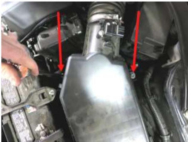
c. Remove the two bolts securing the factory airbox.
