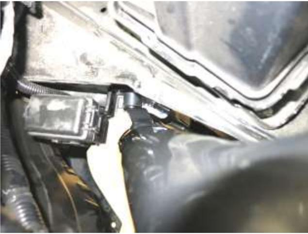
d. Lower the tube down into the engine bay. Insert the tube bracket between the rubber mount & the washer. Slide other end into the coupler & tighten the clamps.
