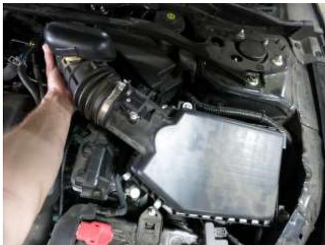
d. Pull the factory intake duct off the throttle body and lift it out along with the airbox.
