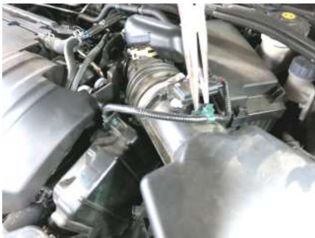
a. Release the green clips retaining the MAF sensor wiring harness and disconnect it from the sensor.
