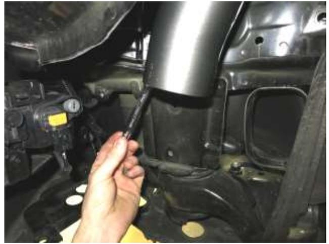
e. Tighten the bolt at the bracket end of the tube with an end wrench.
