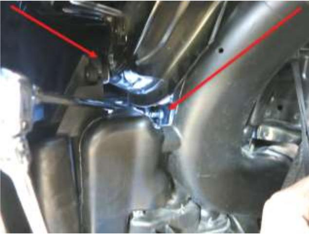
i. First remove the bolt shown above on the left, allowing you to lower the resonator. Using a short 10mm socket and u-joint on the end of at least 14" of exten-
