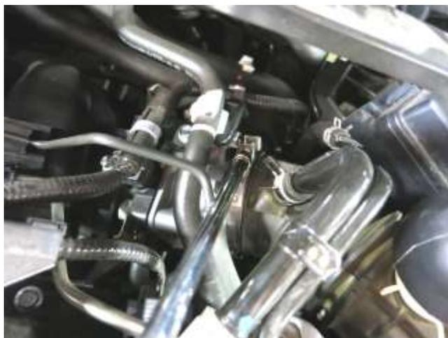
b. Use a cross screw driver or 5.5mm socket to loosen the hose clamp securing the factory intake system to the throttle body. Also remove PCV line from intake boot.
