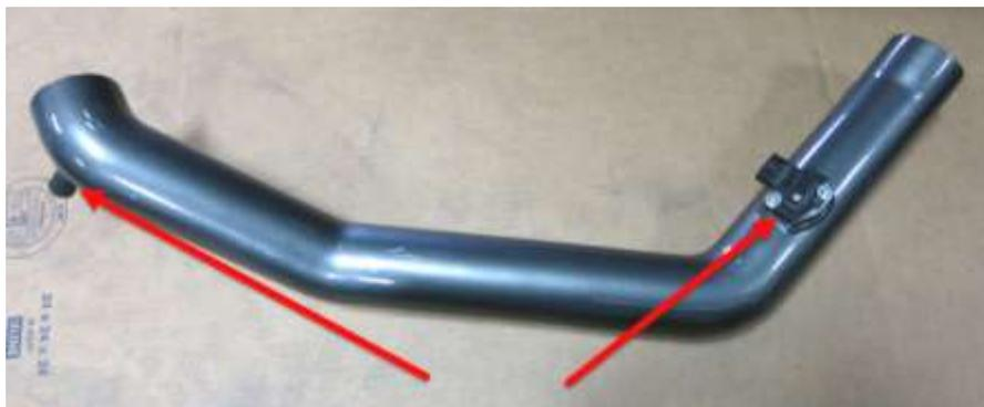
c. Remove the MAF sensor from the factory intake system and install it in your new AEM intake tube with the factory hardware. Also install the rubber tube adapter in the hole at the opposite end of the tube.
