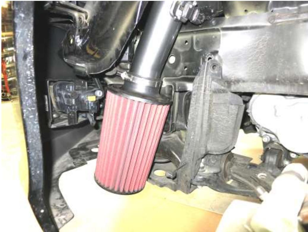
f. Connect the MAF sensor and install the air filter. Install the PCV tube into the adapter at the other end of the tube and seat fully. Reinstall the fender liner and check for clearance at the end of the filter and around the upper edge. If the filter displaces the fender liner, loosen the clamps and bolt, adjust and re-tighten. Reinstall the wheel, taking care to properly torque the wheel to factory specifications.
