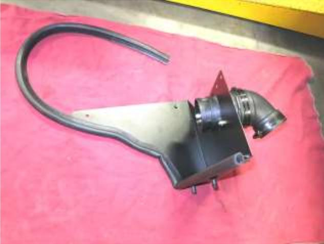
a. Assemble the lower heat shield components as shown according to the graphic on page 2 of this document leaving the edge trim loose at the upper left corner.
