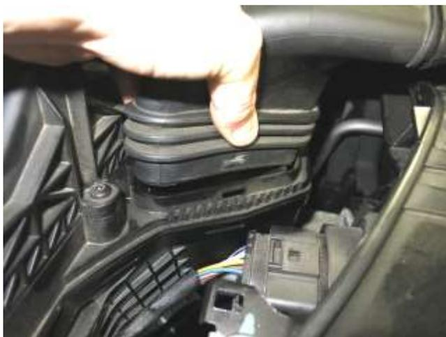
c. Squeeze the lower-most end of the dirty air duct assembly to release and remove it from the factory airbox.
