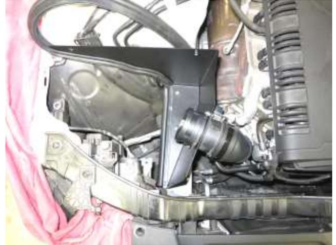
b. Lower the assembly into the vehicle being careful to orient the hose clamps such that they can be accessed by tools to be tightened.
