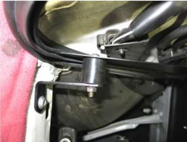
c. Install the included bracket and soft-mount using the factory bolt as shown.
