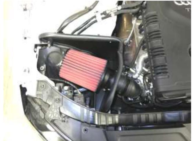
d. Install the air filter. If an open element kit is desired, the edge trim can be installed around the lower heat shield edge as shown above. For better performance via colder air supply, add the upper heat shield/duct and hardware according the graphic on page 2 of this document continuing the edge trim along the edge of the upper heat shield as shown in step f (next page).
