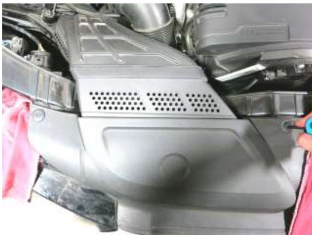
a. Use small pointed tool to depress & release the two left-most pins holding down the radiator top panel.
