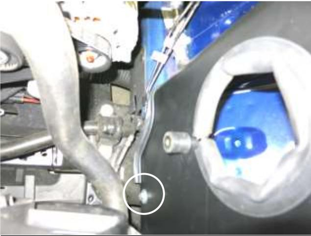
e. Using the provided M8 bolt and washer, tighten the heat shield to the vehicle where shown.
