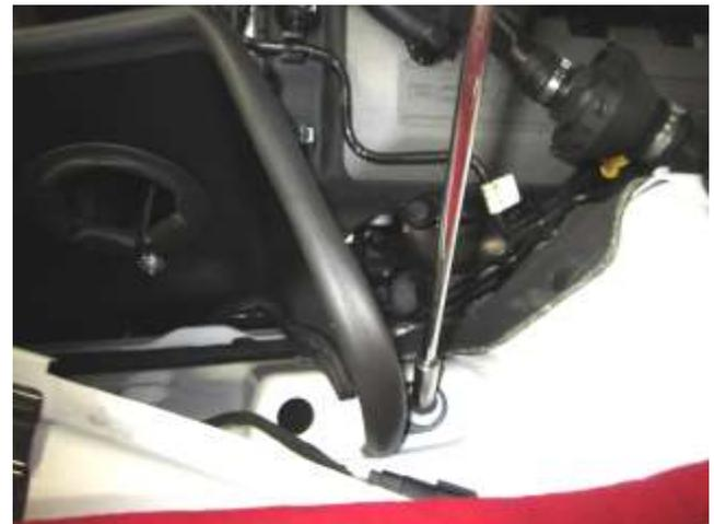
d. Install the completed heat shield into the vehicle. With the bolt removed in step 2b. install the provided washers and tighten the heat shield to the vehicle.
