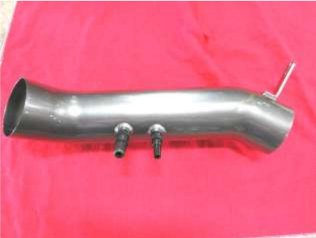
a. Install the two provided vent adapters into the tube as shown. Manual transmissions will use the plug provided instead of the vent adapter on the right side. Install finger tight, then a 1/4 turn with a wrench.
