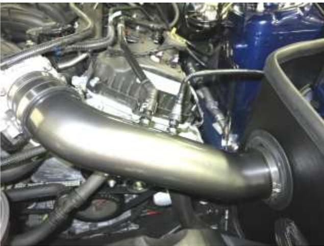
g. Slide the 2 vent lines onto the adapters, making sure you hear a click to confirm they are attached. Manual transmissions will only connect 1 vent line.
