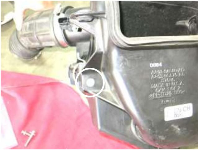
f. Remove the bolt that secures the air scoop to the lower air box. The bolt will not be reused.
