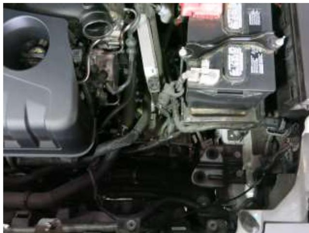
d. Remove the complete air intake assembly from the vehicle. NOTE: DO NOT DISCARD ANY OF YOUR STOCK EQUIPEMNT.
