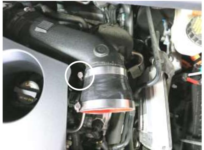
h. Slide the hose onto the turbo inlet pipe with the hose clamps and tighten the one closest to the pipe.
