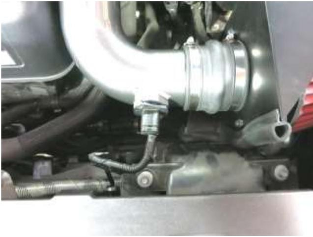
l. Plug the sensor connector back into the sensor and slide the red locking tab in that was removed in step 2a.
