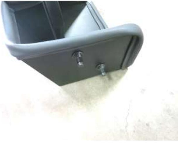
e. Install the plastic mounts with the provided hardware as shown.
