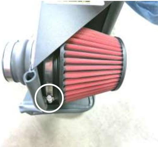
g. Insert the AEM air filter onto the filter adapter and secure with the hose clamp at this time.
