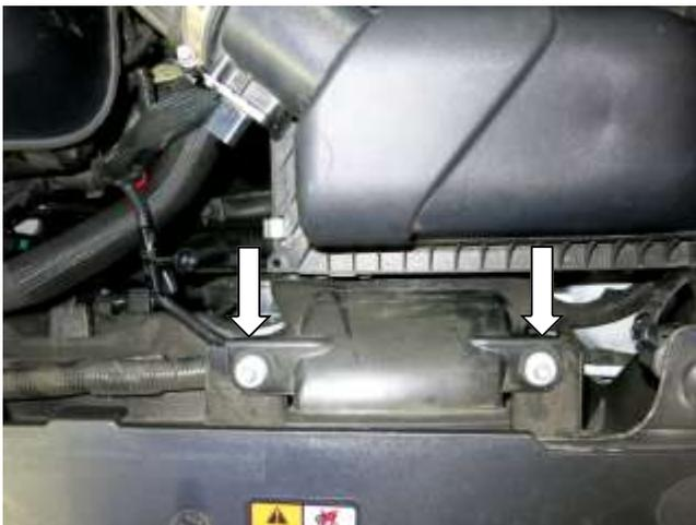
c. Remove the two bolts securing the air scoop to the vehicle. The scoop will be reinstalled in step 3a.
