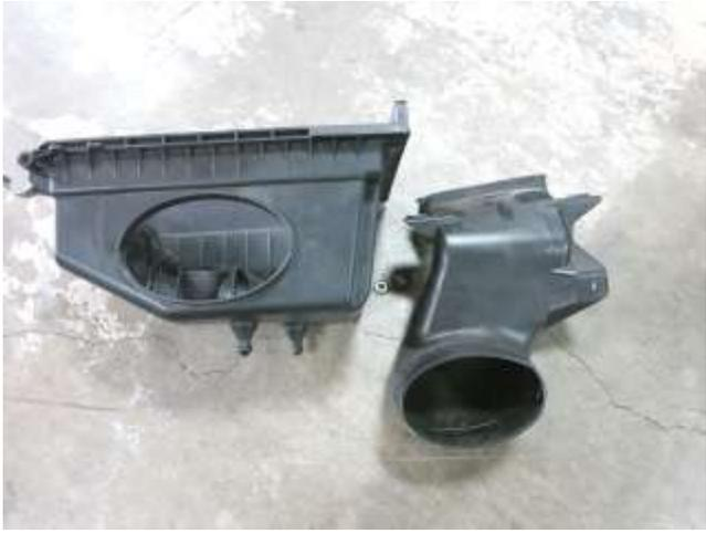
h. Separate the lower air box from the air scoop.
