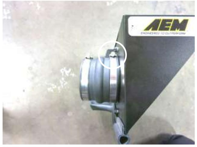
f. Install the provided coupler onto the heat shield air filter adapter. Tighten the hose clamp closest to the heat shield at this time.
