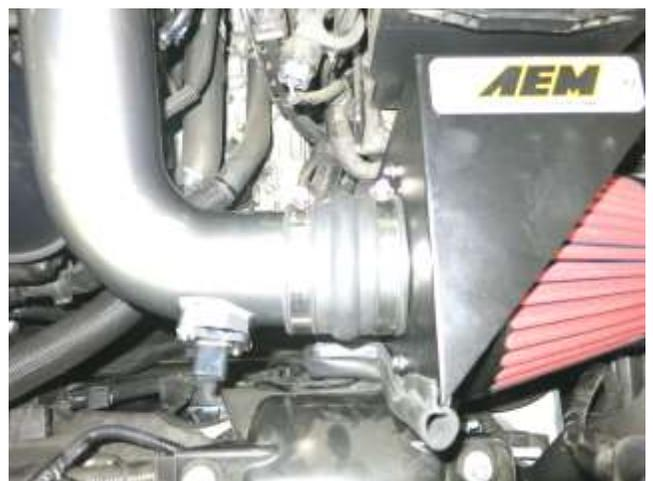
j. Slide the AEM intake tube into the coupler. Do not tighten the hose clamp at this time.
