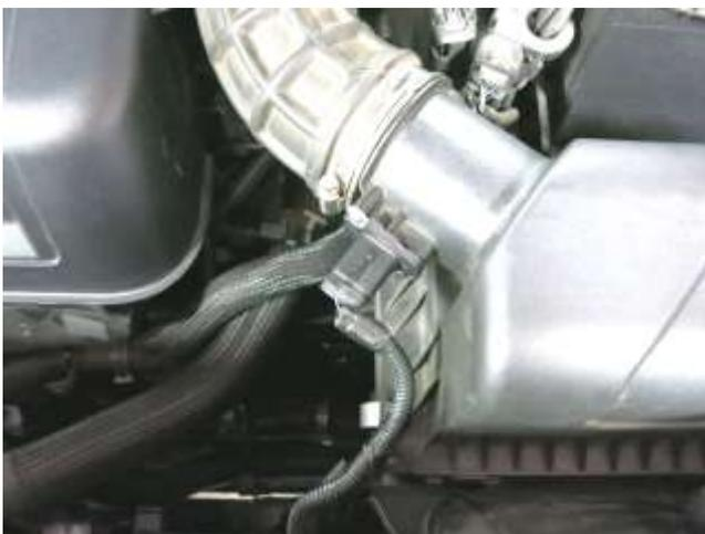
a. Slide the red locking tab and detach the electrical connector from the sensor.
