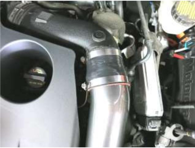
k. Slide the other end into the previously installed coupler on the inlet tube. Secure both hose clamps now once proper tube alignment has been achieved.
