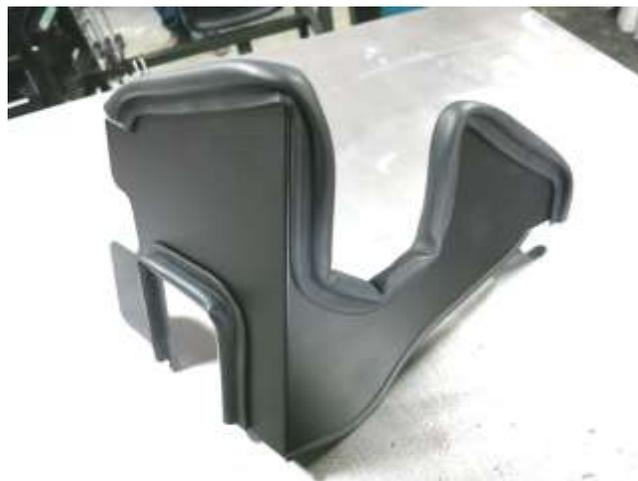
d. Install the 3 provided edge trim pieces onto the AEM heat shield as shown.
