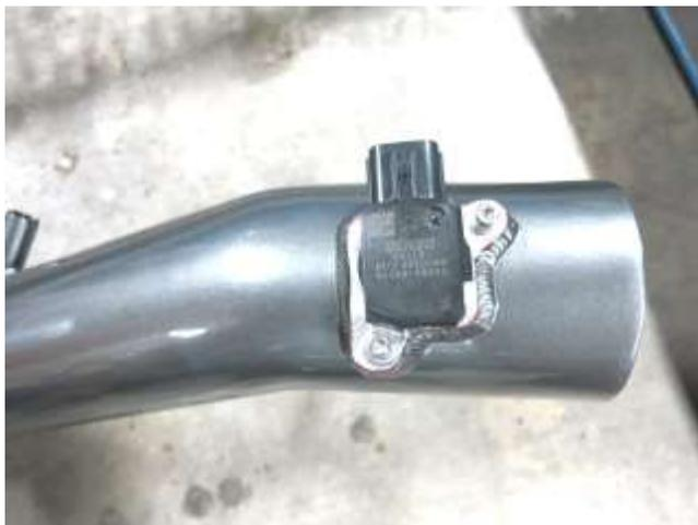
a. Reinstall the MAF sensor into the AEM tube and fasten using the provided bolts(07733).
