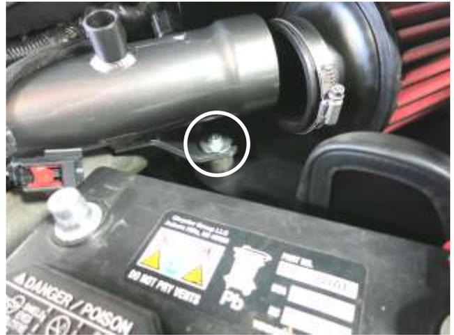
l. Install the provided hardware and secure the AEM intake tube to the rubber mount.
