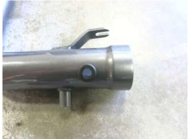
b. Install the provided grommet into the hole on the AEM intake tube.
