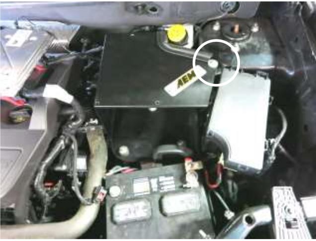
g. Install the assembled heat shield into the vehicle aligning the mounts in the heat shield with the grommets in the vehicle. Align the heat shield with the rubber mount circled and tighten with supplied hardware.
