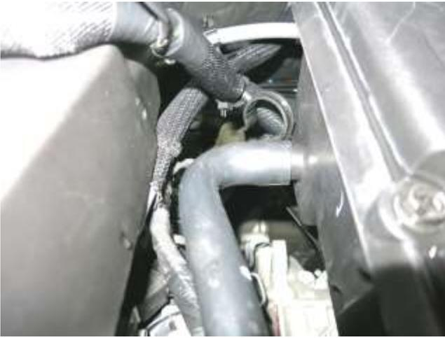
e. Remove the vent hose on the side of the stock air box. This will be reattached in step 30.
