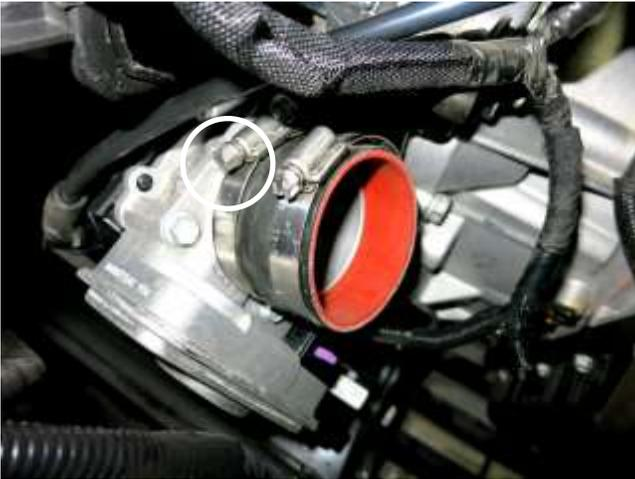
a. Install the provided hose and hose clamps onto the throttle body. Tighten the hose clamp closest to the throttle body at this time.
