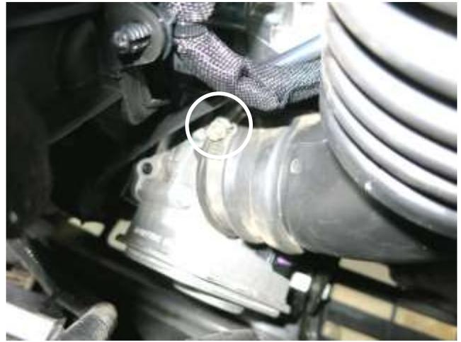
h. Loosen the hose clamp securing the stock intake tube to the throttle body and then remove the intake tube from the vehicle.
