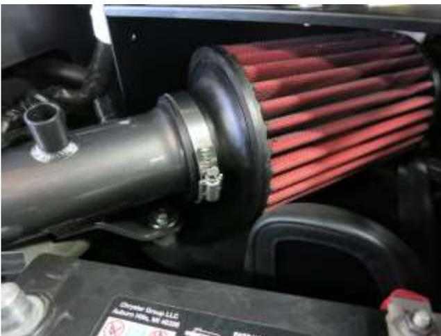
m. Install the AEM air filter onto the AEM tube and tighten the hose clamp.
