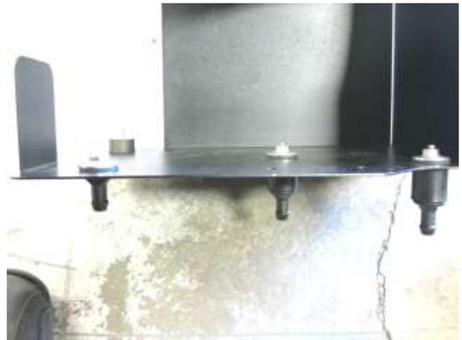
d. Install the provided hardware onto the AEM heat shield. Refer to the exploded view for hardware orientation.
