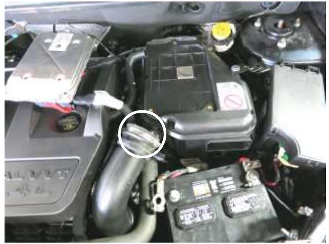
f. Disconnect the stock intake tube from the stock air box.
