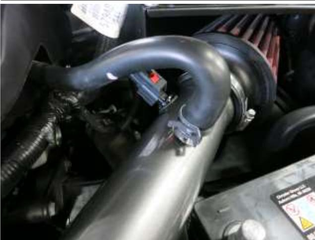
o. Install the vent tube that was removed in step 2e. onto the AEM intake tube with the provided spring clamp.
