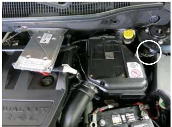
d. Carefully lay the ECU over the engine cover and remove the bolt securing the air box mounting bracket to the inner fender.
