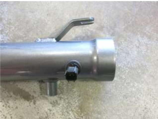
c. Install the air temperature sensor that was removed in step 2i. into the grommet.
