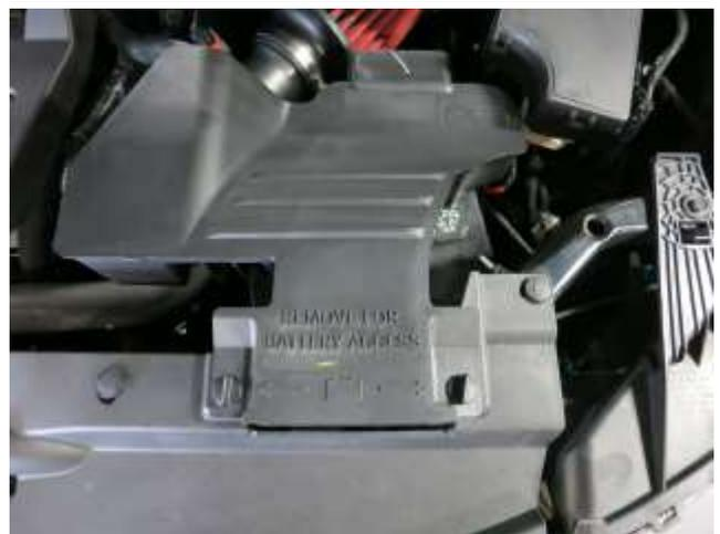
p. Install the fresh air scoop back onto the vehicle that was removed in step 2a.
