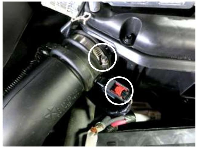
b. Slide the red locking tab and disconnect the intake air temperature (IAT) sensor from the stock intake. Loosen the hose clamp circled.
