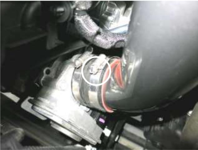
k. With the AEM intake tube aligned in the hose, tighten the hose clamp circled.
