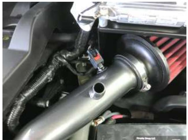
n. Plug the air temperature sensor connector into the air temperature sensor and lock the red locking tab.
