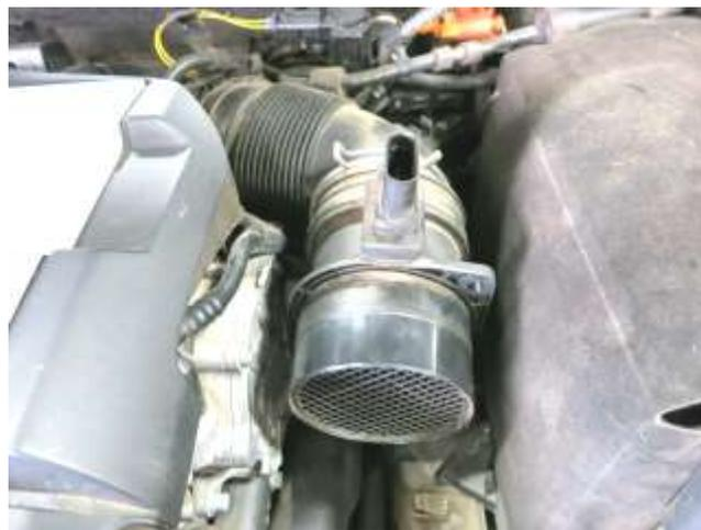
d. Install the MAF sensor into the factory turbo inlet hose. **Note: Pay attention to the air flow direction, the screen side of MAF sensor should face the front of the vehicle.**
