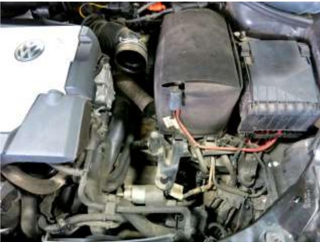
g. Pull up on the air box to disengage it from the tray and remove it from the vehicle. **Note: The smaller hose connected to the lower air box is a water drain.**
