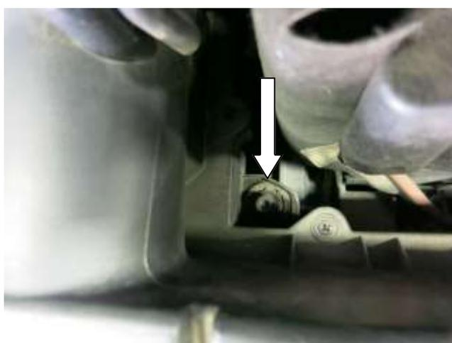
d. Remove the bolt that secures the air box to the air box tray.
