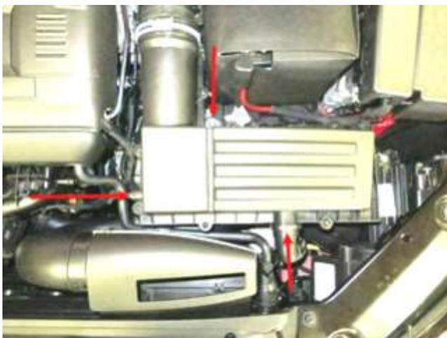
a. Prepare the airbox to be removed by fully loosening the bolt next to the battery, pulling off the hose on the left and disengaging the retained hose on the front and the airbox inlet duct.
