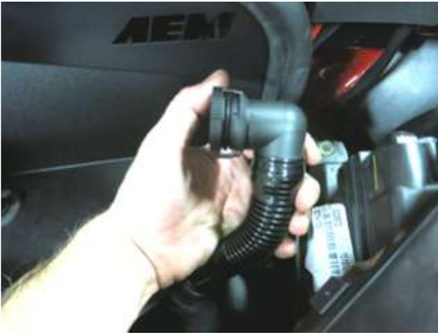
e. Route the retained hose from the airbox to the end of the filter and rotate the fitting in the end of the hose to align it with the end of the filter. Install the adapter into the end of the filter and rotate the filter for best alignment before inserting the hose into the fitting until it clicks to indicate engagement on both sides. Torque all three hose clamps to 30 in-lbs. **If your vehicle does not have air injection system, install the supplied 8-215 cap to the 088012 adaptor.**
