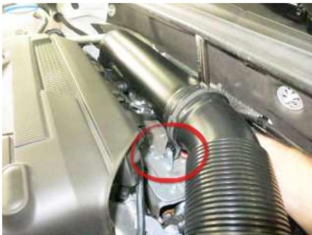
c. Remove the bolt behind the engine securing the factory intake hose to the engine. Lift out the hose and the airbox assembly after pulling the PCV hose near the turbo inlet off.
