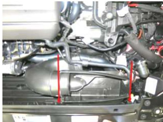
d. Remove the remaining duct components by removing the Torx screws indicated in the photo above.
